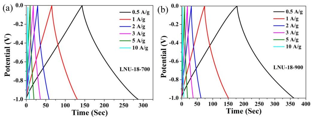
**Fig. S9** GCD curves for (a) LNU-18-700 and (b) LNU-18-900 at different current densities.
