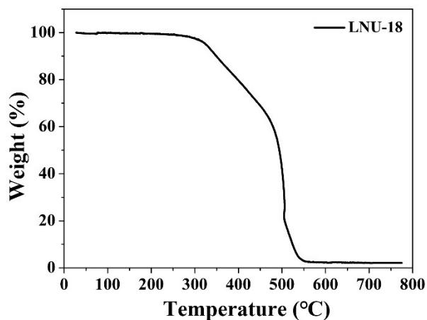
**Fig. S4** TGA curve for LNU-18 in air condition.
