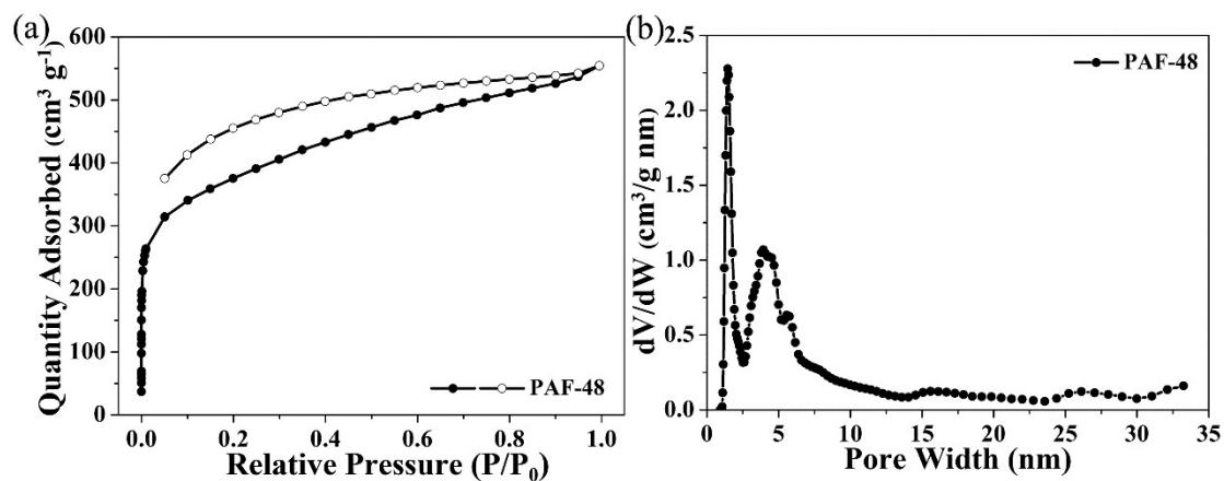
**Fig. S14** (a) Nitrogen adsorption (closed)/desorption (open) isotherms for PAF-48; (b) Pore size distribution curve for PAF-48 calculated by the NLDFT method.
