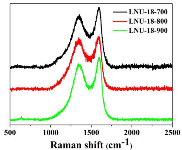
**Fig. S6** Raman spectra for LNU-18-700, LNU-18-800, and LNU-18-900.
