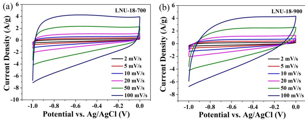
**Fig. S8** CV curves for (a) LNU-18-700 and (b) LNU-18-900 at different scan rates.
