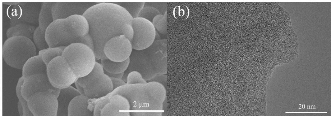
**Fig. S13** (a) SEM and (b) TEM micrograph for PAF-48.
