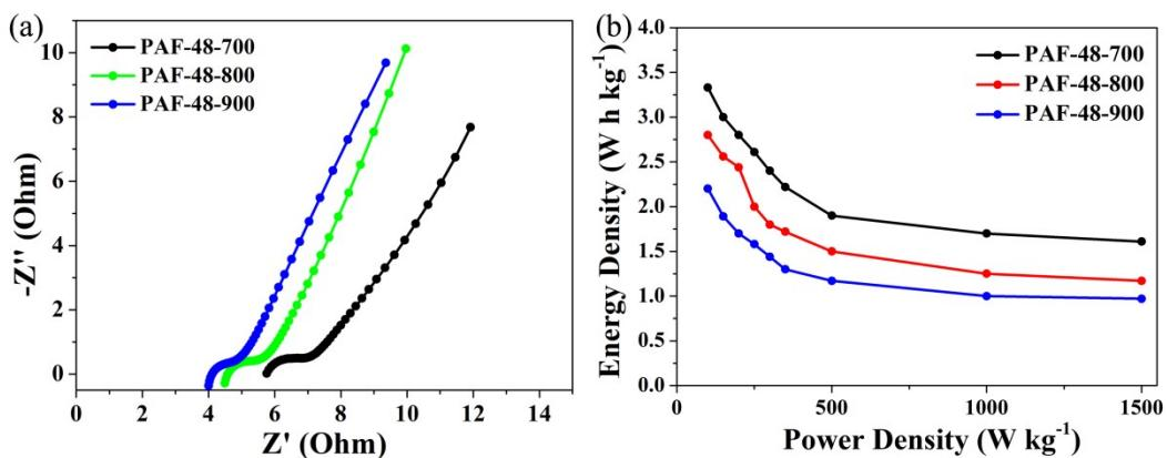
**Fig. S18** (a) Nyquist plots for PAF-48s in the frequency range from 0.01 Hz to 100 kHz in the three-electrode system; (b) Ragone plots for PAF-48s in the two-electrode system.
