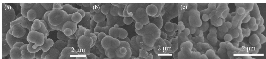
**Fig. S15** SEM micrographs for PAF-48-700 (a), PAF-48-800 (b) and PAF-48-900 (c).
