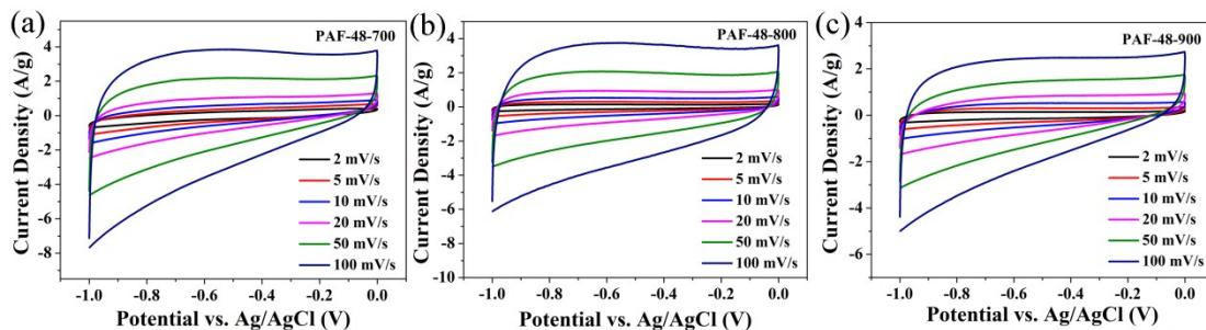
**Fig. S16** CV curves for (a) PAF-48-700, (b) PAF-48-800, and (c) PAF-48-900 at different scan rates.
