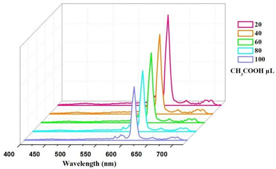
**Fig.S10** Emission spectra of doped complex Eu<sub>0.4</sub>Gd<sub>0.6</sub>DBM upon incremental addition of acetic acid.
