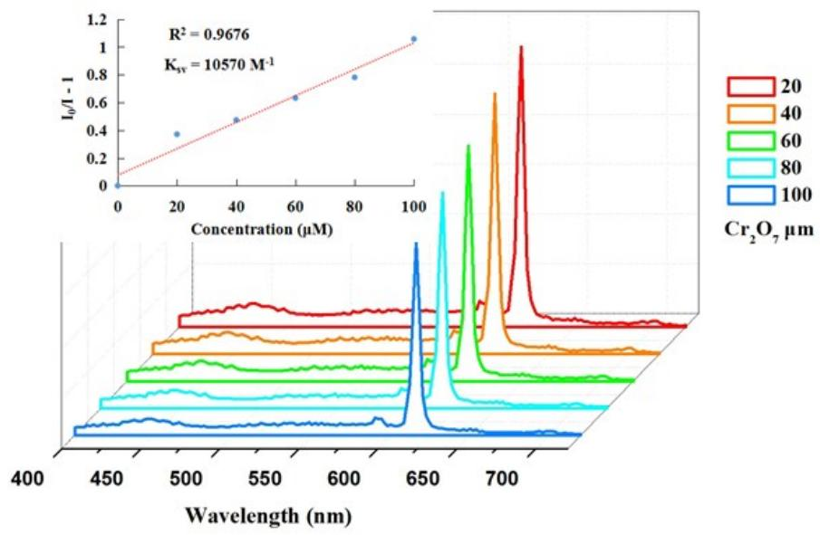
**Fig.S12** Emission spectra of complex  $\text{Eu}_{0.4}\text{Gd}_{0.6}\text{DBM}$  with increasing concentration of  $\text{Cr}_2\text{O}_7^{2-}$ .
