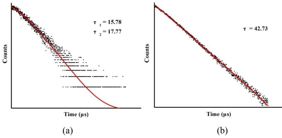
**Fig.S5** (a) Luminescence decay profile for complex **1** in the solid state; (b) Luminescence decay profile for doped complex **Sm<sub>0.4</sub>Gd<sub>0.6</sub>DBM** in the solid state.
