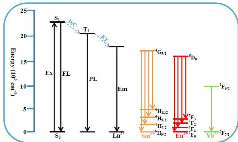
**Fig.S9** Schematic energy level diagram and energy transfer processes.  $S_1$ : first excited singlet state and  $T_1$ : first excited triplet state.
