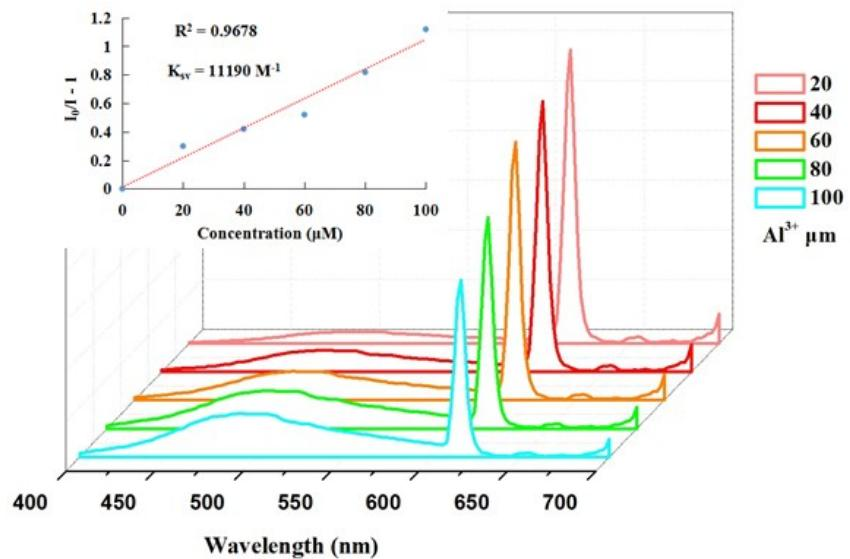
**Fig.S11** Emission spectra of doped complex Eu<sub>0.4</sub>Gd<sub>0.6</sub>DBM with increasing concentration of Al<sup>3+</sup>.
