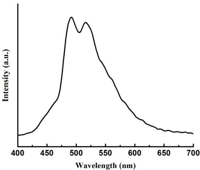
**Fig.S8** Phosphorescence spectrum of  $\text{Gd}_2\text{L}_2(\text{DBM})_4(\text{OAc})_2$  (**3**) at 77K.
