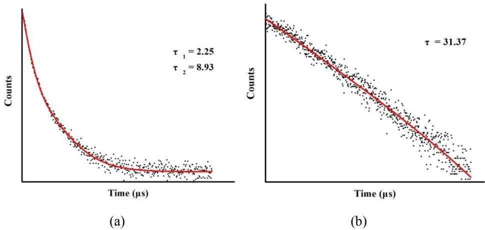
**Fig.S7** (a) Luminescence decay profile for complex **4** in the solid state; (b) Luminescence decay profile for doped complex **Yb<sub>0.1</sub>Gd<sub>0.9</sub>DBM** in the solid state.
