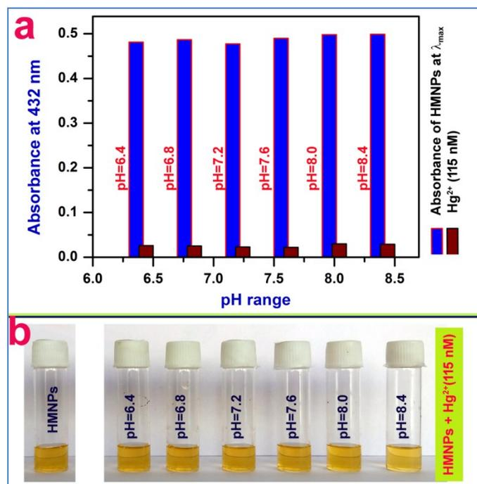
**Fig S6:** (a) Optimization of sensing response for  $Hg^{2+}$  ion in a pH range 6.4 to 8.4 at 432 nm.
