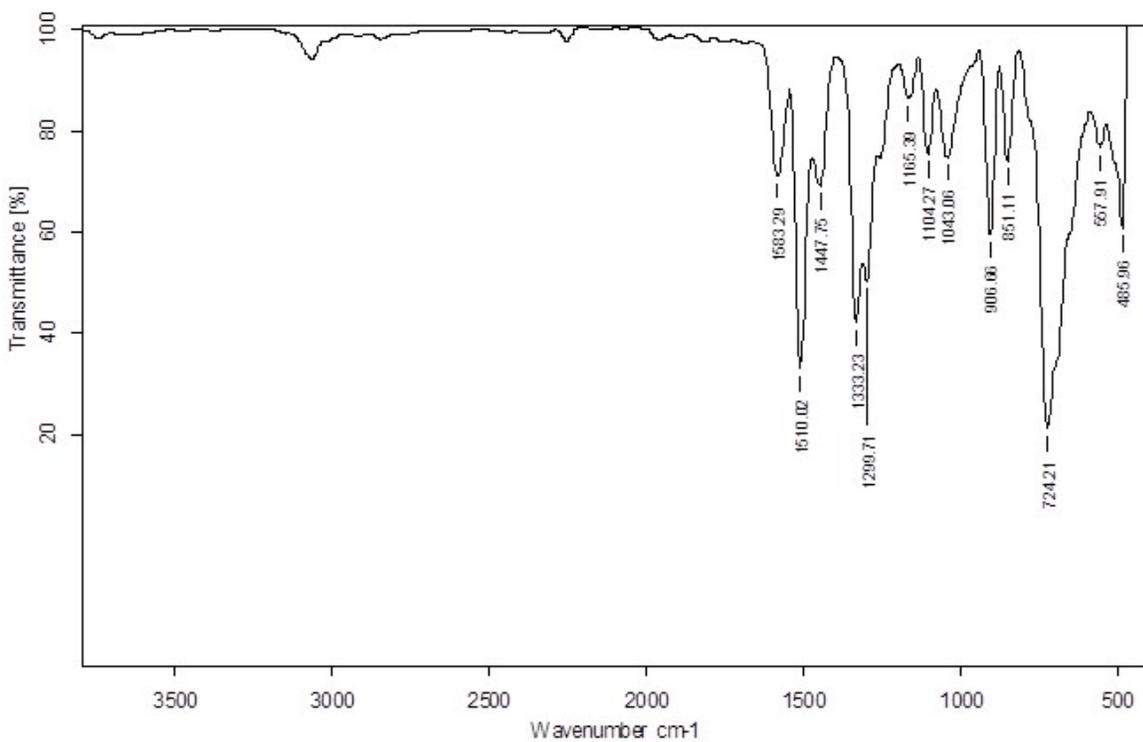
Fig. S32. Neat FT-IR spectrum of compound **2a**
