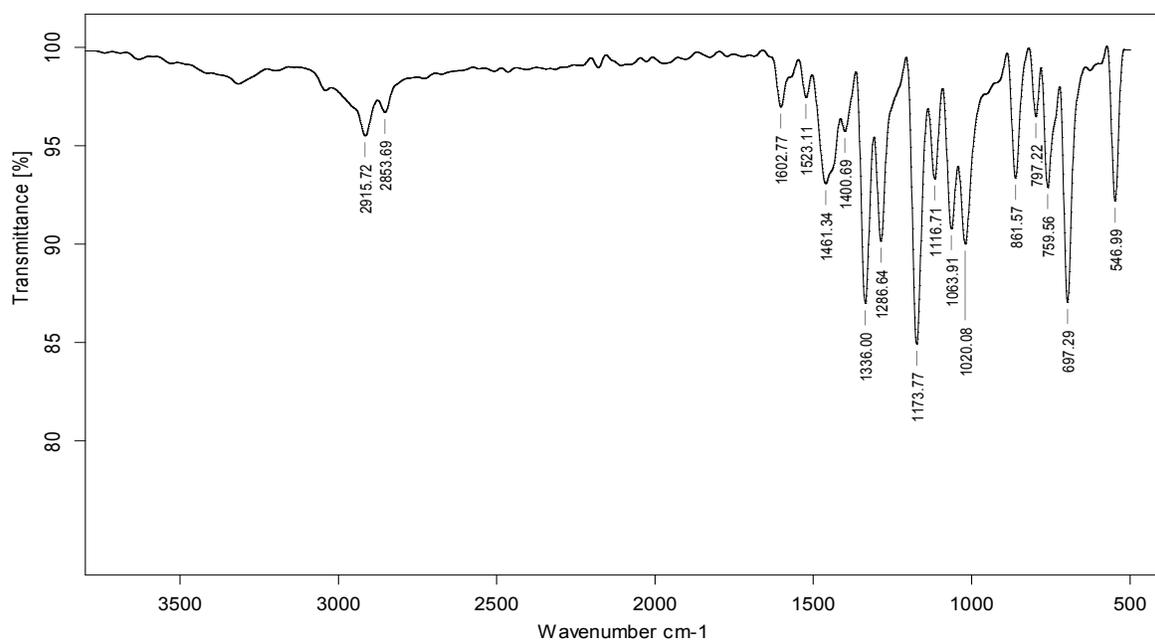
Fig. S6. Neat FT-IR spectrum of  $L^2$
