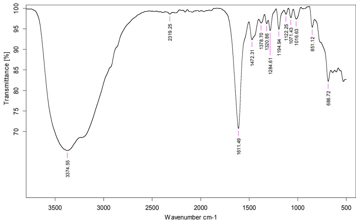
Fig. S16. Neat FT-IR spectrum of complex **2**
