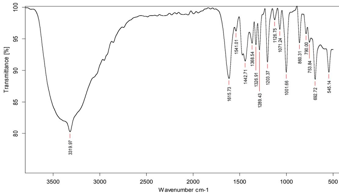
Fig.S19. Neat FT-IR spectrum of complex 3
