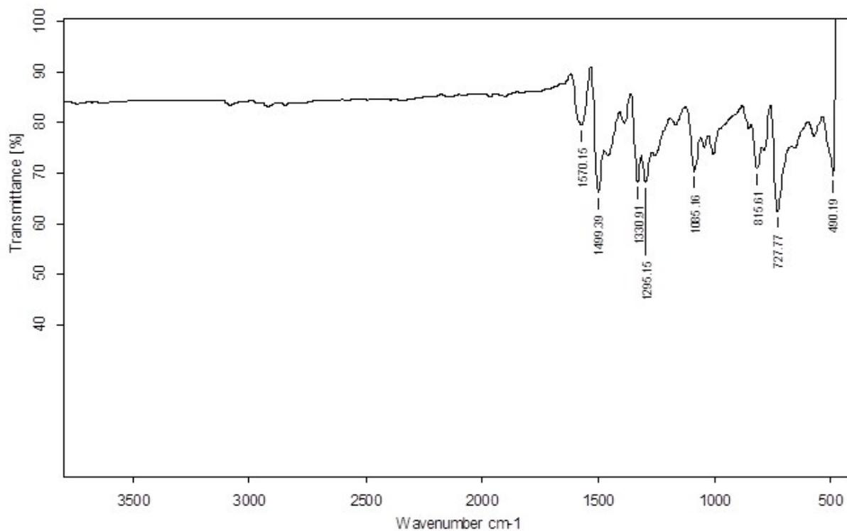
Fig. S44. Neat FT-IR spectrum of compound **6a**
