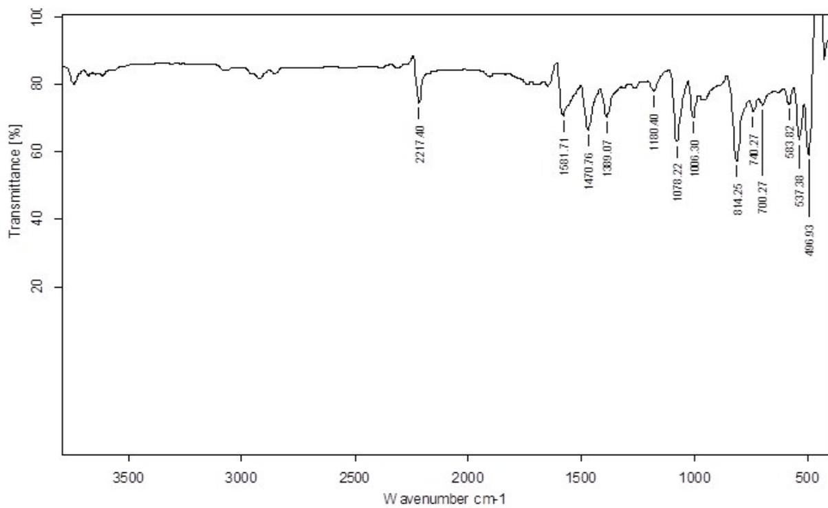
Fig. S35. Neat FT-IR spectrum of compound **3a**
