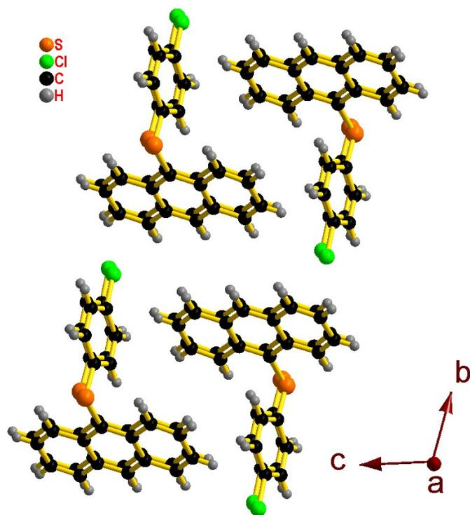
Fig. S72. Molecular packing of **E14**.
