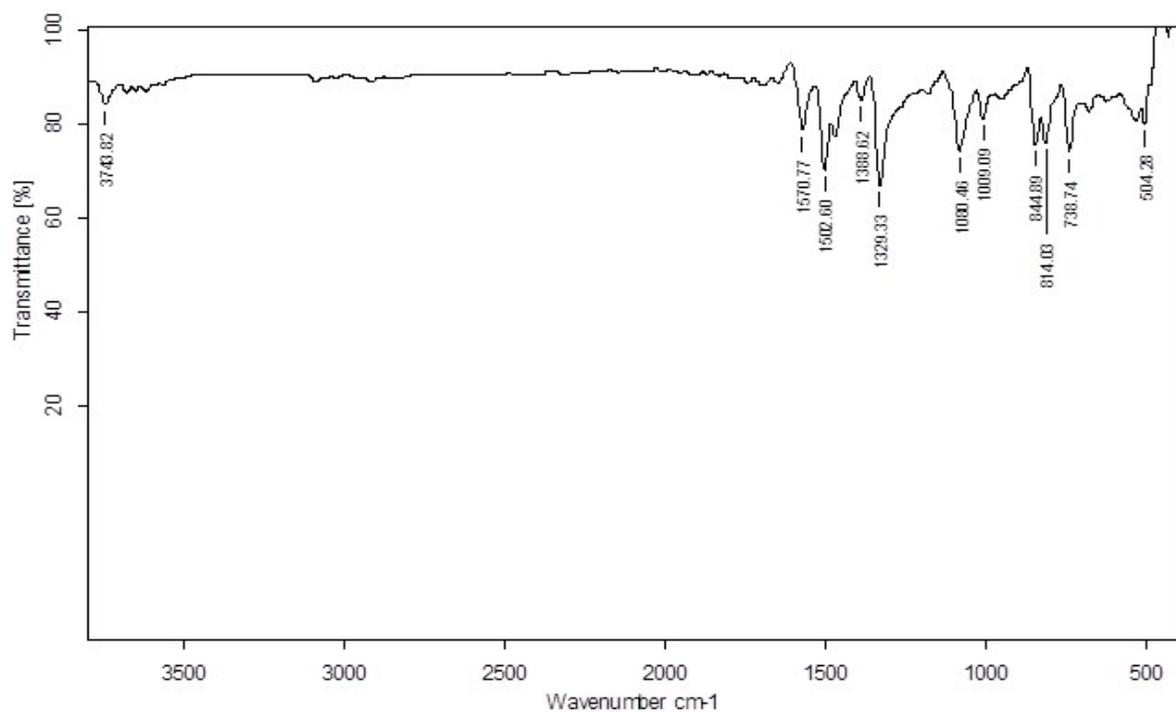
Fig. S62. Neat FT-IR spectrum of compound **12a**
