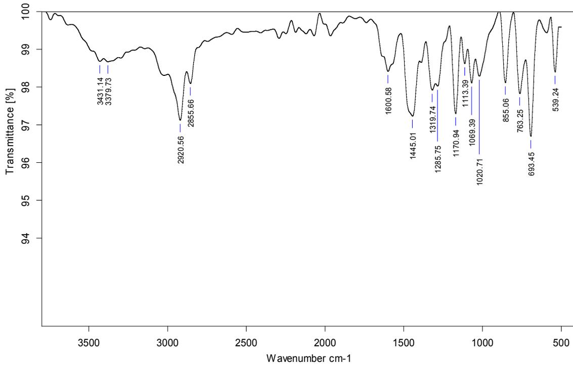
Fig. S3. Neat FT-IR spectrum of  $L^1$
