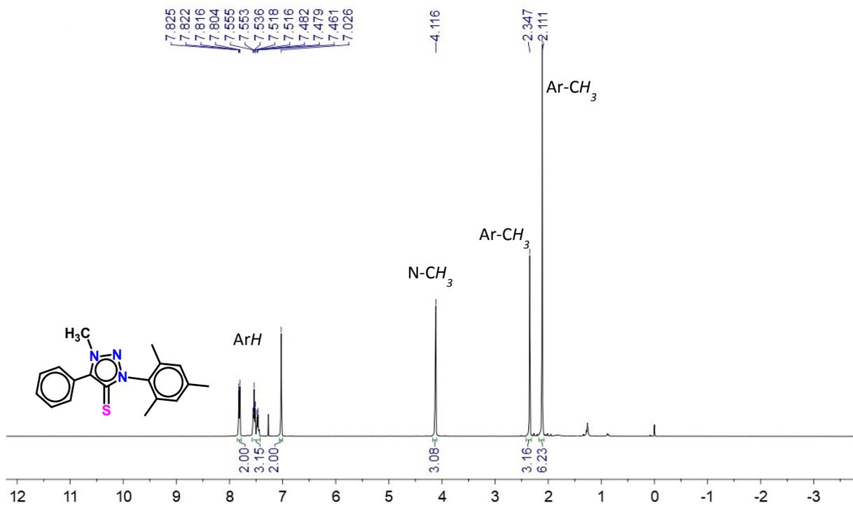
Fig. S4  $^1H$  NMR spectrum of  $L^2$  in  $CDCl_3$
