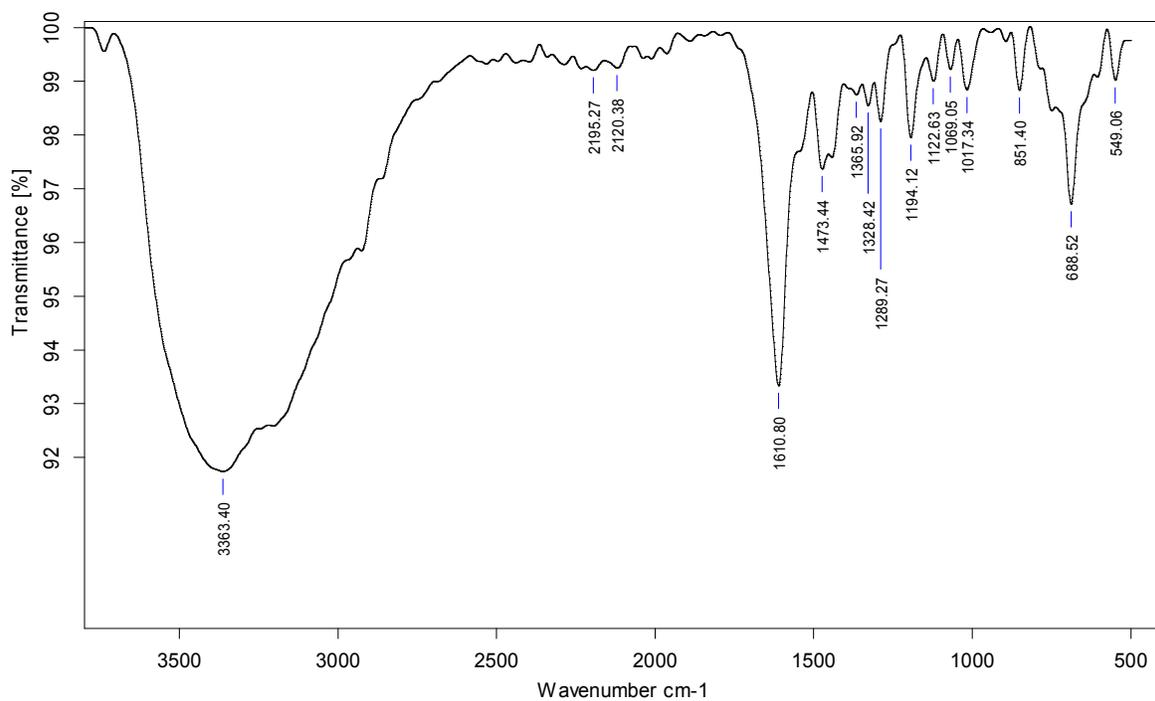
Fig. S22. Neat FT-IR spectrum of complex 4
