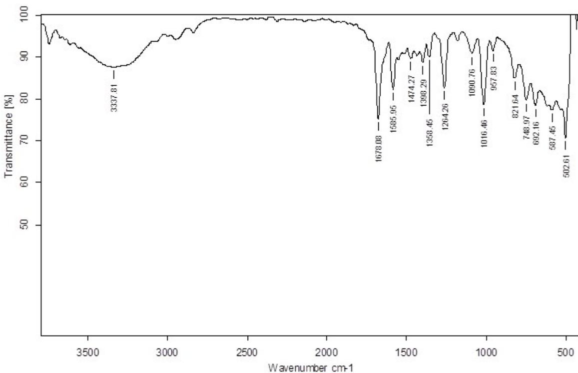
Fig. S38. Neat FT-IR spectrum of complex 4a
