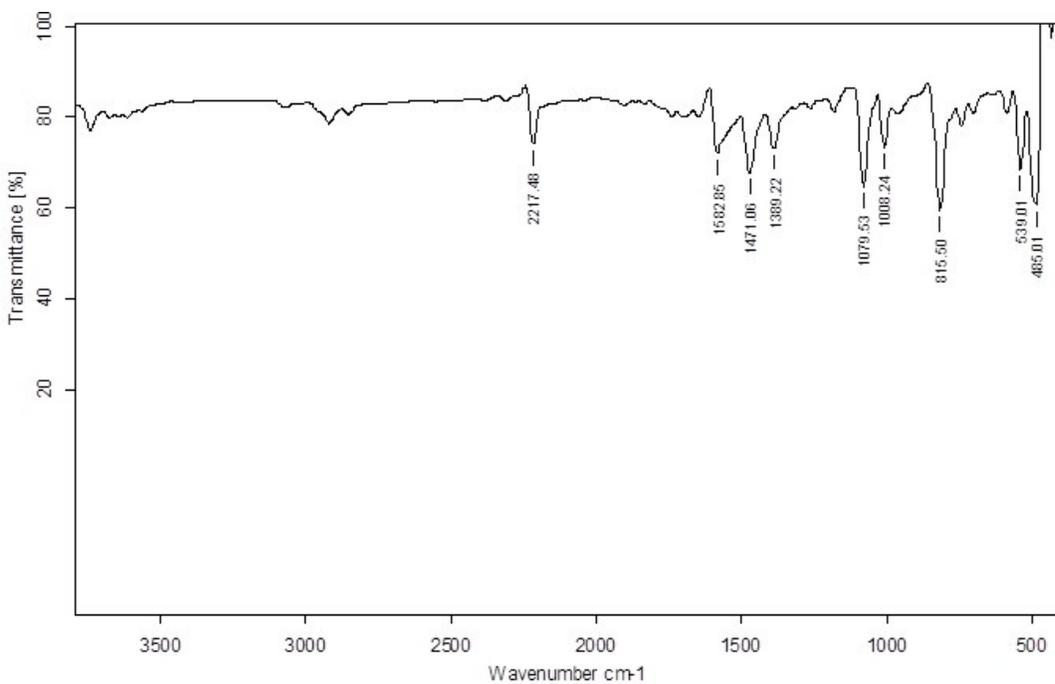
Fig. S47. Neat FT-IR spectrum of compound **7a**
