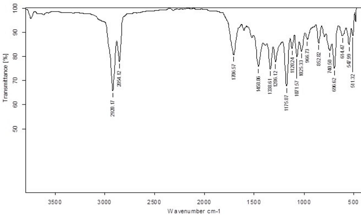
Fig. S59. Neat FT-IR spectrum of complex **11a**
