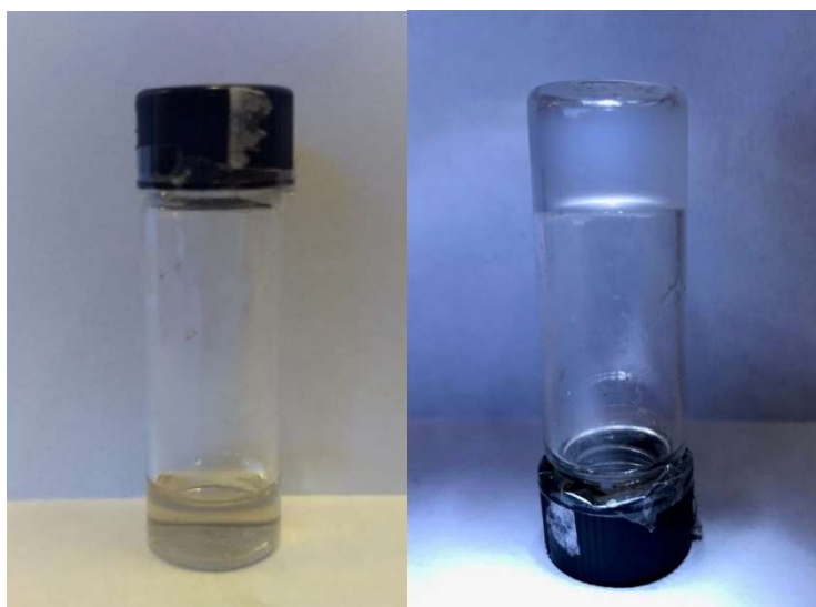
Figure S5. Pictures taken at 25°C of a sol and a gel (inverted flask) of gelator 2,7-THTP-DiC6OH ( 5b ) in ethanol/water 95/5.
