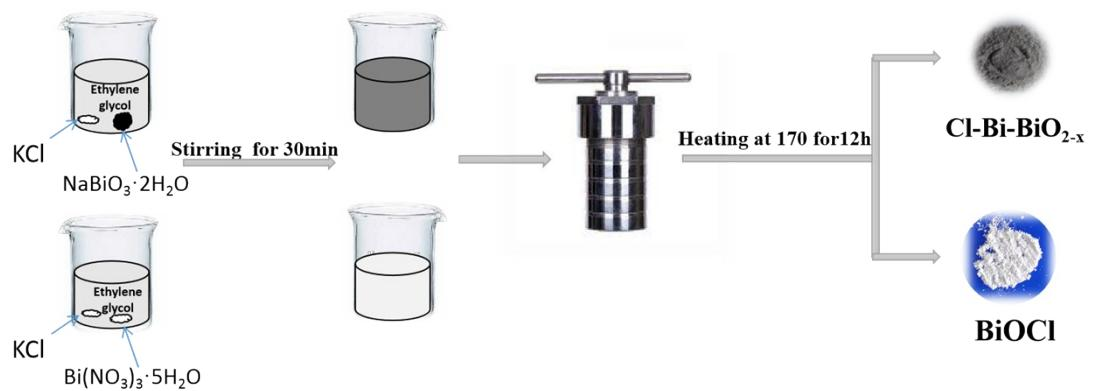
**Scheme S1.** The synthesis flow diagram of  $\text{Cl-Bi-BiO}_{2-x}$  and  $\text{BiOCl}$ .
