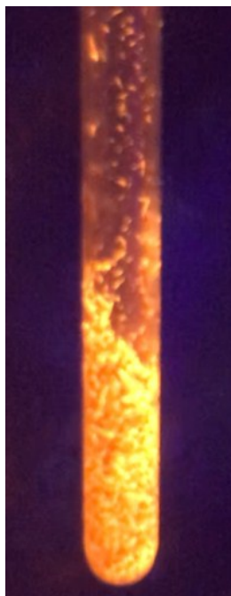
Figure S7. The photograph of the luminescence of 1 taken at 77 K (soaked in liquid nitrogen) excited with a hand-held UV lamp (365 nm).
