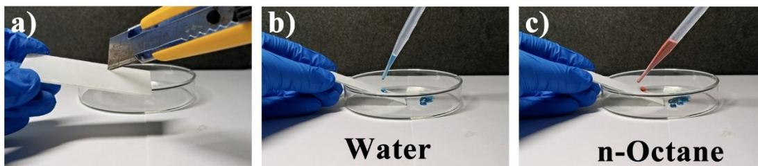
**Fig S1.** a) The scratching test of superamphiphobic coating. b) and c) After scratching test, the liquid repellency with water and n-octane.
