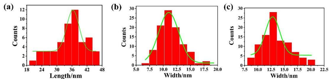
**Fig. S1** Length- (a) and width-distribution histogram (b) for rectangular-shaped 2D CdSe nanocrystals and width-distribution histogram (c) for square-shaped 2D CdSe nanocrystals.
