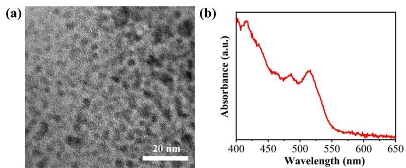
Fig. S5. TEM image (a) of CdSe 2D nanocrystals grown for 20 min at 230 °C at an intermediate concentration of the seeds, and their corresponding absorption spectra (b).
