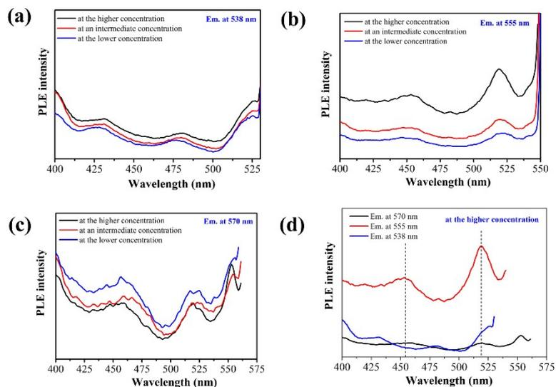
**Fig. S4** The PLE spectra of the CdSe 2D nanocrystals obtained at different concentrations of CdSe seeds measured at PL peak position of 538 nm (a), 555 nm (b) and 570 nm (c) and normalized to its absorbance peak around at 554 nm, respectively. (d) the PLE spectra of the CdSe 2D nanocrystals grown at the higher concentration of CdSe seeds at different emission wavelength.
