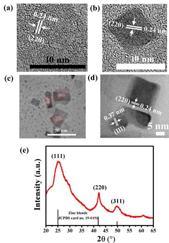
**Fig. S3** (a, b, c and d) HRTEM images of CdSe 2D nanocrystals grown at the lower concentration of the seeds, (e) XRD pattern of the CdSe 2D nanocrystals, the standard zinc blende structure of CdSe (black line, JCPDS card no. 19-0191) inserted as references.
