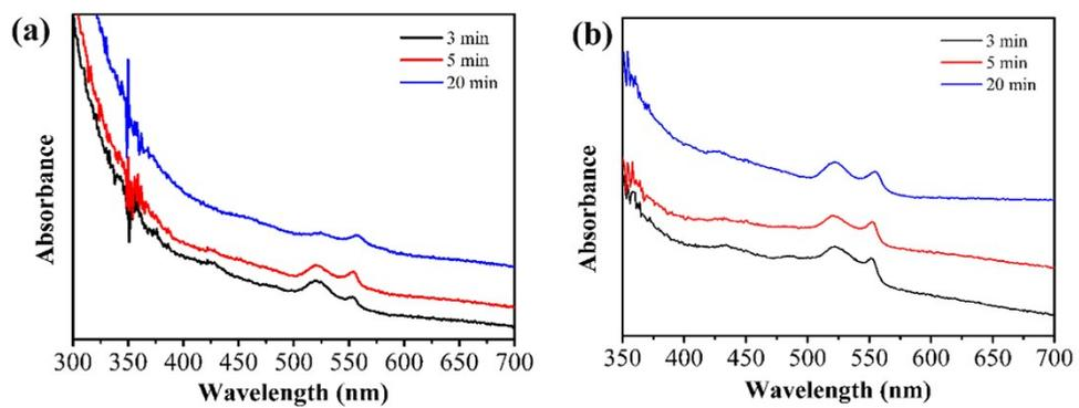
**Fig.S2** The spectra of UV-vis of CdSe 2D nanocrystals at a lower concentration of the seeds (a) and at a higher concentration of the seeds (b).
