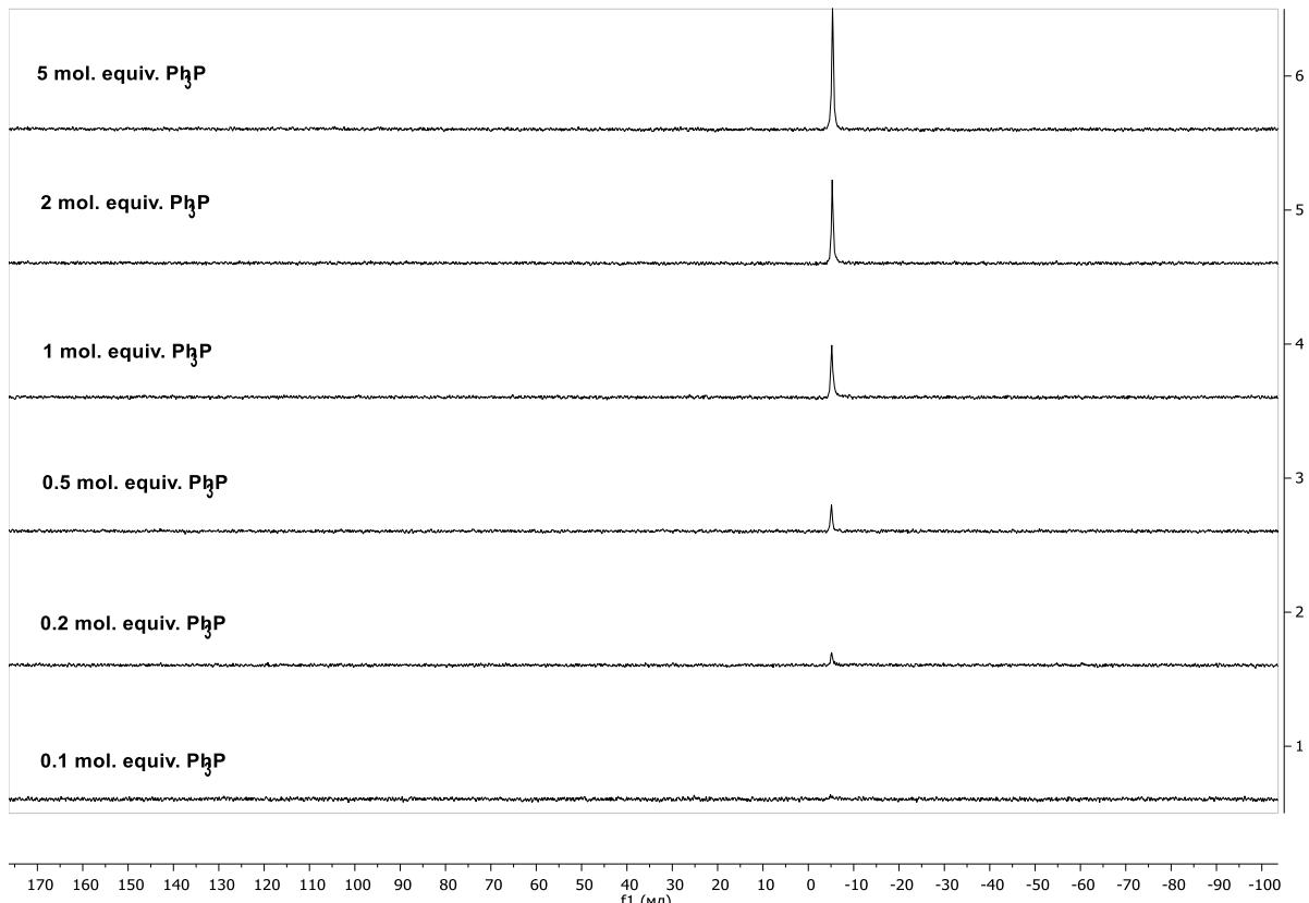
**Figure S7.**  $^{31}\text{P}$  NMR (400 MHz) spectrum of **2** titrated with  $\text{PPh}_3$  in  $\text{CD}_2\text{Cl}_2$ .
