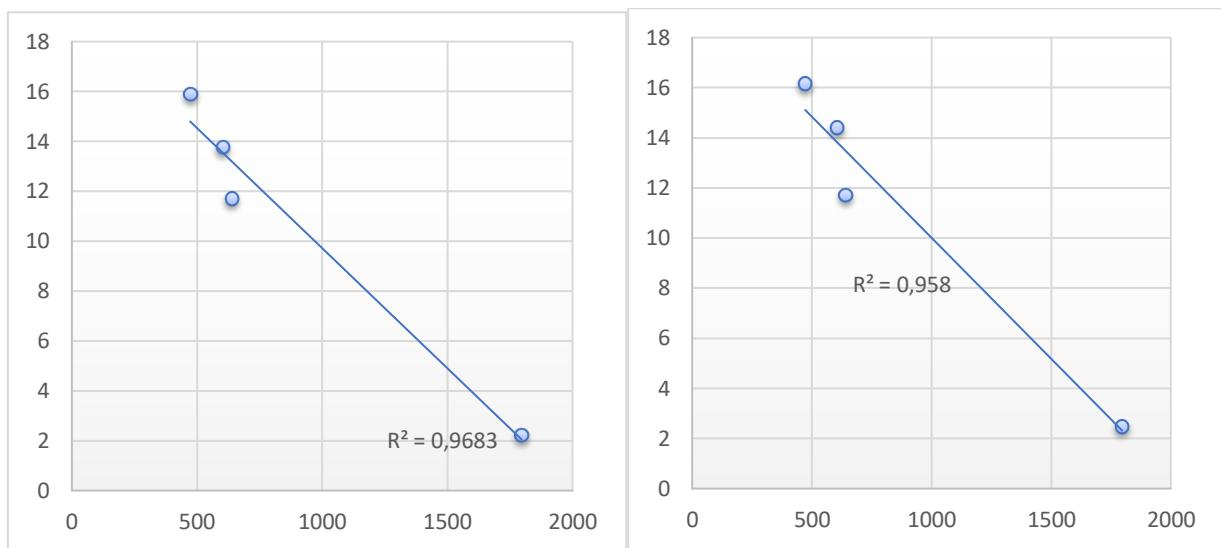
**Figure S8.** Dependencies of 1-butene (A) and  $\alpha$ -olefin (B) shares on activity of **2**/Et<sub>2</sub>AlCl 150 with different amounts of Ph<sub>3</sub>P.
