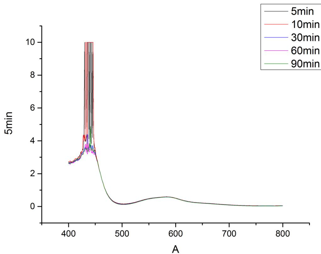
**Figure S13.** UV-Vis spectrum of complex **3** in  $\text{CH}_2\text{Cl}_2$ .
