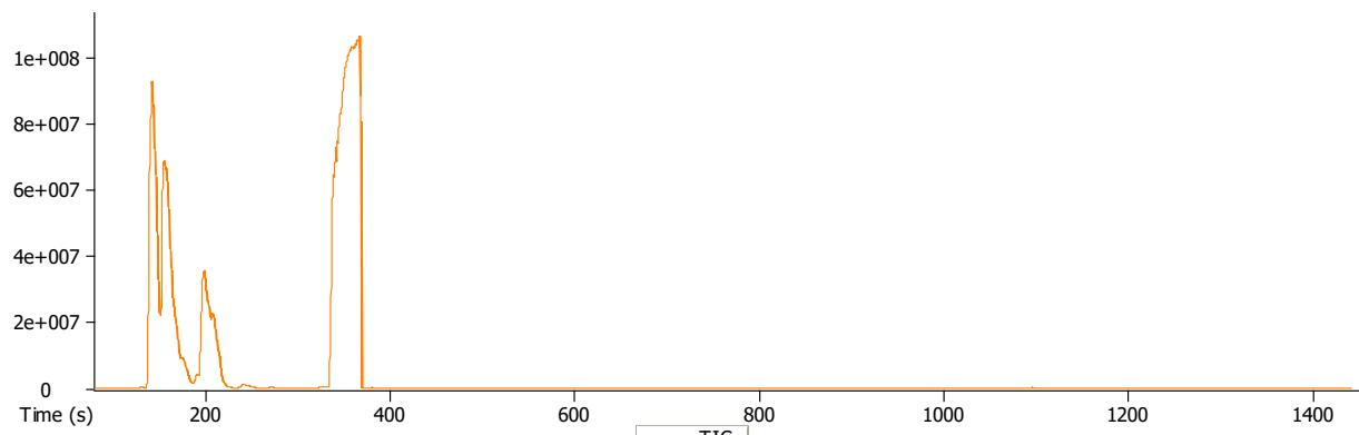
**Figure S16.** GC-MS total ion current chromatogram of run 5, Table 2, system **2/Et<sub>2</sub>AlCl 150/Ph<sub>3</sub>P 1**
