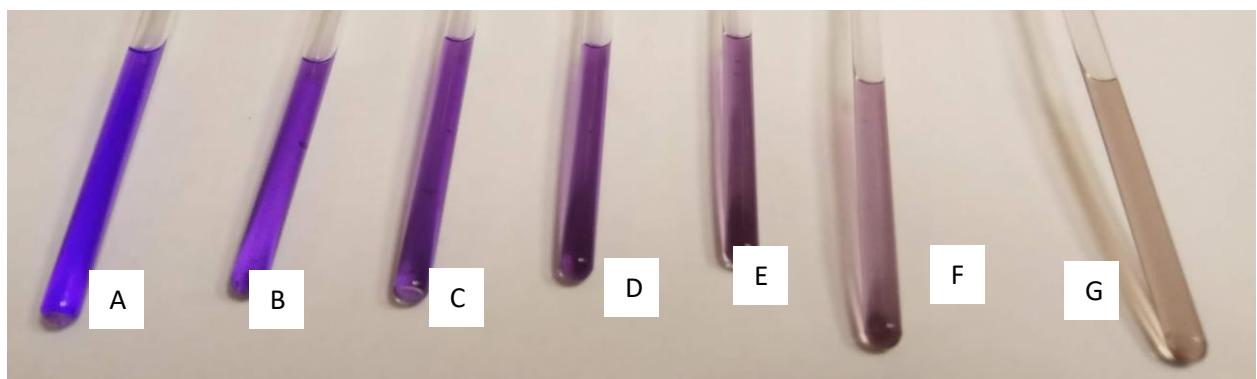
**Figure S9.** Change of complex **2** solution colors in CD<sub>2</sub>Cl<sub>2</sub> with the addition of Ph<sub>3</sub>P: (A) – pure complex, (B) – **2** + 0,1 mol. equiv. of Ph<sub>3</sub>P, (C) – **2** + 0,2 mol. equiv. of Ph<sub>3</sub>P, (D) – **2** + 0,5 mol. equiv. of Ph<sub>3</sub>P, (E) – **2** + 1 mol. equiv. of Ph<sub>3</sub>P, (F) – **2** + 2 mol. equiv. of Ph<sub>3</sub>P, (G) – **2** + 5 mol. equiv. of Ph<sub>3</sub>P.
