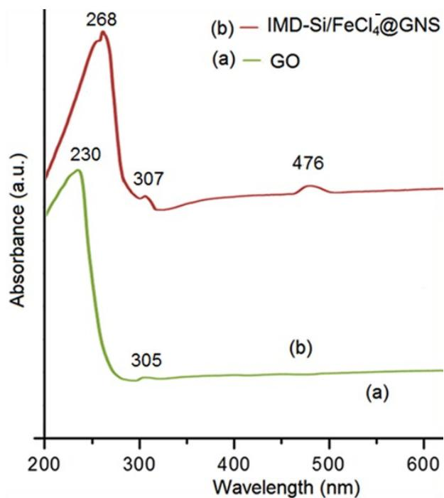
**Figure S1.** UV -Vis spectrum of (a) GO and (b) IMD-Si/FeCl<sub>4</sub><sup>-</sup>@GNS
