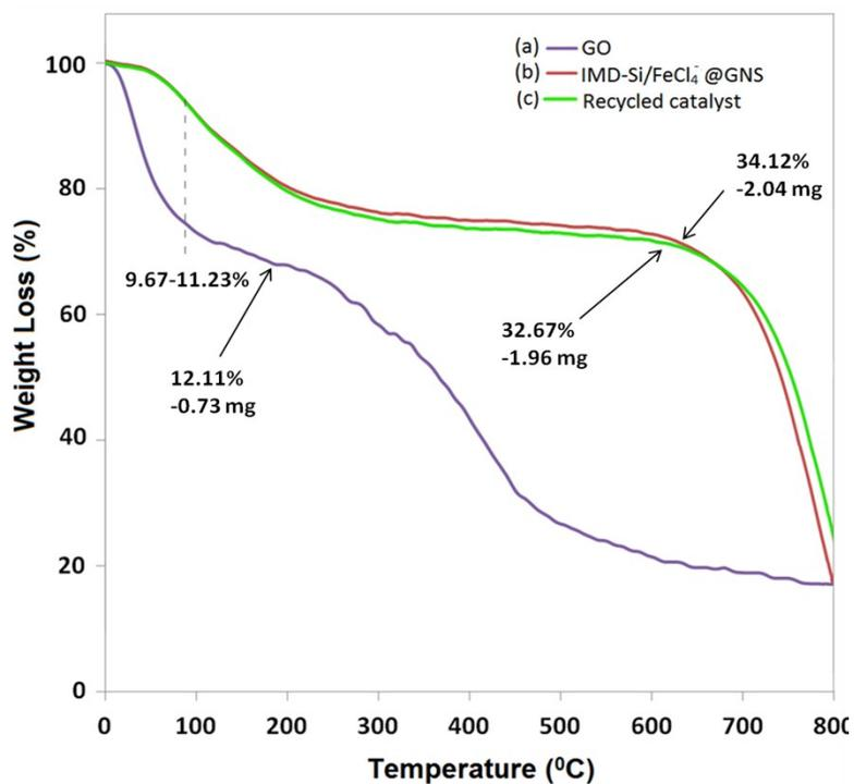
**Figure S2.** TG curves of (a) GO (b) IMD-Si/FeCl<sub>4</sub><sup>-</sup>@GNS and (c) Recycled catalyst
