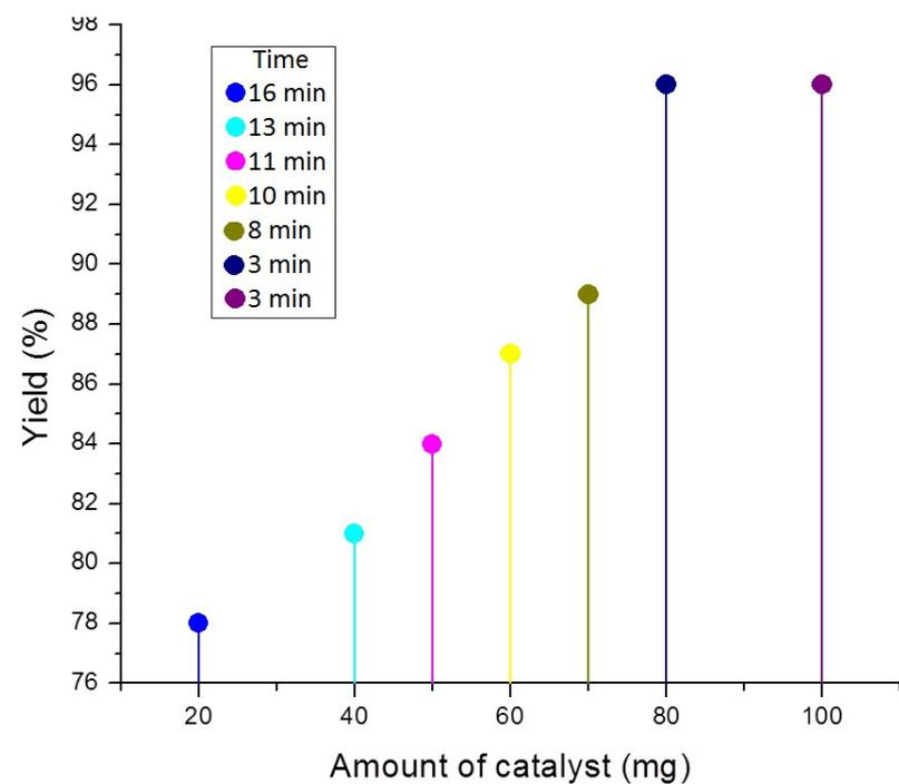
**Figure S4:** Effect of amount of material on model reaction<sup>a</sup> (<sup>a</sup>Reaction conditions: acetyl 1,3-dimethylbarbituric acid **1c** (2 mmol), thiosemicarbazide **2** (2 mmol), IMD-Si/FeCl<sub>4</sub><sup>-</sup>@GNS, T = 30°C. <sup>b</sup>Reaction progress monitored by TLC. <sup>c</sup>Isolated yield)
