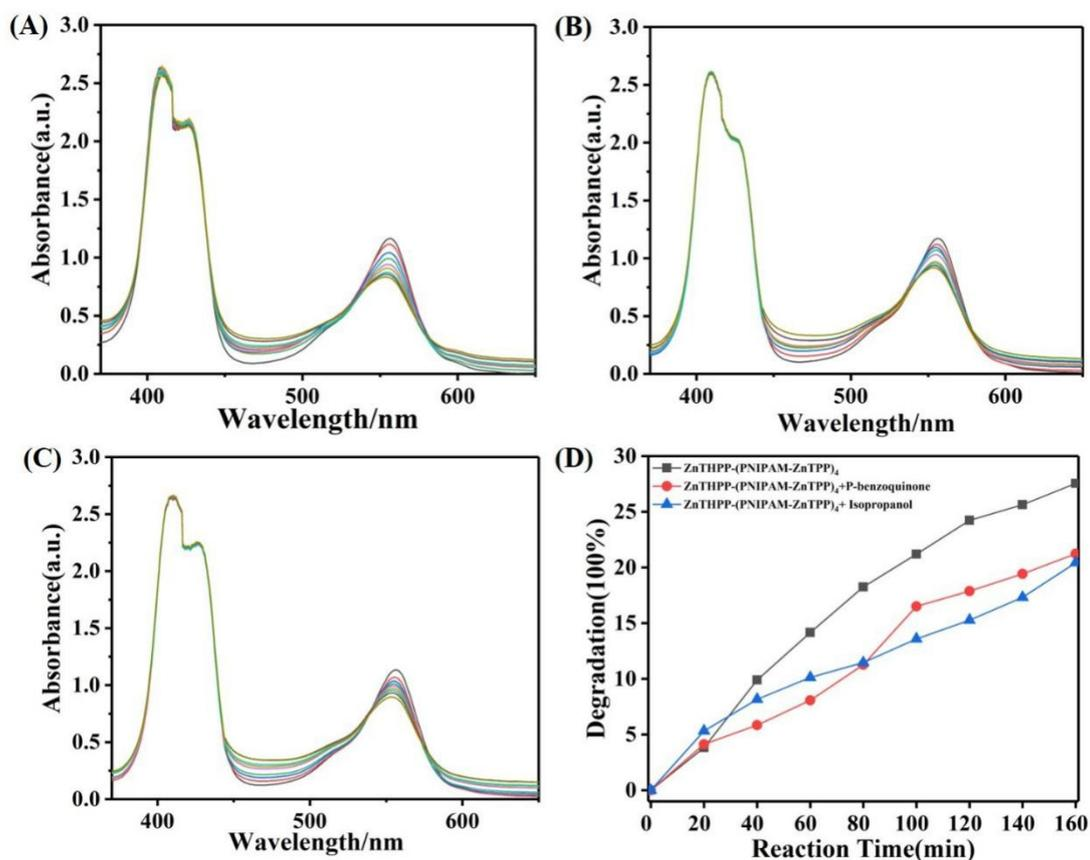
Fig. S7 UV-vis absorbance spectra of RhB degraded by photocatalytic upon visible light irradiation in the respective presence of (A) ZnTHPP-(PNIPAM-ZnTPP)<sub>4</sub>, (B) ZnTHPP-(PNIPAM-ZnTPP)<sub>4</sub> and p-benzoquinone, (C) ZnTHPP-(PNIPAM-ZnTPP)<sub>4</sub> and isopropanol. (D) The RhB degradation rates of ZnTHPP-(PNIPAM-ZnTPP)<sub>4</sub>, ZnTHPP-(PNIPAM-ZnTPP)<sub>4</sub>+p-benzoquinone and ZnTHPP-(PNIPAM-ZnTPP)<sub>4</sub> + isopropanol.
