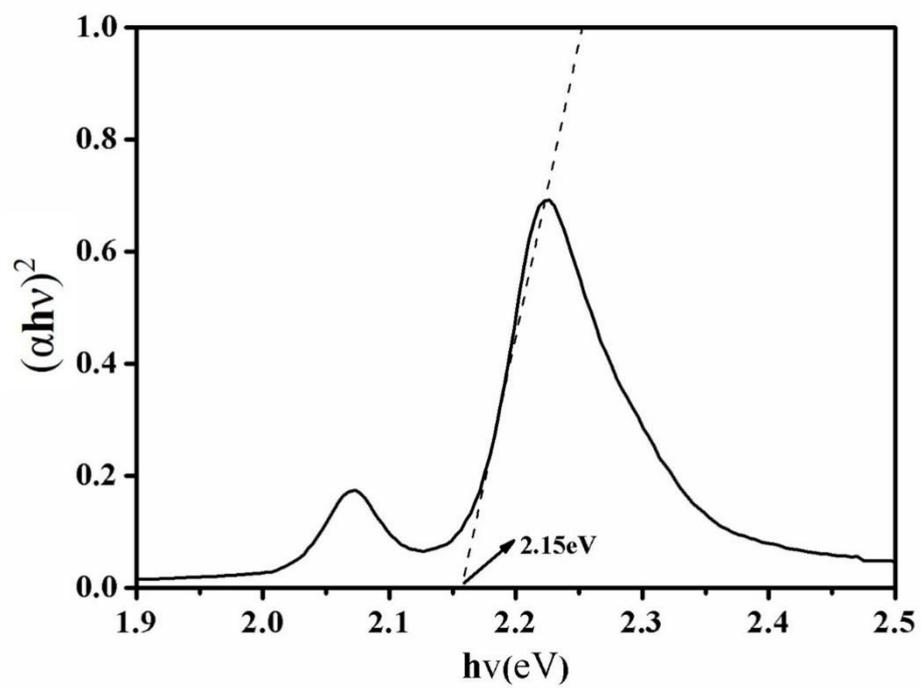
Fig. S6 Optical band gaps of ZnTHPP-(PNIPAM-ZnTPP)<sub>4</sub> obtained from UV-vis absorption spectra.
