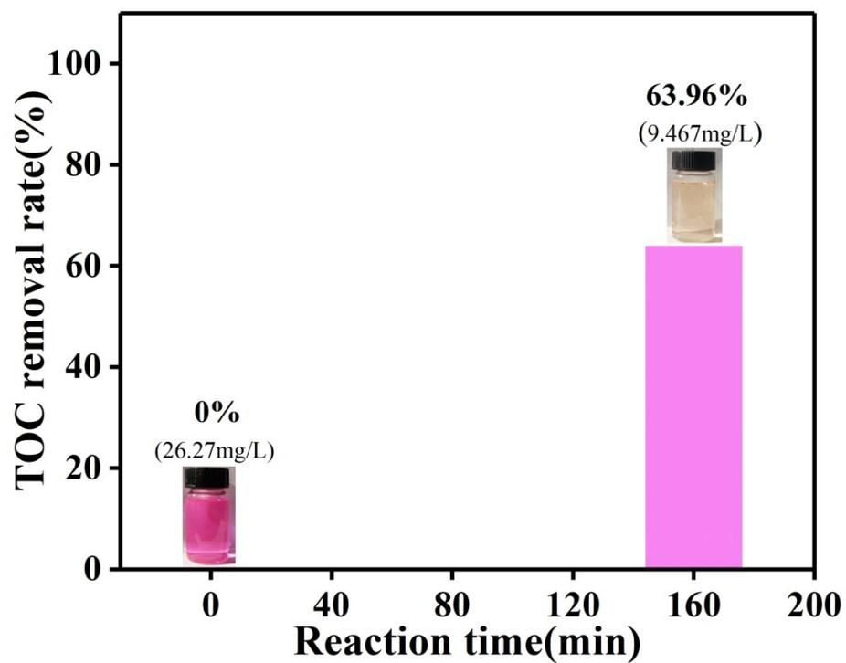
Fig. S5 Initial and final TOC changes during the course of RhB degradation in the presence of ZnTHPP-(PNIPAM-ZnTPP)<sub>4</sub> and H<sub>2</sub>O<sub>2</sub> under visible light radiation.
