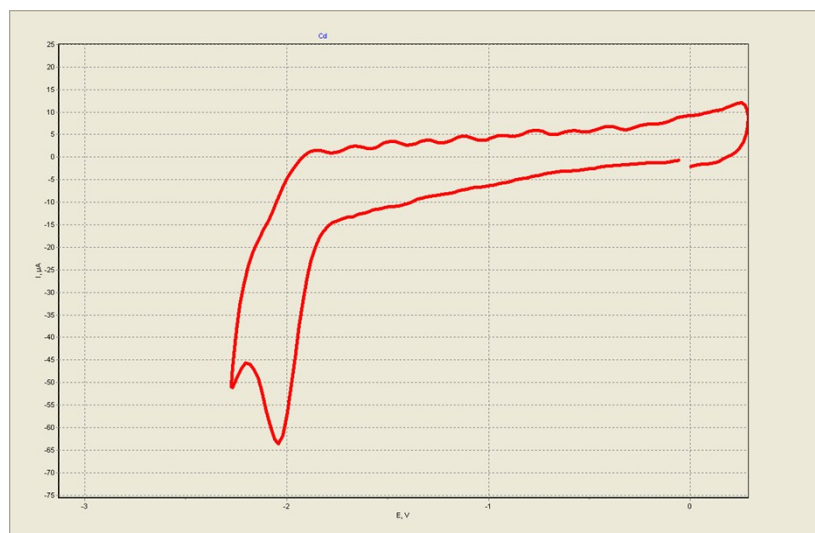
Fig. S12. Cyclic voltammograms of 2 obtained on GC electrode, E_0 = -1.98\text{V} 51mA
