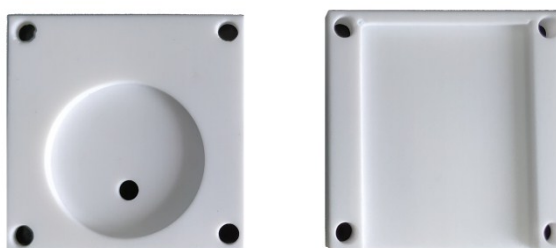
Fig.S1 The specially designed electrochemical cell used in this EC-SERS platform
