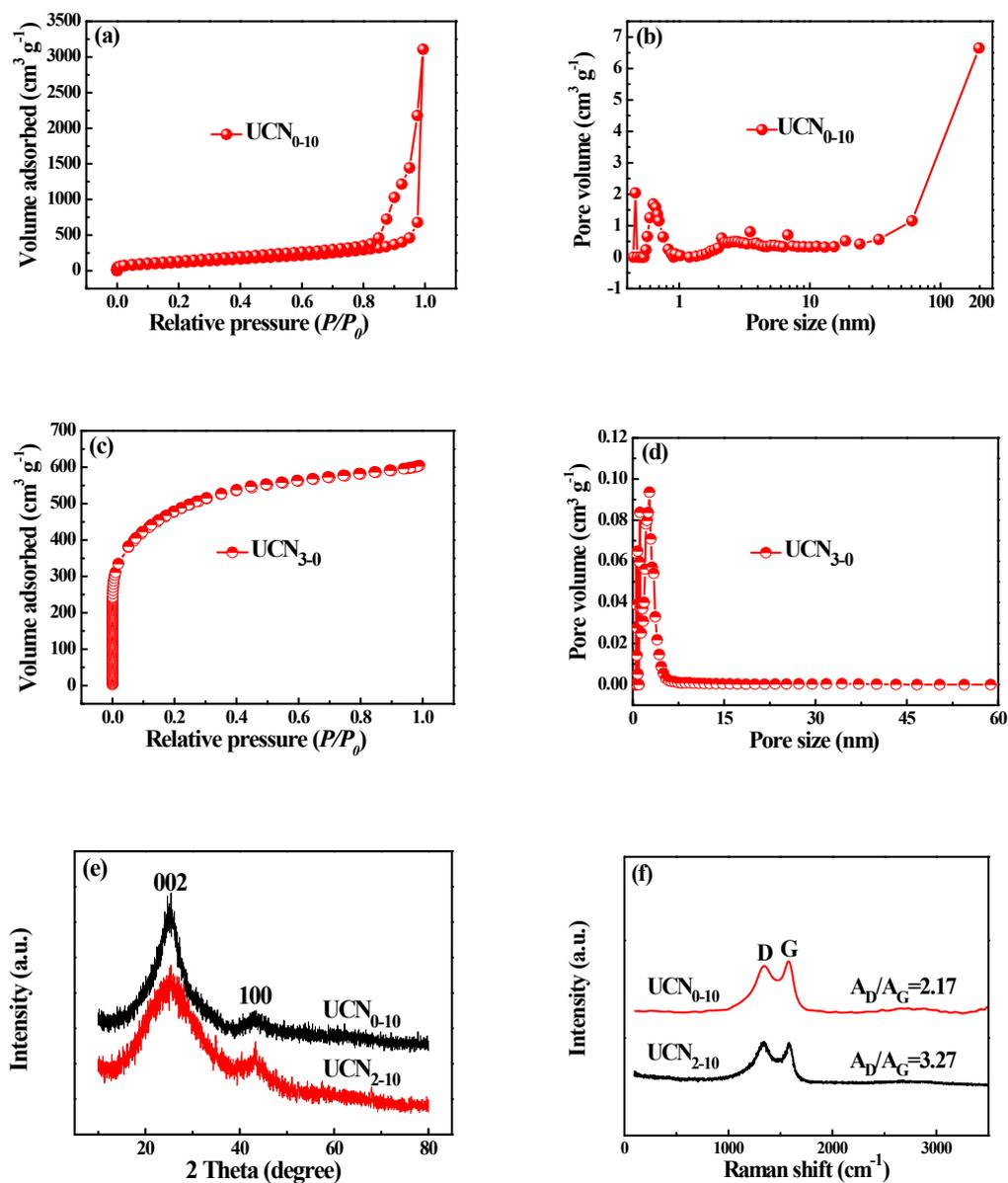
**Figure S4.** N<sub>2</sub> adsorption-desorption isotherms of: (a) UCN<sub>0-10</sub>, (c) UCN<sub>3-0</sub>. Pore size distribution curves of: (b) UCN<sub>0-10</sub>, (d) UCN<sub>3-0</sub>. (e) XRD patterns of UCN<sub>0-10</sub> and UCN<sub>2-10</sub>. (f) Raman spectra of UCN<sub>0-10</sub> and UCN<sub>2-10</sub>.
