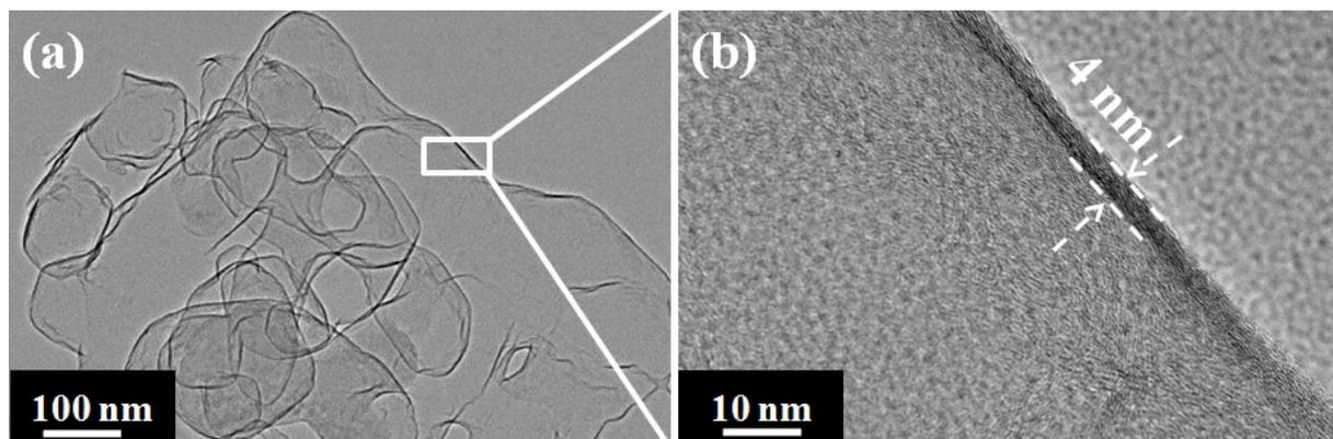
**Figure S2.** TEM images of (a, b)  $UCN^{0-10}$ .  $UCN^{0-10}$  is made on 2 g naked nano-MgO particles in another corundum boat.
