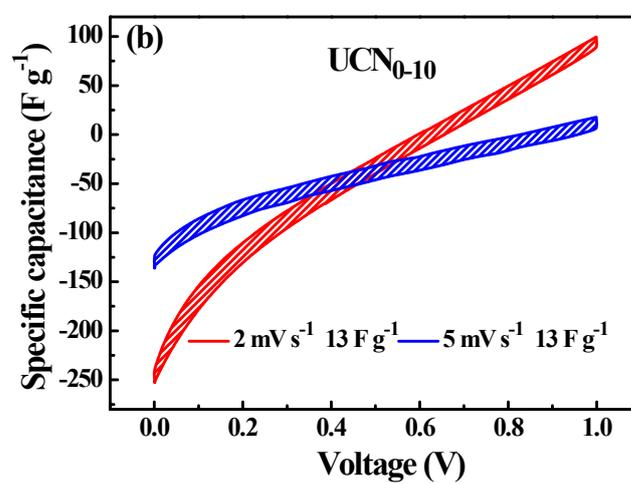
**Figure S9.** (a) CV curves of UCN<sub>3-10</sub> electrode at 2 and 5 mV s<sup>-1</sup>. (b) CV curves of UCN<sub>0-10</sub> electrode at 2 and 5 mV s<sup>-1</sup>.
