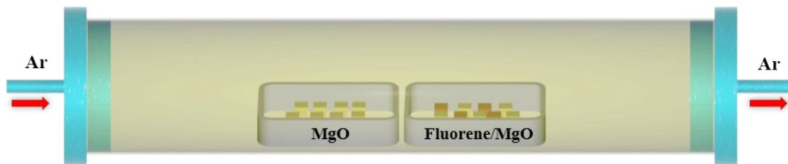
**Figure S3.** Schematic for the relative position of corundum boats in horizontal tubular furnace.
