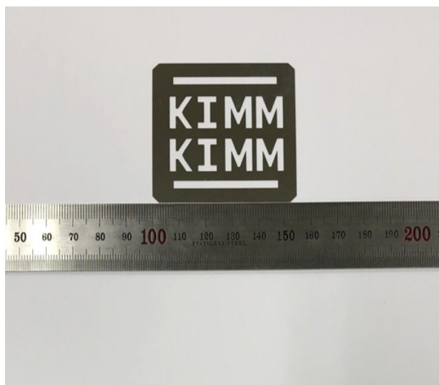
Fig. S3. Photograph of the mask used to deposit the metals on the polymer stamp at different angles.
