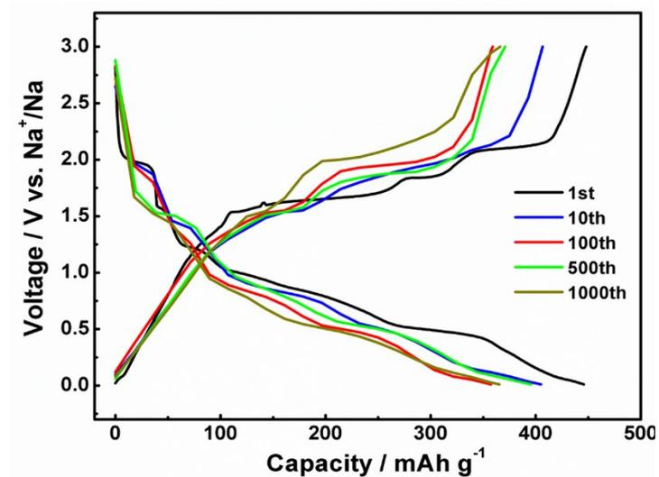
**Figure S8.** Discharge/charge profiles of  $\text{Cu}_9\text{S}_5\text{-AHP-1.5}$  at  $1000 \text{ mA g}^{-1}$ .
