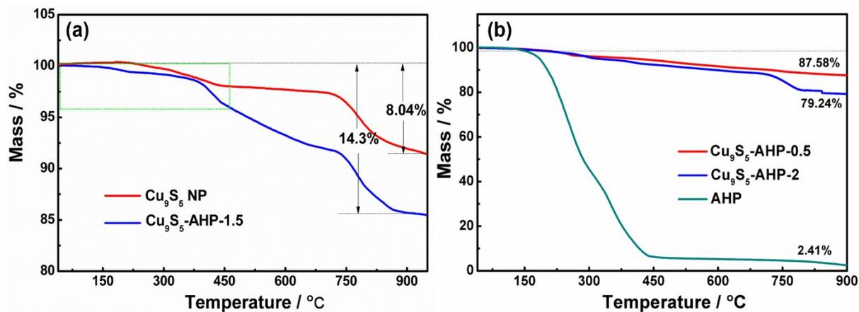
**Figure S3.** TGA curves of (a) Cu<sub>9</sub>S<sub>5</sub> NP and Cu<sub>9</sub>S<sub>5</sub>-AHP-1.5, (b) AHP, Cu<sub>9</sub>S<sub>5</sub>-AHP-0.5 and Cu<sub>9</sub>S<sub>5</sub>-AHP-2 in N<sub>2</sub> atmosphere at a heating rate of 10 °C min<sup>-1</sup>
