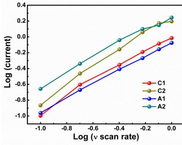
**Figure S10.**  $\text{Log}(i)$  vs  $\text{log}(v)$  plots for different redox peaks of  $\text{Cu}_9\text{S}_5\text{-AHP-1.5}$  electrode.
