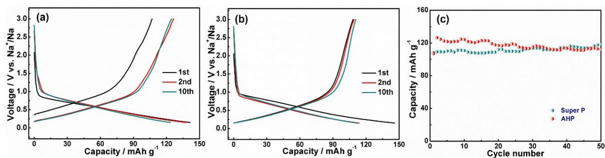
**Figure S6** Charge/discharge curves of (a) AHP and Super P (1:1), (b) Super P and cycling performance (c) at 100 mA g<sup>-1</sup>.
