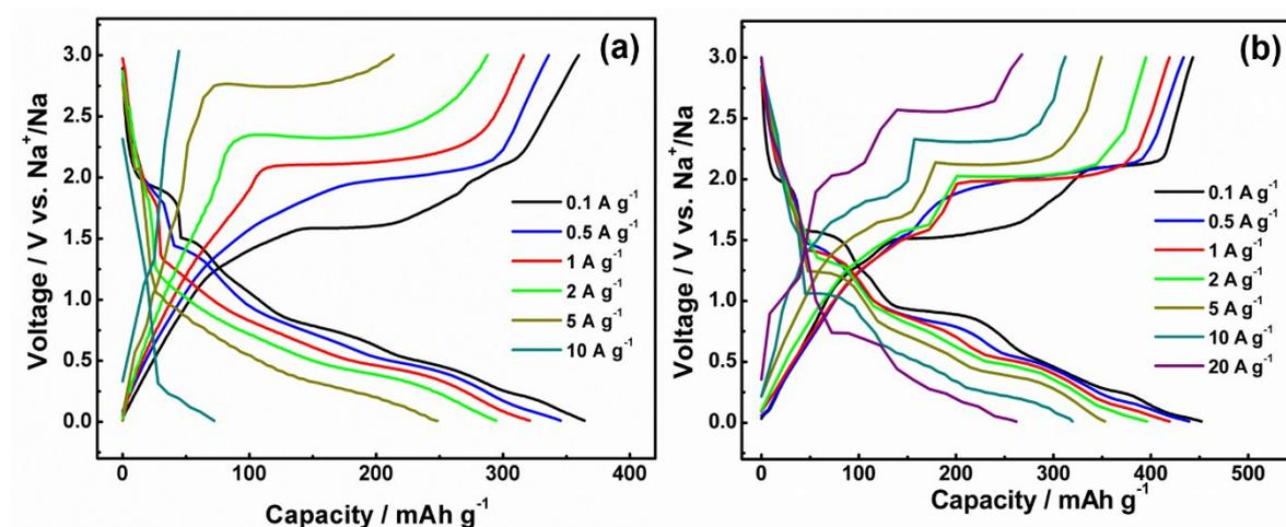
**Figure S7.** Charge/discharge curves of (a) Cu<sub>9</sub>S<sub>5</sub> NP and (b) Cu<sub>9</sub>S<sub>5</sub>-AHP-1.5 at various current densities.
