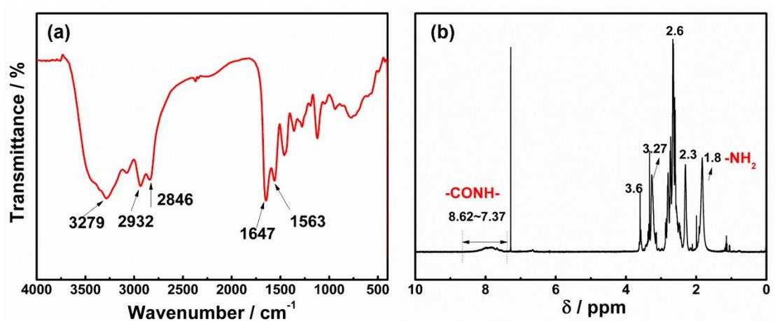
**Figure S2.** (a) The FT-IR spectra and (b)  $^1\text{H}$  NMR spectra of AHP.
