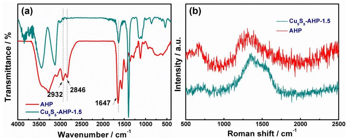
**Figure S4.** FT-IR (a) and Raman (b) spectra of Cu<sub>9</sub>S<sub>5</sub>-AHP-1.5 and AHP.
