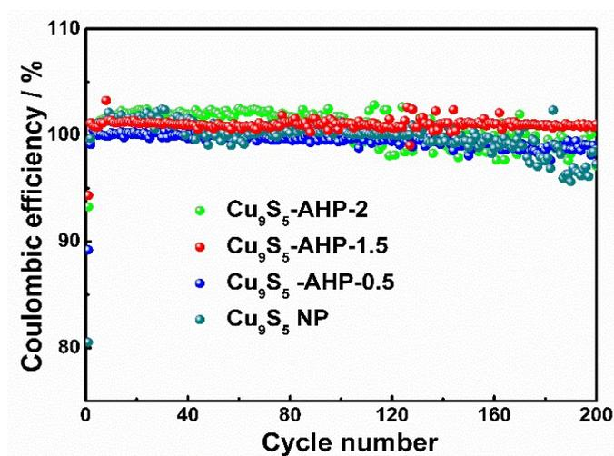
**Figure S5.** Coulombic efficiency in 1 M  $\text{NaPF}_6$  + DOL-DME (1:4 by volume) at 100  $\text{mA g}^{-1}$
