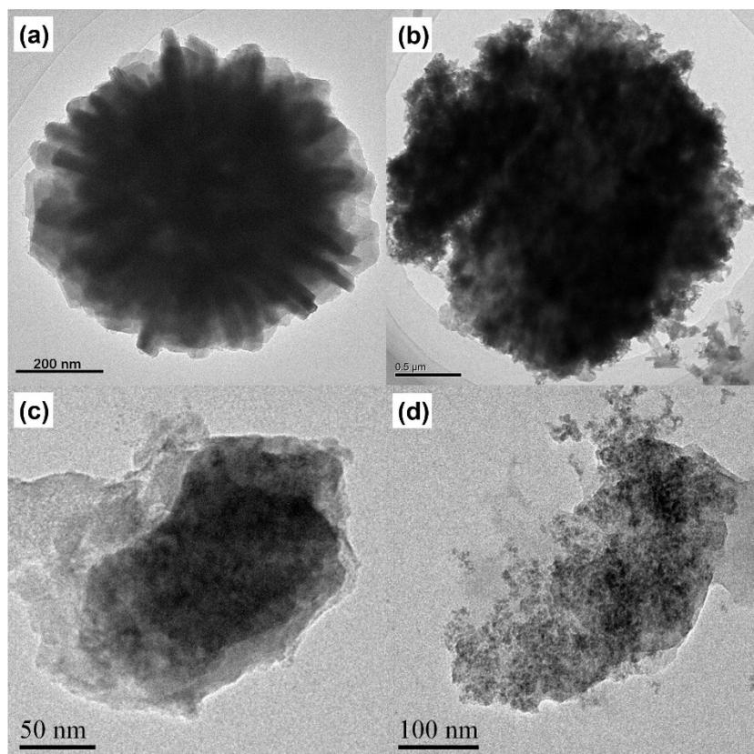
**Figure S9.** TEM images of  $\text{Cu}_9\text{S}_5\text{-AHP-1.5}$  (a) at initial state, (b) after 300 cycles and  $\text{Cu}_9\text{S}_5$  NP (c) at initial state, (d) after 300 cycles at  $100 \text{ mA g}^{-1}$ .
