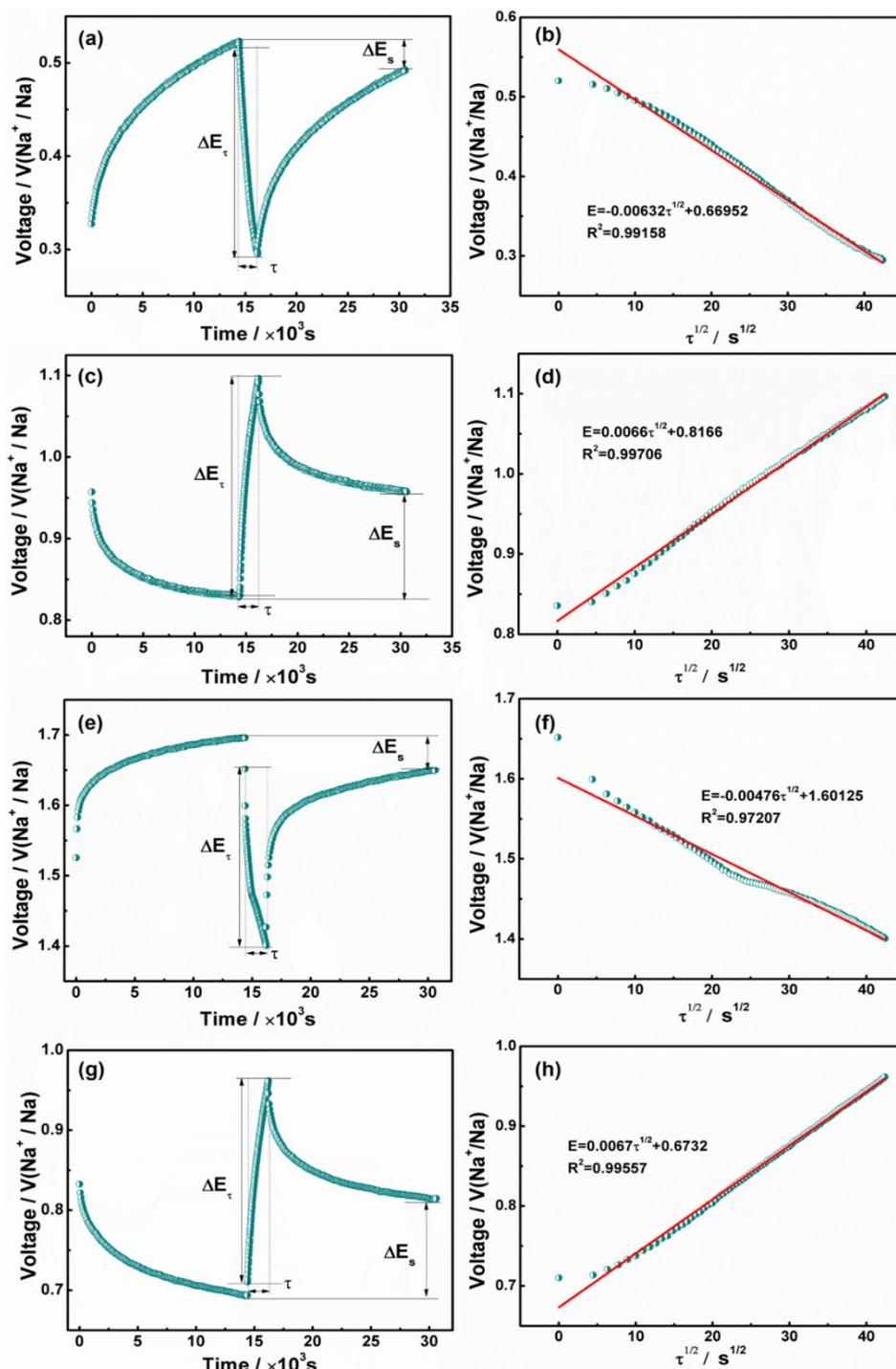
**Figure S12.** A single GITT titration and the corresponding linear behavior of  $E$  vs.  $\tau^{1/2}$  relationship: (a, b) Cu<sub>9</sub>S<sub>5</sub>-AHP-1.5 during discharge processes; (c, d) Cu<sub>9</sub>S<sub>5</sub>-AHP-1.5 during charge processes; (e, f) Cu<sub>9</sub>S<sub>5</sub> NP during discharge processes; (g, h) Cu<sub>9</sub>S<sub>5</sub> NP during charge processes.
