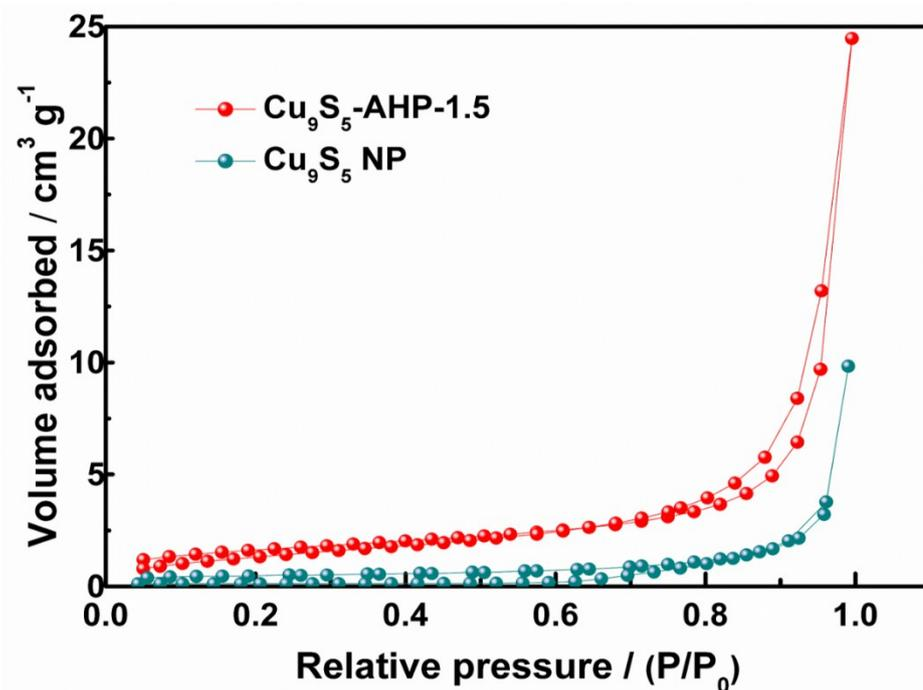
**Figure S13.** N<sub>2</sub> adsorption-desorption isotherm curves of Cu<sub>9</sub>S<sub>5</sub>-AHP-1.5 and Cu<sub>9</sub>S<sub>5</sub> NP. The specific surface areas of Cu<sub>9</sub>S<sub>5</sub>-AHP-1.5 and Cu<sub>9</sub>S<sub>5</sub> NP are 5.73 and 1.58 m<sup>2</sup> g<sup>-1</sup>, respectively.
