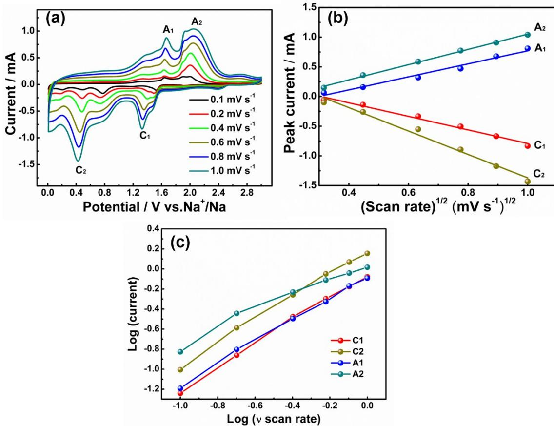
**Figure S11.** (a) CV curves at different scan rates, (b) linear relationship between peak current ( $i_p$ ) and square root of scan rate ( $\nu^{1/2}$ ), (c)  $\text{Log}(i)$  vs  $\text{log}(\nu)$  plots for different redox peaks of  $\text{Cu}_9\text{S}_5$  NP electrode.
