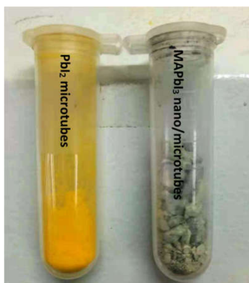
Figure S1 Photographic image of as-synthesized \text{PbI}_2 microtubes and \text{MAPbI}_3 nano/microtubes. The as-synthesized samples are dried in vacuum oven at 40 °C.
