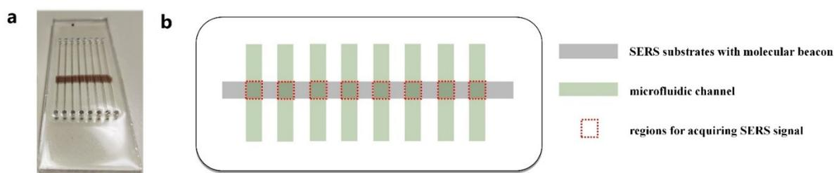
**Figure S5.** (a) Photo of the real chip (b) Schematic illustration of the regions for SERS signal acquisition (top view). The signal measured in each region corresponds to the sample flowed through its corresponding channel.
