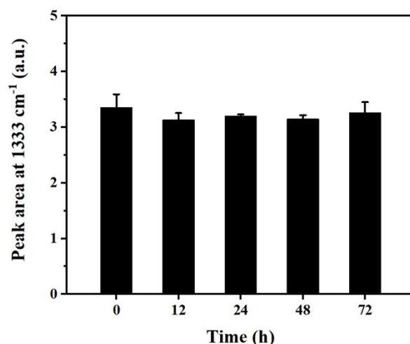
**Figure S2. Stability test of the SERS substrate.** Peak area at 1333 cm<sup>-1</sup> of DTNB molecules measured at different time after the fabrication of SERS substrate.
