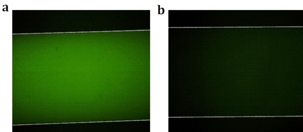
**Figure S8.** Fluorescence imaging of the DNA assay with 5nM target DNA (a) and the blank control (b). The scale bars indicate a length of 100  $\mu\text{m}$ . The channels are profiled by the dotted lines.
