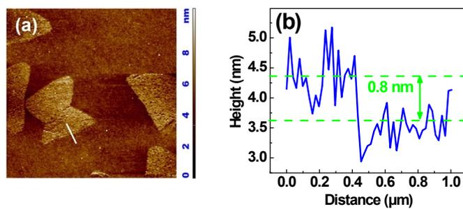
**Fig. S12.** (a) AFM image of pristine h-BN flakes transferred onto a SiO<sub>2</sub>/Si substrate. (b) Height profiles along the white lines drawn in (a), showing a thickness of 0.8 nm.
