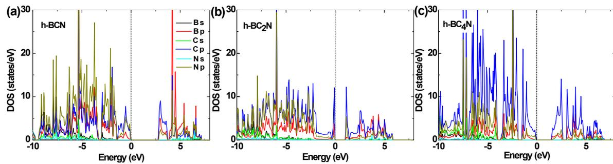
**Fig. S11.** The density of states (DOSs) of the (a) h-BCN, (b) h-BC<sub>2</sub>N, and (c) h-BC<sub>4</sub>N.
