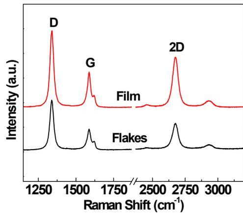
**Fig. S7.** Raman spectra of pristine graphene flakes and continuous film.
