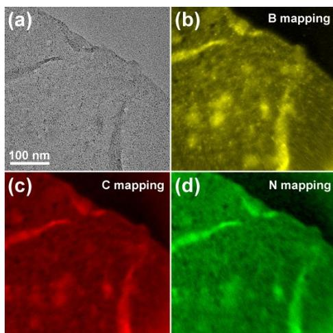
**Fig. S10.** (a) TEM image of an h-BNC film with 48 at.% C. The corresponding EELS mapping for (b) B, (c) C and (d) N in the h-BCN film.
