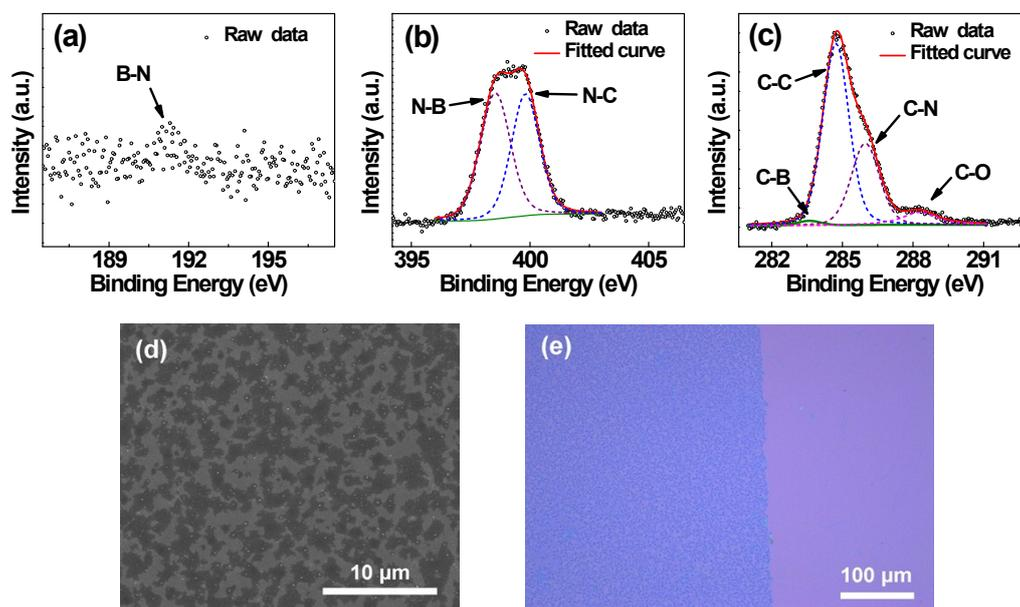
**Fig. S4.** Characterization of the h-BCN layer with 82 at.% C. XPS core level spectra of (a) B 1s, (b) N 1s, and (c) C 1s for the h-BCN sample grown with an ion beam aperture of 10 mm and 20 sccm CH<sub>4</sub>. The C content is determined to be 82 at.% in this sample. (d) SEM image of the h-BCN film with 82 at.% C. The formation of segregated graphene domains embedded in h-BCN matrix was observed. (e) Optical microscopy image of h-BCN film with 82 at.% C on a SiO<sub>2</sub>/Si substrate.
