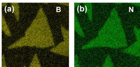
**Fig. S6.** (a) B (KLL) and (b) N (KLL) Auger electron maps of pristine h-BN flakes.
