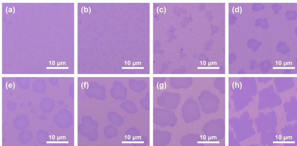
**Fig. S9.** Optical microscopy image of (a) pristine h-BN, and h-BCN flakes with (b) 4 at.%, (c) 16 at.%, (d) 35 at.%, (e) 48 at.%, (f) 58 at.%, (g) 67 at.%, as well as (h) pristine graphene transferred on SiO<sub>2</sub>/Si substrates.
