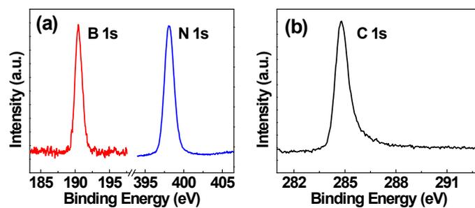
**Fig. S2.** XPS core level spectra of (a) B 1s and N 1s for pristine h-BN, (b) C 1s for pristine graphene.
