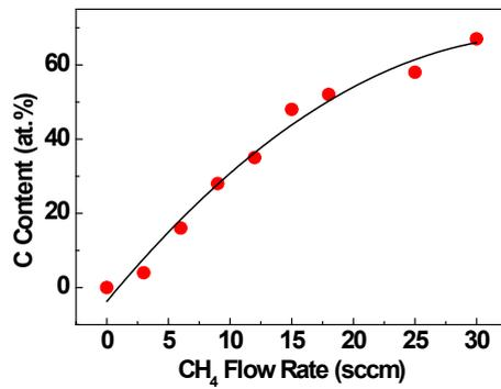
**Fig. S3.** Dependence of the C content in h-BCN layers on the CH<sub>4</sub> flow rate.
