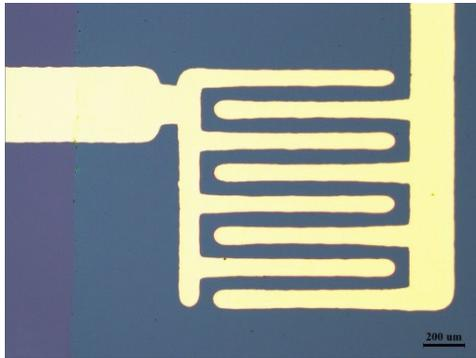
**Fig. S13.** Optical microscopy image of the h-BCN layers with interdigitated Ti/Au electrodes.
