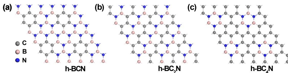
**Fig. S5.** Geometries of (a) h-BCN, (b) h-BC<sub>2</sub>N, and (c) h-BC<sub>4</sub>N with the lowest formation energies with respect to the chemical potential of h-BN and graphene.
