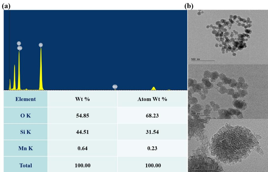
Figure. S1 (a). Elements analysis of  $MNH_s$ . (b). TEM images of  $MNH_s$  scale bar from up to down are 500 nm, 200nm and 20 nm. Table1. The element types O, Si, Mn and the atom weight respectively.
