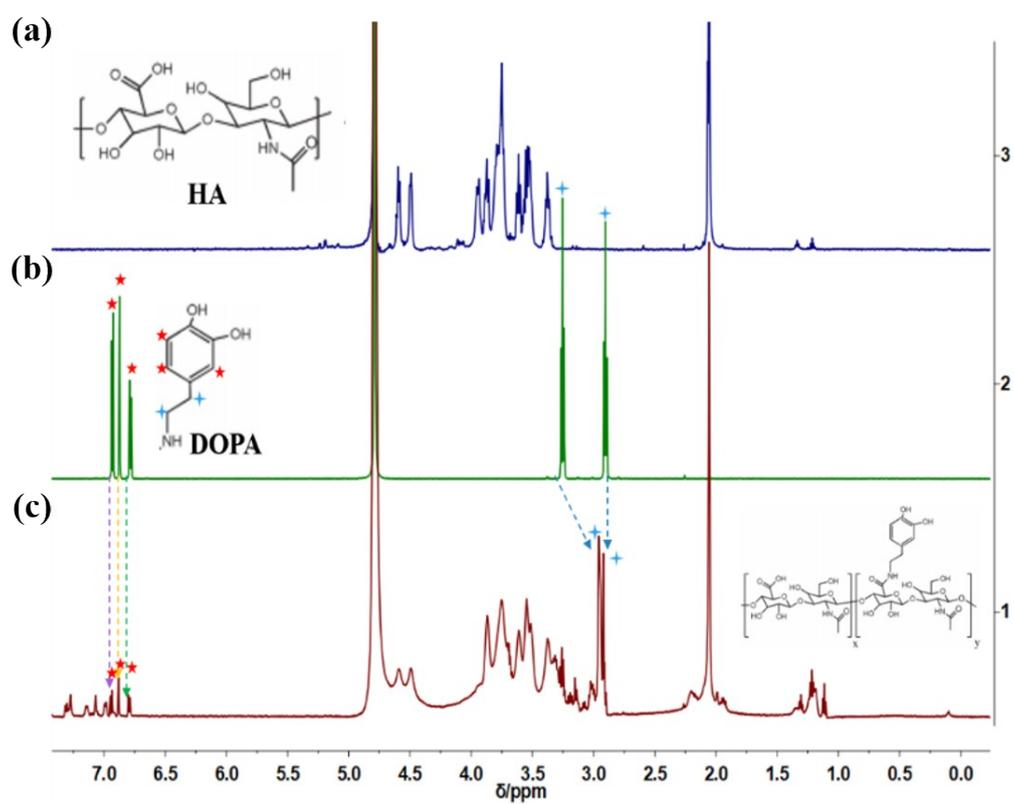
Figure. S4 (a).  $^1\text{H-NMR}$  spectrum of the unmodified hyaluronic acid (b)  $^1\text{H-NMR}$  spectrum of dopamine (c).  $^1\text{H-NMR}$  spectrum of HA-DN complex.
