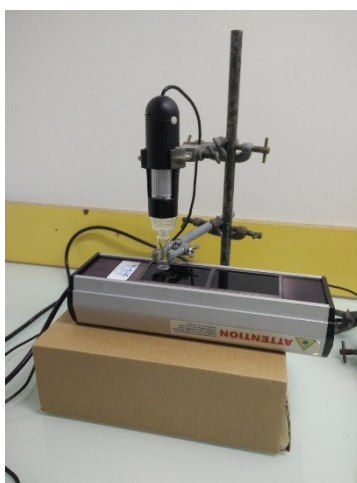
Supplementary Figure 5. Setup for recording gel contraction. See a typical recording of the contraction process in the supplementary video furnished.
