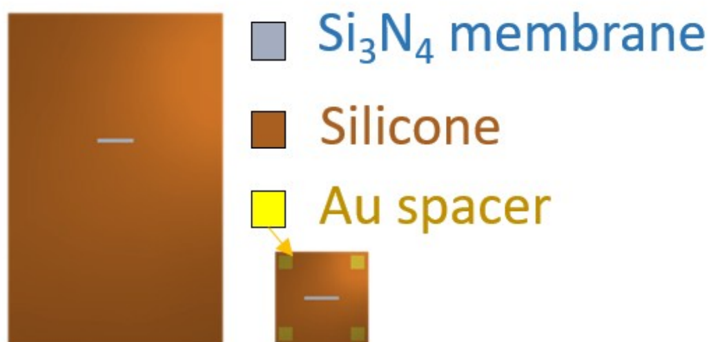
Figure S1. Schematic diagram of the specific E-chips used in the Protochips Poseidon 200. The left image is the top chip, and the right image is the bottom chip. The size of the bottom chip is 2.3 mm x 2.3 mm, and the thickness of the Au spacer is 150 nm for sealing the precursor solution. The size of the top chip is 4 mm x 5.8 mm. The center of each chip is the 60 nm thick \text{Si}_3\text{N}_4 membrane used as an observation area.
