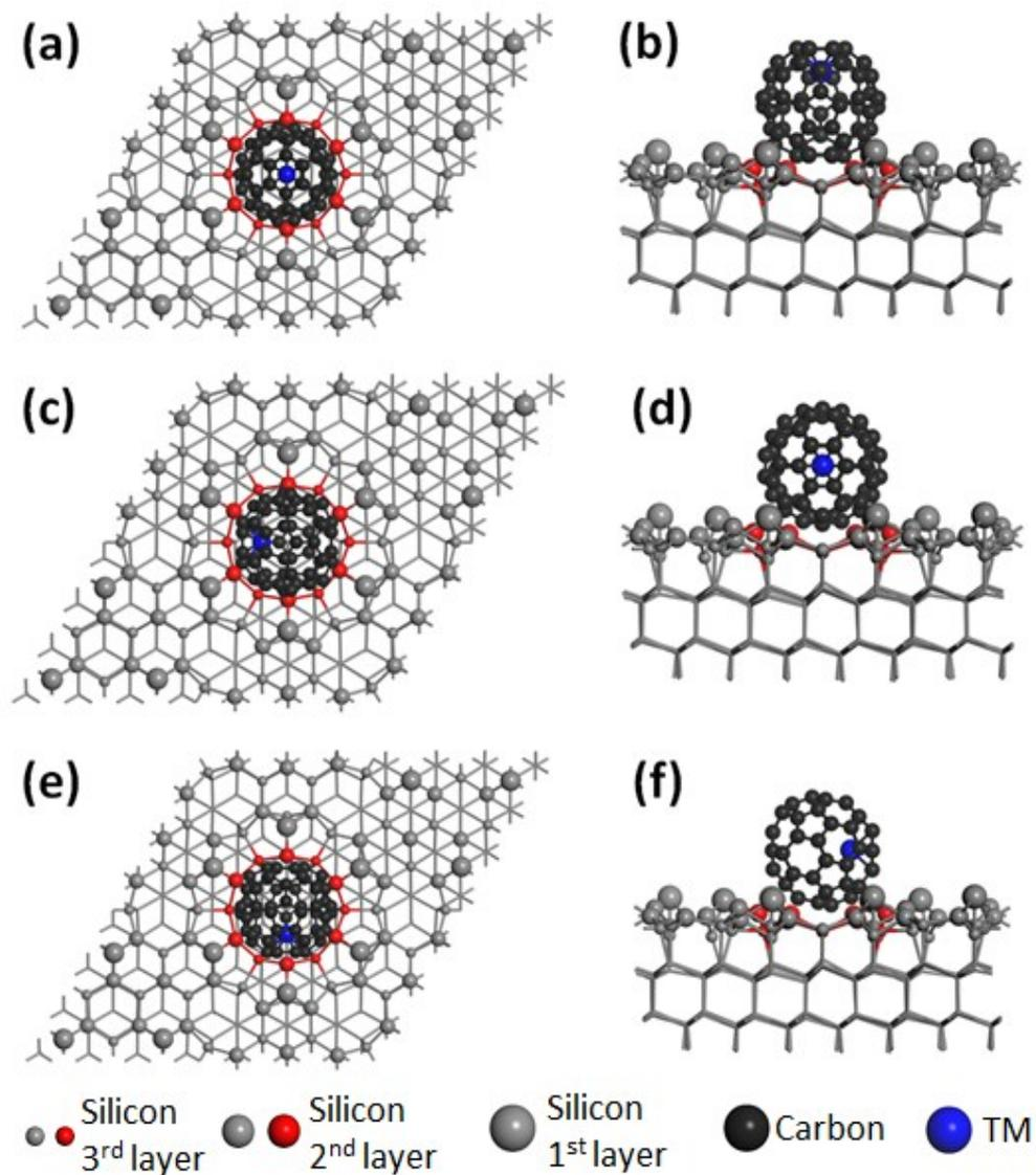
Figure S4. (a), (c) and (e) top view, and (b), (d), (f) side view of TM@C<sub>60</sub> adsorb inside the corner hole of Si(111)-(7×7) with different orientations.
