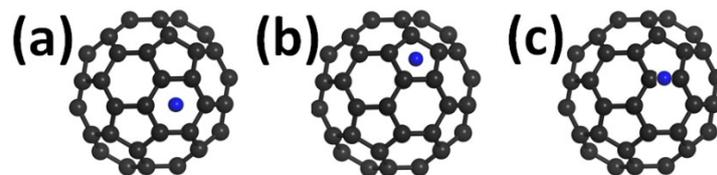
Figure S2. Possible adsorption sites of TM atoms inside a  $C_{60}$  molecule that considered in our calculations. (a) near the center of a six-membered ring, (b) near the center of a five-membered ring, and (c) near the center of a C-C bridge.
