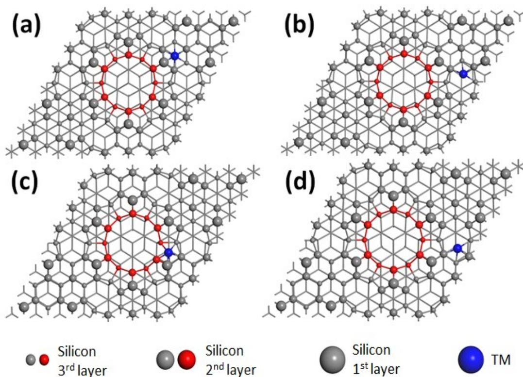
Figure S1. Top view of TM atoms adsorb on various sites of the Si(111)-(7×7) outside the corner hole. The corresponding adsorption energies are listed in table S1.
