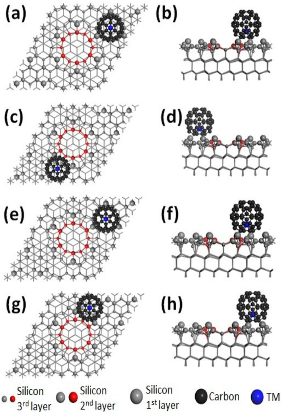
Figure S3. (a), (c), (e), (g) Top view and, and (b), (d), (f), (h) side view of TM@C<sub>60</sub> adsorb on the surface of the Si(111)-(7×7) outside the corner hole.
