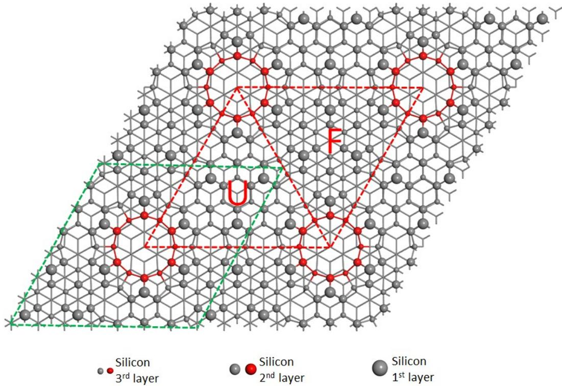
Figure S0. The red dashed lines indicate a usually used unit cell of Si(111)-7x7 surface. The letters “F” and “U” show the faulted and unfaulted half unit cells, respectively. While the unit cell we used in the current paper is the one shown with the green lines.
