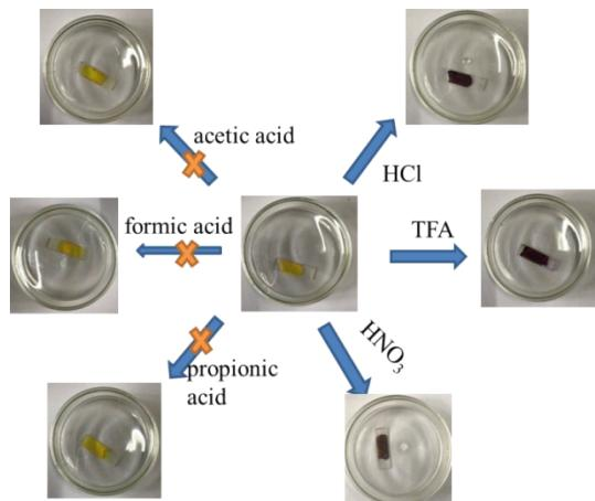
**Figure S9** Images of film 1 with sensing different acids.
