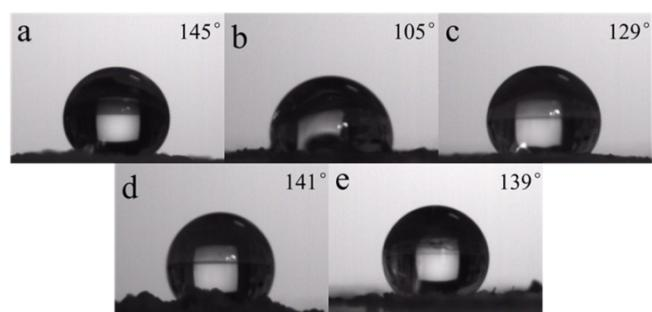
**Figure S17** Water contact angle of xerogel **1** formed in acetonitrile (a) and xerogels **1** upon addition of 1.0 eq. (b)  $\text{Hg}^{2+}$ , (c)  $\text{Fe}^{3+}$ , (d)  $\text{Cu}^{2+}$  and (e) TFA.
