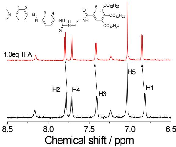
**Figure S7**  $^1\text{H}$ NMR of **1** before and after addition of 1.0 eq. TFA in  $\text{CD}_3\text{CN}$ . Inset showing assigned protons of **1** for convenience.
