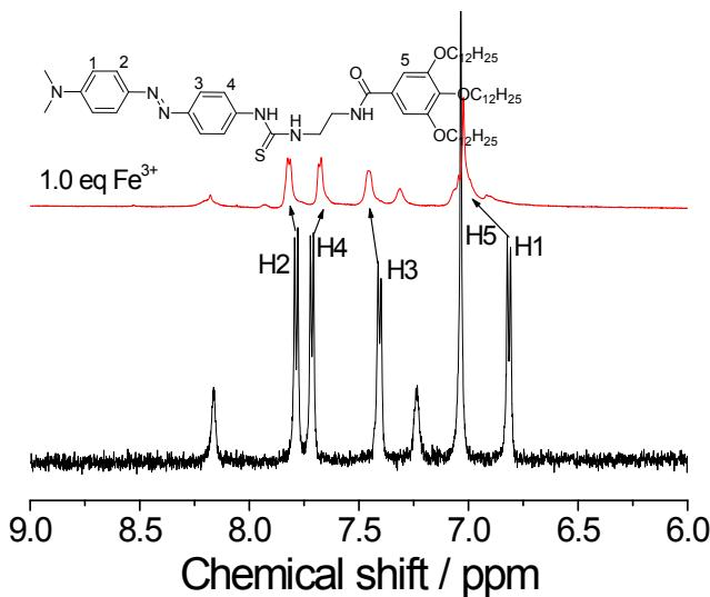
**Figure S5**  $^1\text{H}$ NMR of **1** before and after addition of 1.0 eq.  $\text{Fe}^{3+}$  in  $\text{CD}_3\text{CN}$ . Inset showing assigned protons of **1** for convenience.
