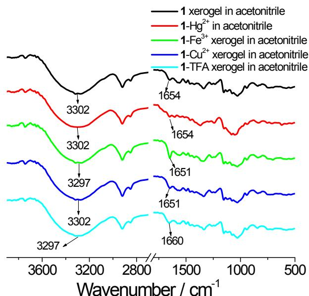
**Figure S14** FTIR spectra of xerogels **1** formed in acetonitrile solution and the changes in the gel state of **1** upon addition of  $\text{Hg}^{2+}$  ion,  $\text{Fe}^{3+}$  ion,  $\text{Cu}^{2+}$  ion and TFA in acetonitrile solution.
