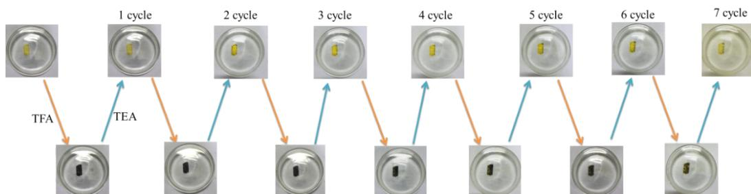
**Figure S11** Images of film 1 with sensing TFA and TEA in turn for seven cycle times.
