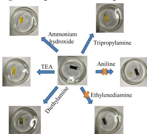
**Figure S10** Images of film 1 with TFA contacting different amines.
