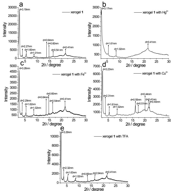
**Figure S16** XRD patterns of xerogel **1** from acetonitrile (a) and xerogels **1** upon addition of 1.0 eq. (b) Hg<sup>2+</sup>, (c) Fe<sup>3+</sup>, (d) Cu<sup>2+</sup> and (e) TFA.
