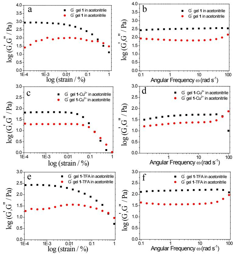
**Figure S15** Rheological tests of gel **1**, gels **1** with 1.0 eq. Cu<sup>2+</sup> and TFA at the CGC at 20°C. (a) Strain sweep at 6.28 rad s<sup>-1</sup>, (b) frequency sweep at 0.1% amplitude within the linear regime.
