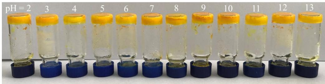
**Figure S12** Images of gels **1** with addition of different pH buffer onto the top of gel surface.
