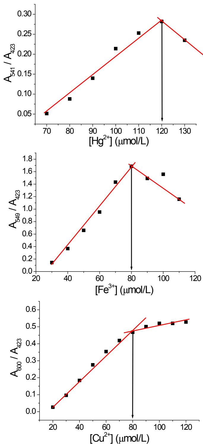
**Figure S4** Plots of  $[A_{541}/ A_{423}]$ ,  $[A_{549}/ A_{423}]$  and  $[A_{600}/ A_{423}]$  v/s increasing concentration of Hg<sup>2+</sup>, Fe<sup>3+</sup> and Cu<sup>2+</sup>.
