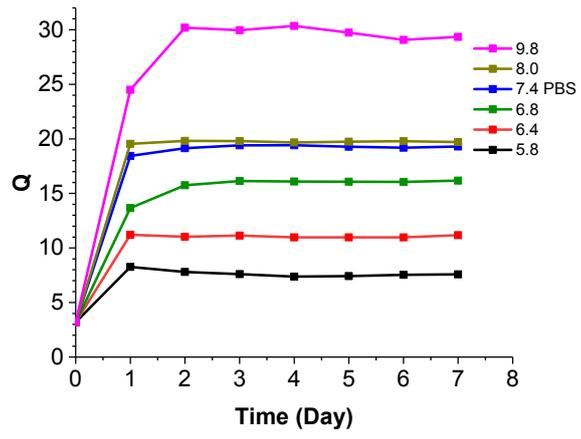
**Figure S8.** Variation of volume swelling ratio (Q) at different pH conditions for the NG-13-PEG-20-6000 gel.
