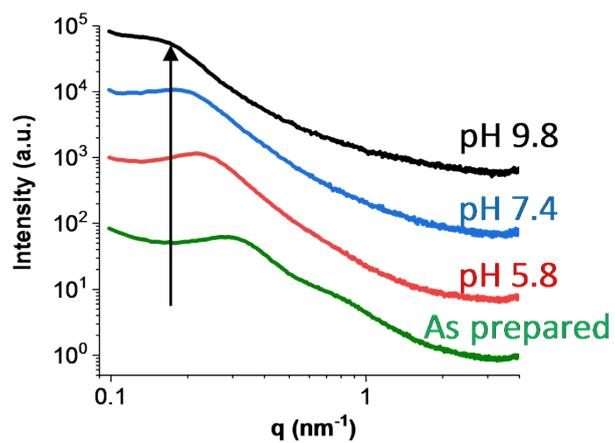
**Figure S9.** SAXS data for the NG-13-PEG-20-6000 gel as prepared and after swelling in different pH conditions for 24 hour. The arrow indicates the principle scattering peak.
