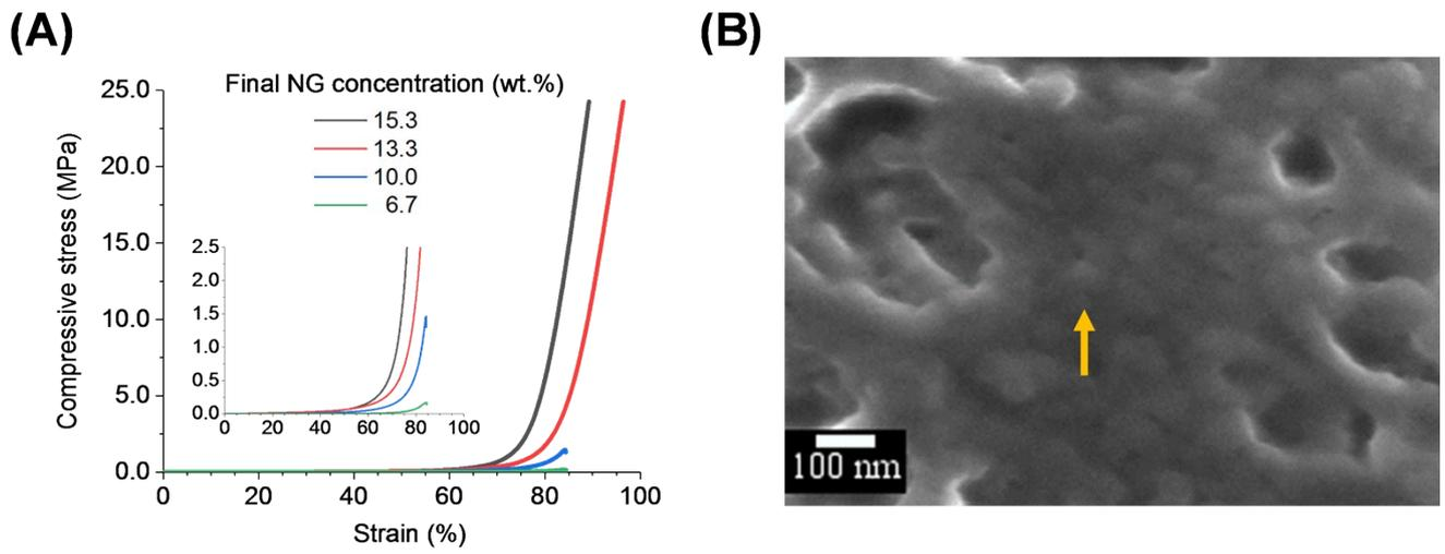
**Figure S5.** (A) Compressive stress vs. strain data for the NG-x-PEG-20-6000 gels with different final NG concentration ratio (x = 6.7 -15.3 wt.%). (B) SEM image for NG-13-PEG-20-6000 gel. Yellow arrow indicates the NG particle.
