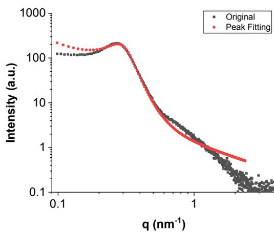
**Figure S6.** Example of Lorentzian peak fitting in SAXS data, conducted in Igor Pro software for the pre-gel mixture for NG-13-PEG-20-6000 gel.
