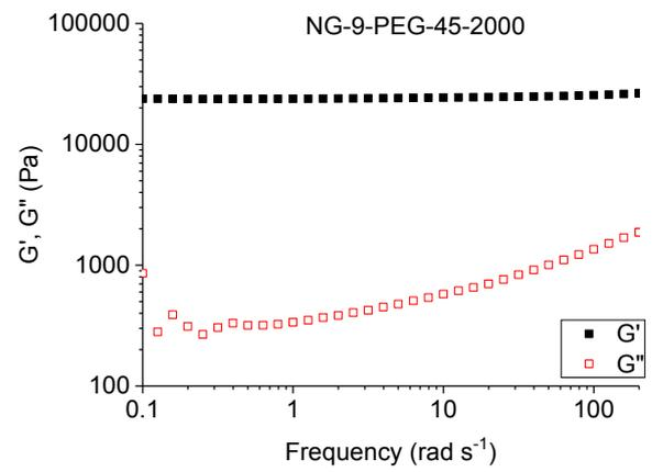
**Figure S3.** Frequency sweep rheology data for (A) NG-9-PEG-45-1000 gel and (B) NG-9-PEG-45-2000 gel.
