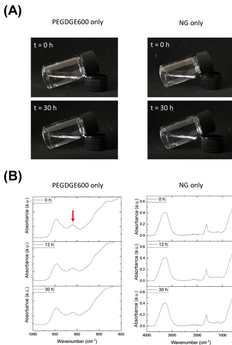
**Figure S2.** (A) Digital photographs of the inverted vial test. The tube containing either NG or PEGDGE600 did not form a gel. (B) FTIR study on the kinetic of the formation of PEGDGE600-based nanocomposite hydrogel at time  $t = 0, 12$  and  $30$  hour for solutions of (Left) PEGDGE600 only, red arrow indicates the epoxide band; (Right) NG only. There are no significant changes with different time intervals.
