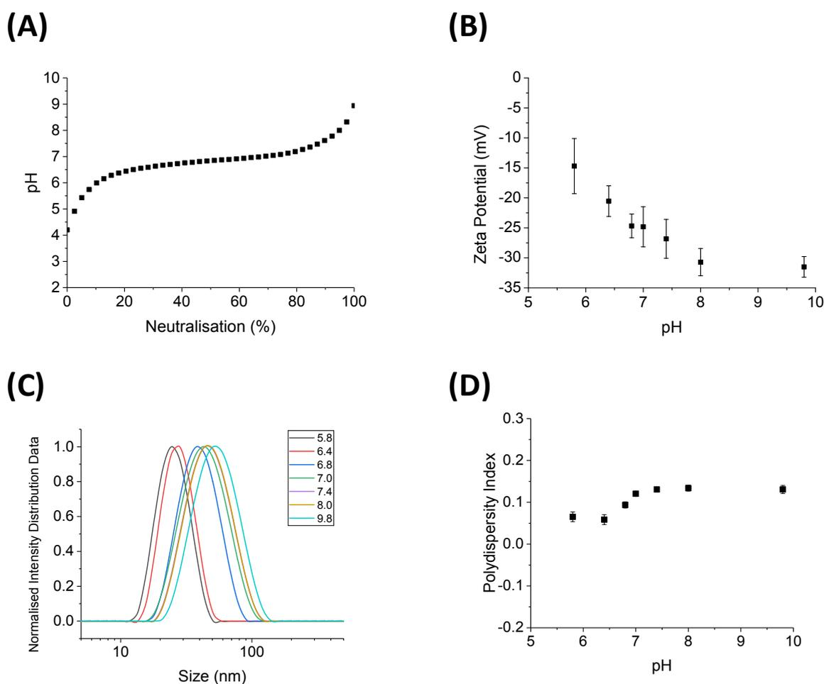
**Figure S1.** (A) Potentiometric titration data for the nanogels (NGs). (B) Variation of zeta potential with pH. (C) Dynamic light scattering (DLS) size distribution. (D) Polydispersity Index from DLS.
