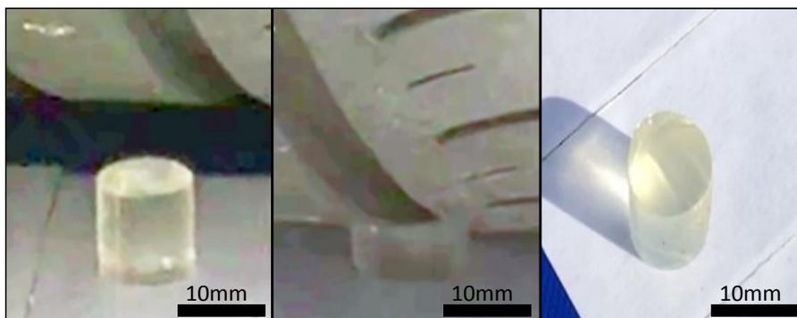
**Figure S4.** Crush experiment where the NG-13-PEG-20-6000 gel was run over by a rear tyre of a 1.0 tonne car (see Video S1, ESI+). Images are captured from Video S1. All hydrogels were prepared under same conditions for 72 h at 37°C with a constant initial solid content of the NG of 20.0 wt.%.
