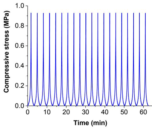
**Figure S7.** Compressive stress vs. time curves. Repetitive loading and unloading compressive cycles for the NG-13-PEG-20-6000 gel.
