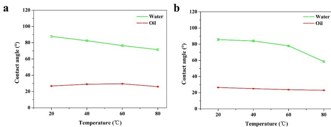
**Fig. S5** (a-b) The contact angle of water and oleic oil on various temperature relative to Sample-2 and Sample-3 respectively.
