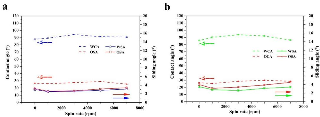
**Fig. S7** (a-b) The contact angle and sliding angle of water and oleic oil on various spin rate relative to Sample-2 and Sample-3 respectively.
