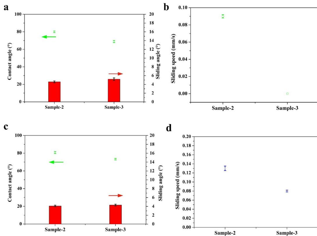
**Fig. S4** (a) After heating at 120°C for 15 min, the variation of water contact angle and sliding angle of Sample-2,3. (b) After heating at 120°C, the sliding speeds of 5uL Sample-2,3. (c) After immersed into boiling water for 15 min, the changes of contact angle and sliding angle of Sample-2,3. (d) After immersed into boiling water for 15 min, the sliding speeds of Sample-2,3.
