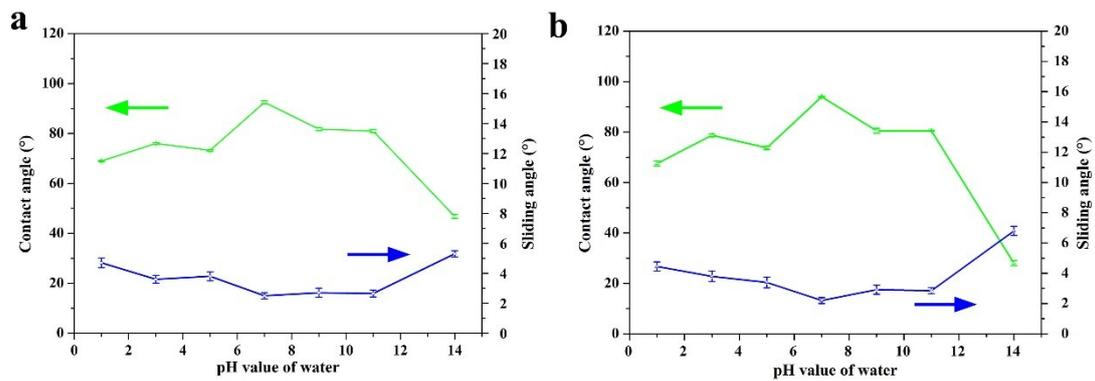
**Fig. S8** (a-b) The variation of contact angle and sliding angle of water on various pH value ranged from 1 to 14 relative to Sample-2 and Sample-3 respectively.
