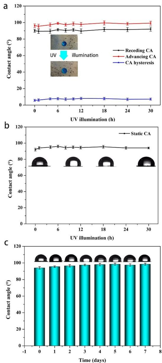
Fig. S3 (a) the variations of receding contact angle, advancing contact angle and contact angle hysteresis under various times of exposure to UV light. (b) Static contact angles of water on slippery surface (Sample-1) under various times of exposure to UV light. (c) Static contact angles of water on slippery surface (Sample-1) as a function of the outdoor storing time. The slippery sample was placed outside and horizontal with ground for 7 days at March 2015 in Lanzhou, China.
