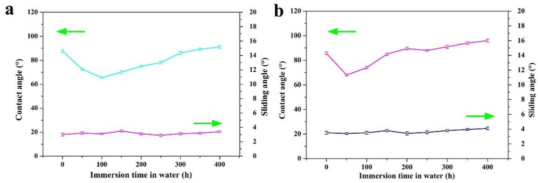
**Fig. S6** (a-b) The changes of contact angle and sliding angle of water on different immersion time relative to Sample-2 and Sample-3 respectively.
