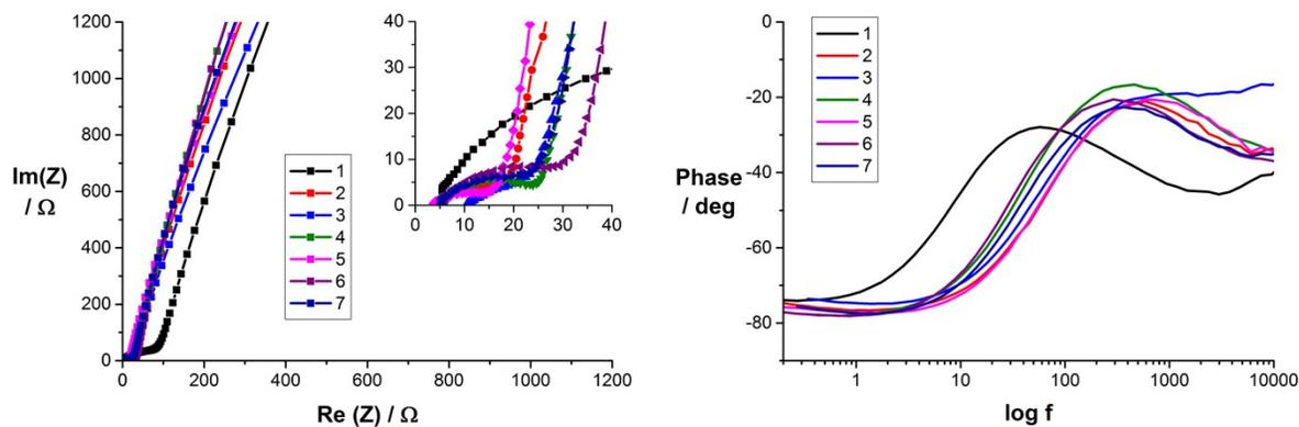
Figure S19. Left: Nyquist impedance plots of coin cell capacitors assembled with electrodes of samples 1 – 7 in 0.5 M TBAPF<sub>6</sub> in acetonitrile as the electrolyte; Right: Phase angle plots of coin cell capacitors assembled with electrodes of samples 1 – 7 with 0.5 M TBAPF<sub>6</sub> in acetonitrile as the electrolyte.
