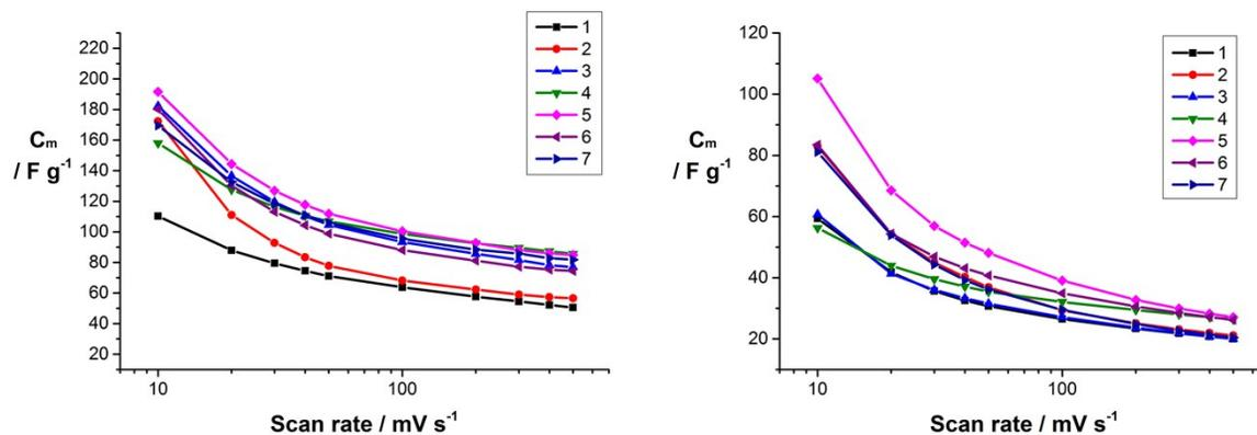
**Figure S13.** Specific gravimetric capacitances of samples 1 – 7 as a function of the scan rate in 6.0 M KOH (left) and in 0.5 M TBAPF<sub>6</sub> in acetonitrile as electrolyte (right).
