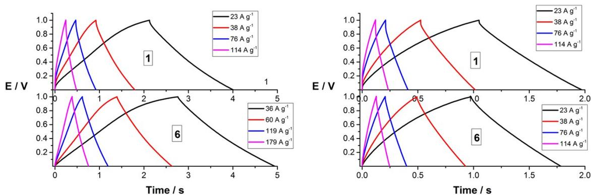
**Figure S14.** Galvanostatic charge discharge curves of samples **1** and **6** obtained at different current densities in 6.0 M KOH (left) and 0.5 M TBAPF<sub>6</sub> in acetonitrile (right).
