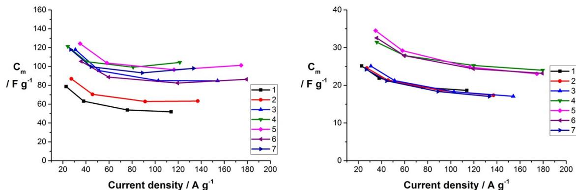
**Figure S15.** Specific gravimetric capacitances of samples **1** – **7** as a function of the current density in 6.0 M KOH (left) and in 0.5 M TBAPF<sub>6</sub> in acetonitrile as electrolyte (right).
