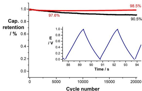
**Figure S16.** Capacitance retention of capacitor cells with sample **1** (black) and sample **6** (red) in 6.0 M KOH after 20,000 charge discharge cycles. Inset: Galvanostatic charge discharge curves of sample **6** obtained with a current density of 7.5 A g<sup>-1</sup>.
