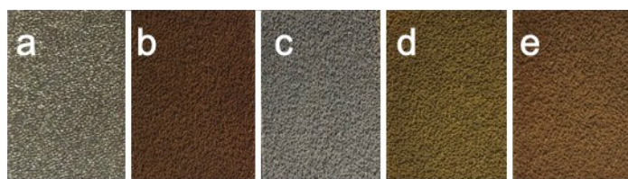
Fig. S1 Photographs of the as-synthesized samples (a: bare NF, b: FeCo CH/NF, c: CoNi CH/NF d: FeNi CH/NF and e: Co-FeNi CH/NF).
