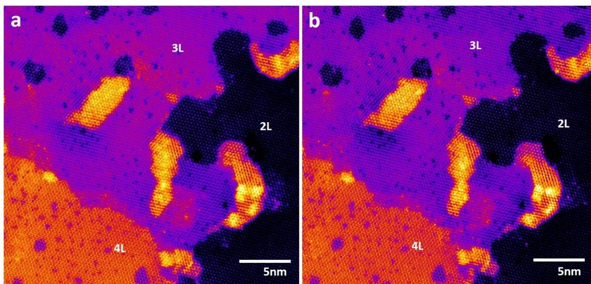
**Figure S12.** Continuous ADF-STEM image showing that no new defects and radical defect extension by electron beam irradiation for multilayer WS<sub>2</sub> have occurred. The time interval of this continuous image is 4 min 17 sec.
