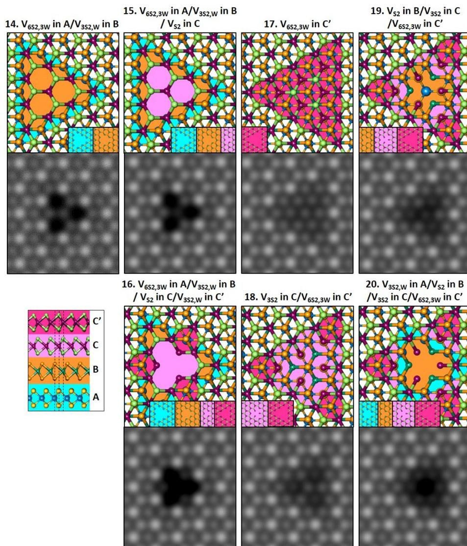
**Figure S9.** Atomic models and multislice ADF-STEM image simulations corresponding to the all atomic models showing the existing type of pores in ABCC' stacked quadralayer  $WS_2$ , further.
