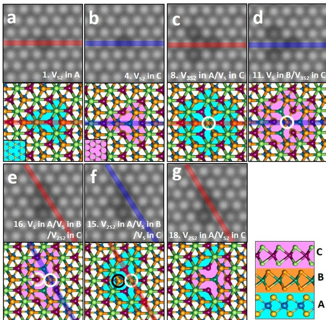
**Figure S6.** Atomic models and multislice ADF-STEM image simulations corresponding to the all atomic models showing the type of pores in Figure 6. Selected lines (red and blue) indicate the region of measured intensity line profiles in Figure 6. White-lined circles indicate S vacancies and black-lined circle indicates an S vacancy in B.
