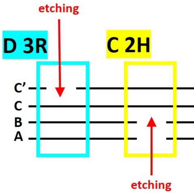
**Figure S10.** Schematic illustration of formation 3R stacked trilayer and 2H stacked bilayer WS<sub>2</sub> in the quadralayer according to etching directions.
