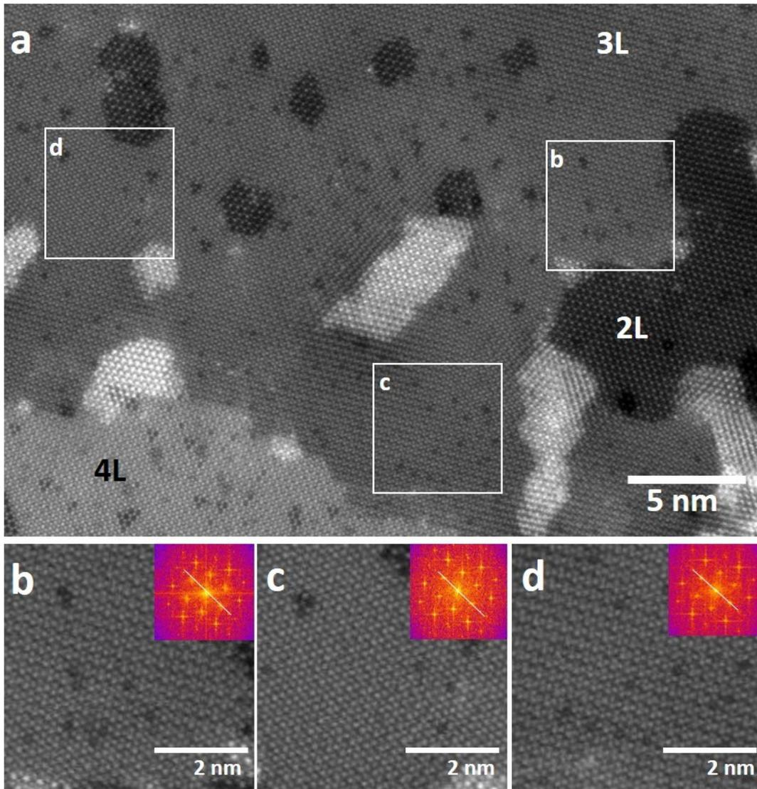
**Figure S7.** (a) ADF-STEM image showing the trilayer WS<sub>2</sub> with the quadralayer and bilayer. (b,c,d) Magnified images of the white boxes in (a). The insets indicate clear main hexagonal spots which means its layer has periodic stacking order without rotations between each layers.
