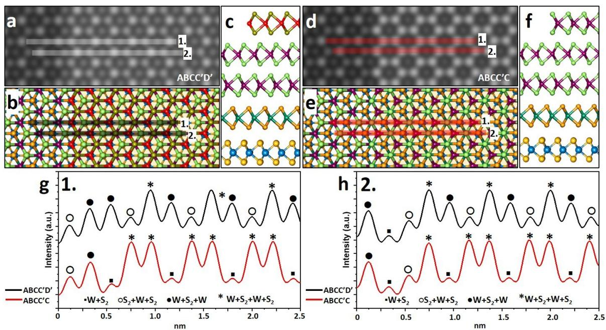
**Figure S11.** Comparison between ABCC'D' stacked and ABCC'C stacked pentalayers using multislice image simulations (a, d) corresponding to atomic models (b, e) and intensity line profiles (g, h), respectively.
