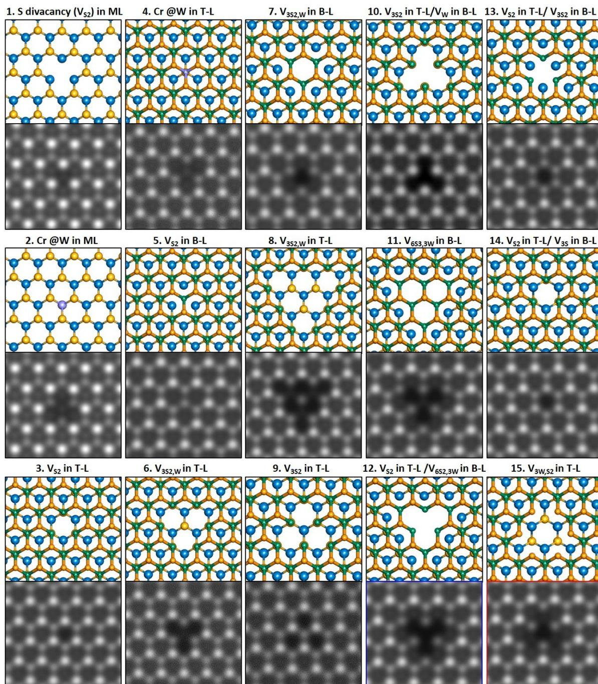
**Figure S2.** Atomic models and multislice ADF-STEM image simulations corresponding to the all atomic models showing the existing type of pores in AB (AB-1) stacked bilayer  $WS_2$ . Yellow and blue spheres indicate S atoms and W atoms in bottom-layer (B-L) and Orange and green spheres indicate S atoms and W atoms in top-layer (T-L) in the atomic models.
