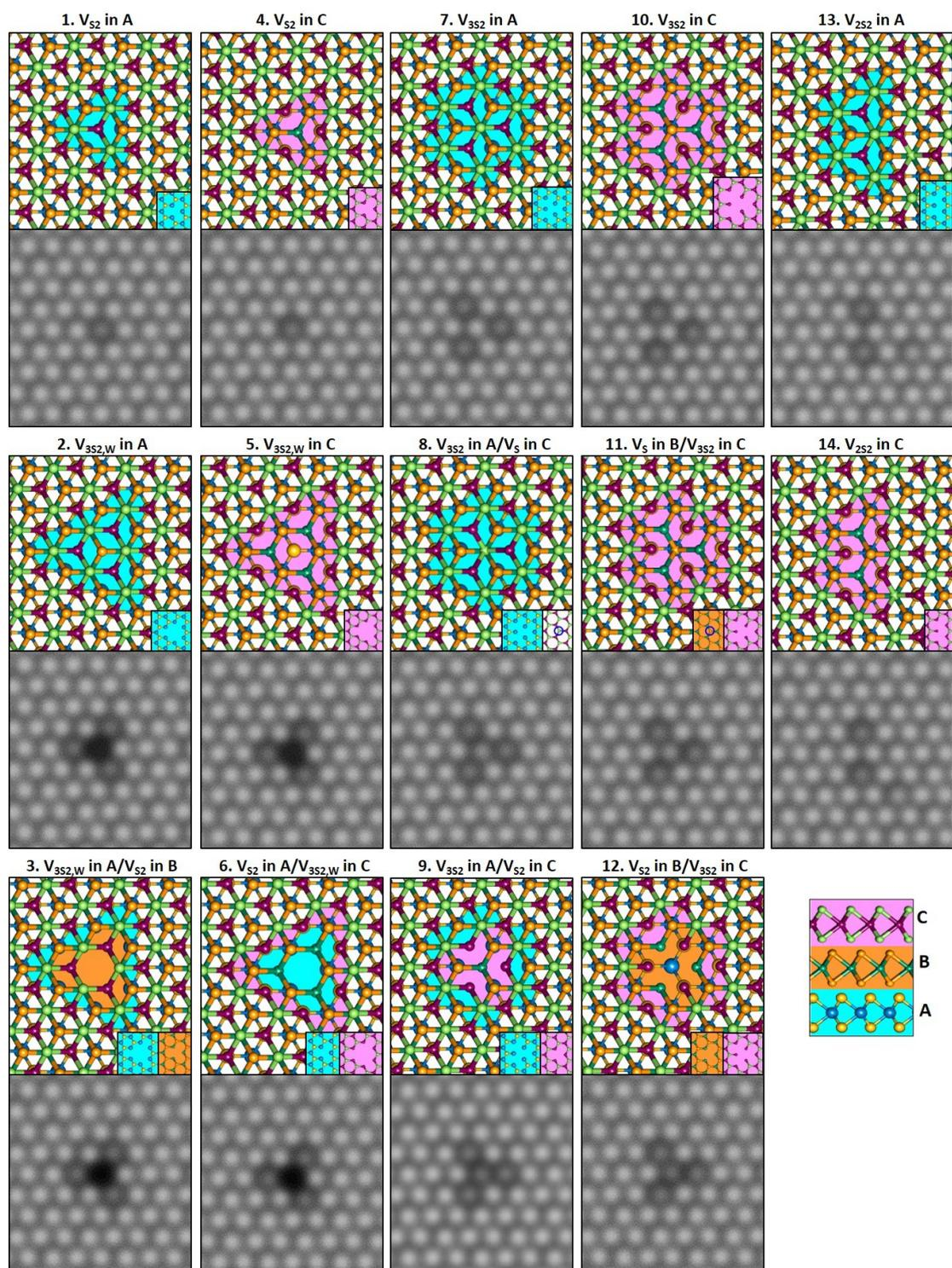
**Figure S4.** Atomic models and multislice ADF-STEM image simulations corresponding to the
