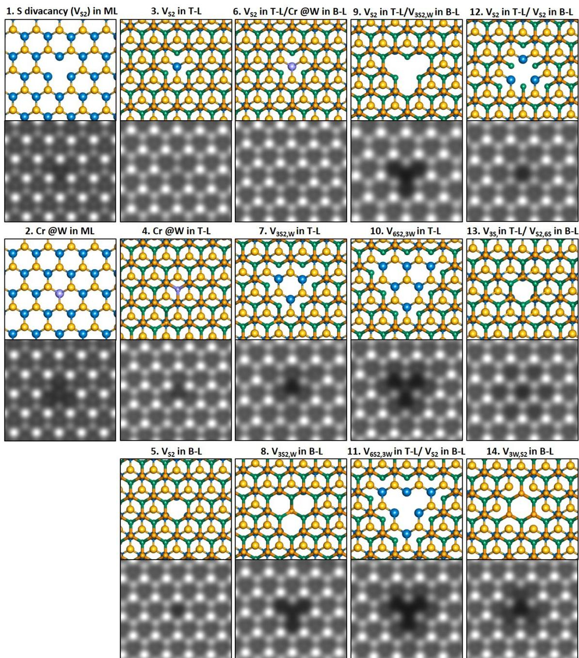
**Figure S3.** Atomic models and multislice ADF-STEM image simulations corresponding to the all atomic models showing the existing type of pores in AB (AB-2) stacked bilayer  $WS_2$ . Yellow and blue spheres indicate S atoms and W atoms in bottom-layer (B-L) and Orange and green spheres indicate S atoms and W atoms in top-layer (T-L) in the atomic models.
