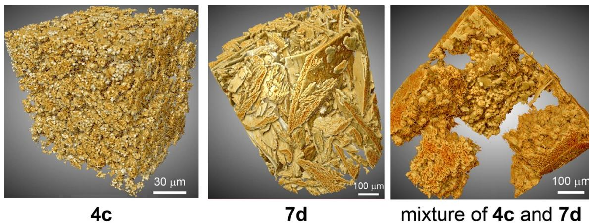
**Fig. S9** 3D rendered X-ray tomography images of individual and mixture of nucleolipids. For clarity, Fig. 6, column 3 has been depicted here in a larger size.
