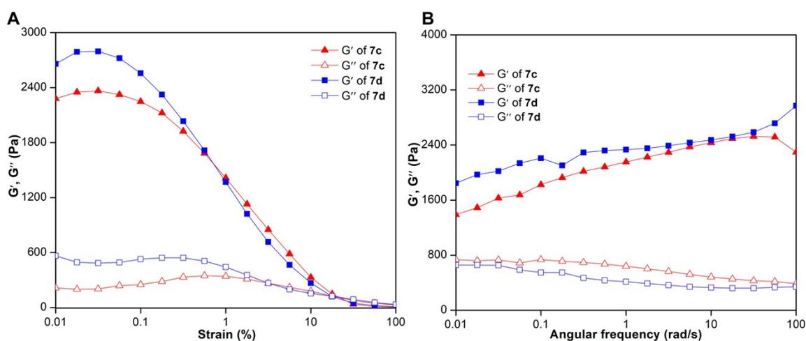
**Fig. S2 (A)** Strain sweep at constant oscillating frequency (10 Hz) plot for uridine nucleolipid gels **7c** (1.2 w/v %) and **7d** (0.7 w/v %) formed in DMSO at respective CGC. **(B)** Frequency sweep at constant strain (0.1 %) plot for the same.
