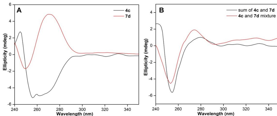
**Fig. S11** (A) CD spectrum of **4c** and **7d** in DMSO (0.5 mM). (B) CD spectrum of a 1:1 mixture of **4c** and **7d** and sum of the CD spectra of individual assemblies of **4c** and **7d**. Spectra were collected from 350 to 240 nm on a Jasco J-815 CD spectrometer using 1 nm bandwidth at 25°C. Experiments were performed in duplicate wherein each spectrum was an average of three scans. The spectrum of DMSO without nucleolipid was subtracted from all the sample spectra.
