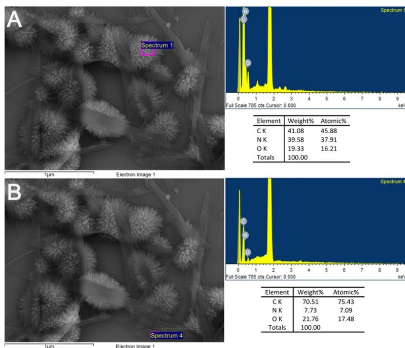
**Fig. S13** EDAX analysis of SEM images obtained from a mixture of uridine nucleolipid **7d** and adenosine. (A) Spectrum 1 (top) shows the elemental composition of the cluster. (B) Spectrum 4 (bottom) elemental composition of the sheet. The compositions were similar for different clusters and sheets, respectively. A comparison of carbon content suggests that the cluster is composed of adenosine and sheets are made of uridine nucleolipid **7d**.
