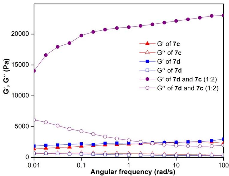
**Fig. S17** Comparison of frequency sweep rheological measurement of nucleolipid gel **7c** (1.2 w/v %), **7d** (0.7 w/v %) and gel formed by a 1:2 mixture of **7d** (9.7 mM) and **7c** (19.4 mM) at constant strain (0.1%).
