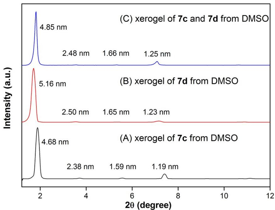
**Fig. S16** Comparison of PXRD spectrum of xerogels of **7c** (A), **7d** (B) and 1:1 mixture of **7c** and **7d** (C). Layer spacing (nm) for diffraction peaks is given.
