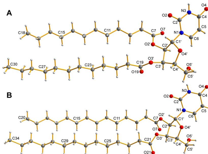
**Fig. S3** X-ray crystal structure of nucleolipid **7b** (A) and **7c** (B) showing one molecule in the unit cell. Nucleobase adopts an *anti* conformation relative to the sugar ring with C2'-endo sugar pucker. Atoms are coded as follows: off white, hydrogen; dark gray, carbon; blue, nitrogen; red, oxygen.
