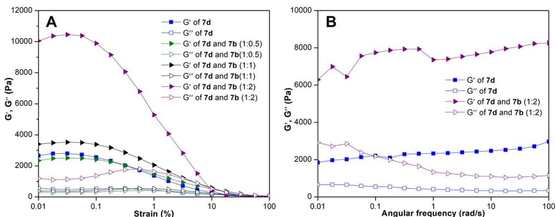
**Fig. S19** Rheological measurement of nucleolipid gels. (A) Comparison of strain sweep of nucleolipid gel 7d (0.7 w/v %) and gels formed by different mixtures of 7d and 7b at constant oscillating frequency. (B) Frequency sweep at constant strain (0.1 %) plot for nucleolipid gel 7d (0.7 w/v %) and gels formed by 1:2 mixture of 7d (9.7 mM) and 7b (19.4 mM).
