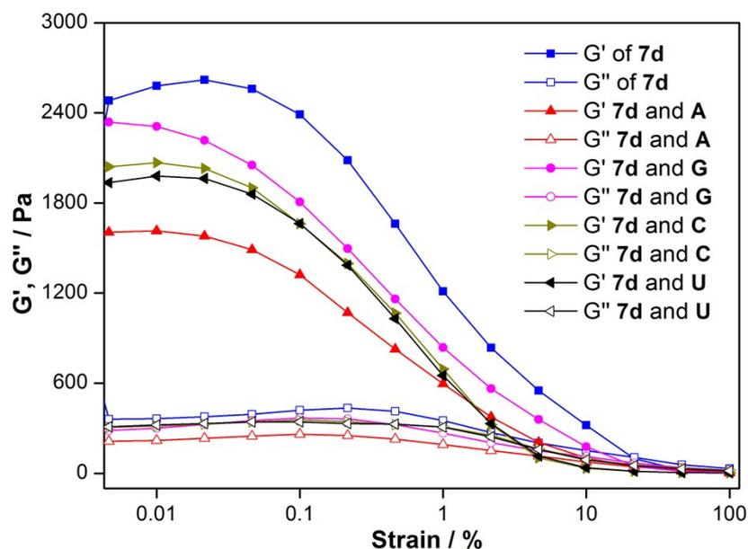
**Fig. S12** Comparison of strain sweep rheological measurement of a 1:1 mixture of uridine nucleolipid gel **7d** in DMSO (0.7 w/v %, CGC) and nucleosides (A = adenosine, G = guanosine, C = cytidine and U = uridine) at constant oscillating frequency.
