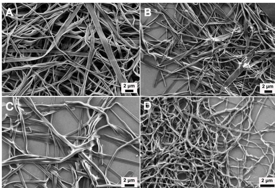
**Fig. S15** FESEM images of xerogels of (A) uridine nucleolipid gel **7d** (0.7 w/v %, CGC) and a mixture of (B) **7d** and guanosine (equiv. 1:1), (C) **7d** and cytidine (equiv. 1:1), (D) **7d** and uridine (equiv. 1:1) in DMSO.
