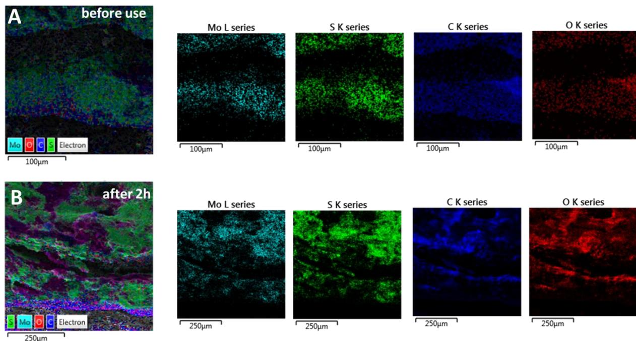
**Figure S10.** Layered images of SEM micrograph and mapping of elements C, O, Mo and S of the external perimeter of the MoS<sub>2</sub>@3D before being used (A) and after being applied to hydrogen evolution reaction for 2 hour at a potential of -500 mV (B).
