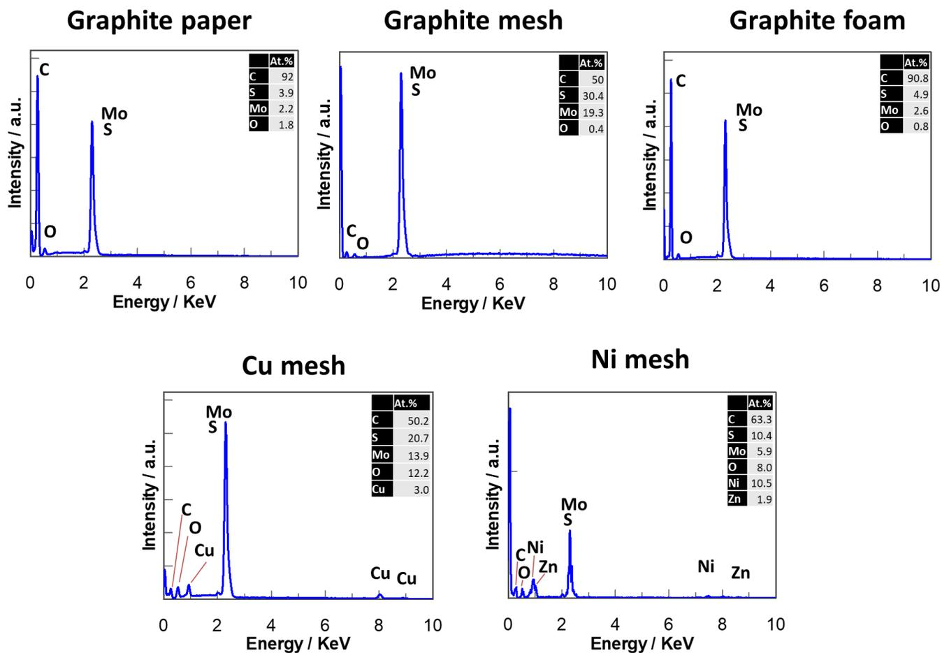
**Figure S7.** EDX spectra different surfaces modified by spray coating using commercial MoS<sub>2</sub> acquired from areas shown in Figure S5.
