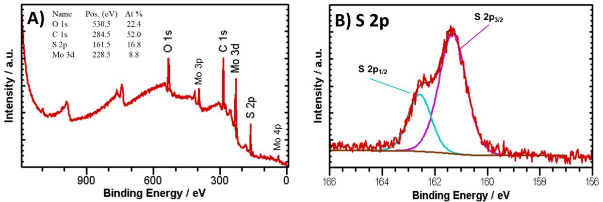
**Figure S3.** Wide XPS spectrum of dried MoS<sub>2</sub> from commercial spray (A) and high resolution S 2p core level with peak deconvolution (B).
