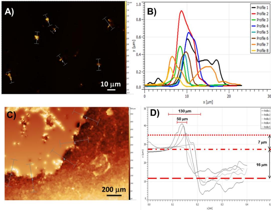
**Figure S2.** Topographical image MoS<sub>2</sub> in ITO acquired by optical profilometer (A), with respective height profiles for measurement of sheet thickness (B). Topographical image of an SPE sprayed with commercial MoS<sub>2</sub> with the 1.5 μm diameter mask acquired by optical profilometer (C), with respective height profiles for measurement of the MoS<sub>2</sub> layer thickness (D).
