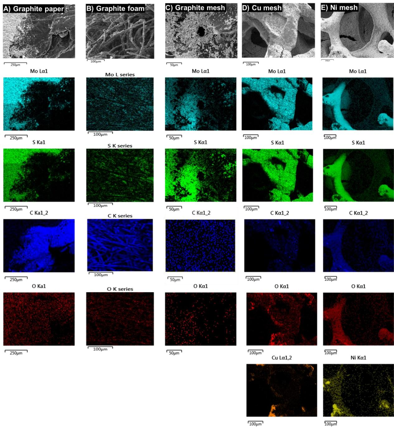
**Figure S6.** SEM micrographs of different surfaces modified by spray coating using commercial MoS<sub>2</sub> with respective mapping of elements: A) Graphite paper, B) Graphite foam, C) Graphite mesh, D) Cu mesh and E) Ni mesh.
