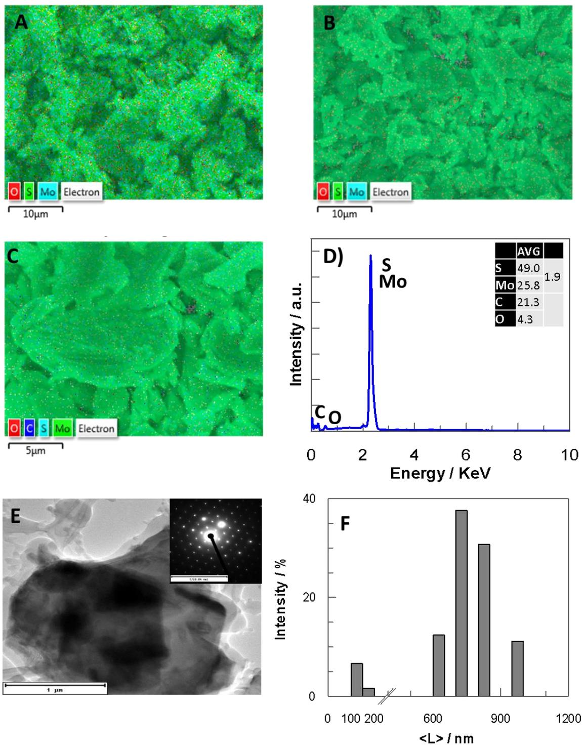
**Figure S1.** SEM micrographs (A-C) of MoS<sub>2</sub> dried films overlaid with mapping of C, O, S and Mo elements. D) Average EDX spectrum of MoS<sub>2</sub> sheets. E) TEM image of MoS<sub>2</sub> sheets. Inset: SEAD. F) Particle lateral size distribution measured by DLS from MoS<sub>2</sub> sheet suspended in DMF.
