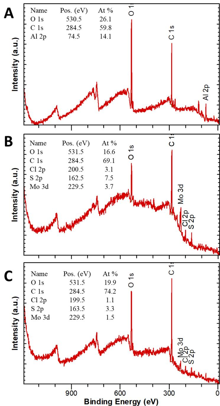
**Figure S5.** Wide XPS spectrum of bare SPE (A), spray coated MoS<sub>2</sub> SPE before (B) and after (C) being used in hydrogen evolution reaction in both acidic and alkali conditions. Inset includes information on the core levels, peak position (eV) and atomic percentage for each sample.
