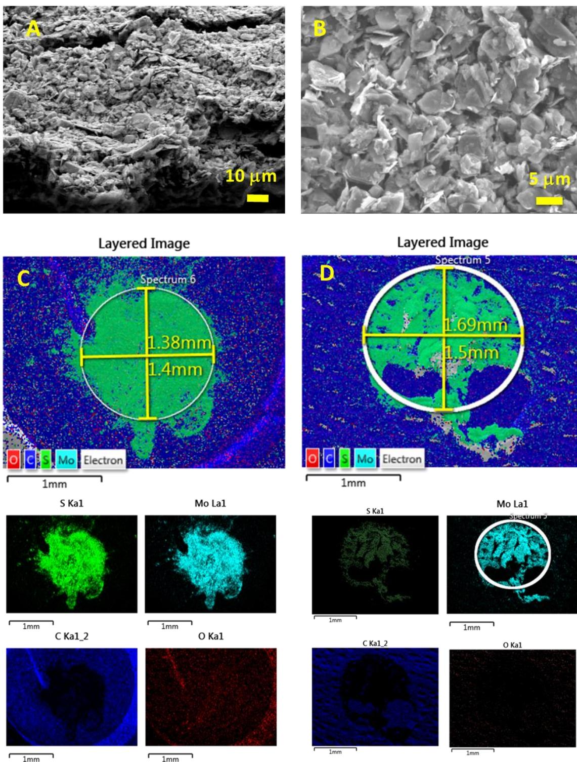
**Figure S4.** SEM micrographs at different magnifications of SPE modified by spray coating using commercial MoS<sub>2</sub> (A and B). Layered images of SEM micrograph and mapping of elements C, O, Mo and S of MoS<sub>2</sub> modified SPEs (C and D).
