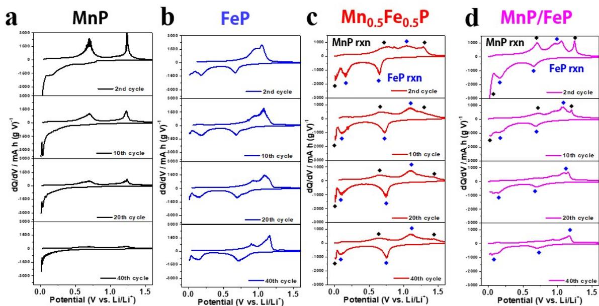
**Fig. S8** DCPs for MnP, FeP,  $\text{Mn}_{0.5}\text{Fe}_{0.5}\text{P}$ , and MnP/FeP electrodes for 2<sup>nd</sup>, 10<sup>th</sup>, 20<sup>th</sup>, and 40<sup>th</sup> cycles at the current density of 100 mA g<sup>-1</sup>.
