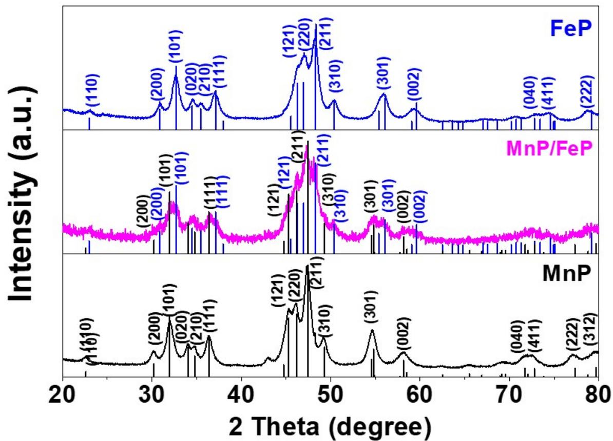
**Fig. S2** XRD patterns of as-synthesized MnP, MnP/FeP mixture, and FeP NPs. The reference peaks for MnP (ICDD # 00-051-0942, black color) and FeP (ICDD # 01-078-1443, blue color) are included.
