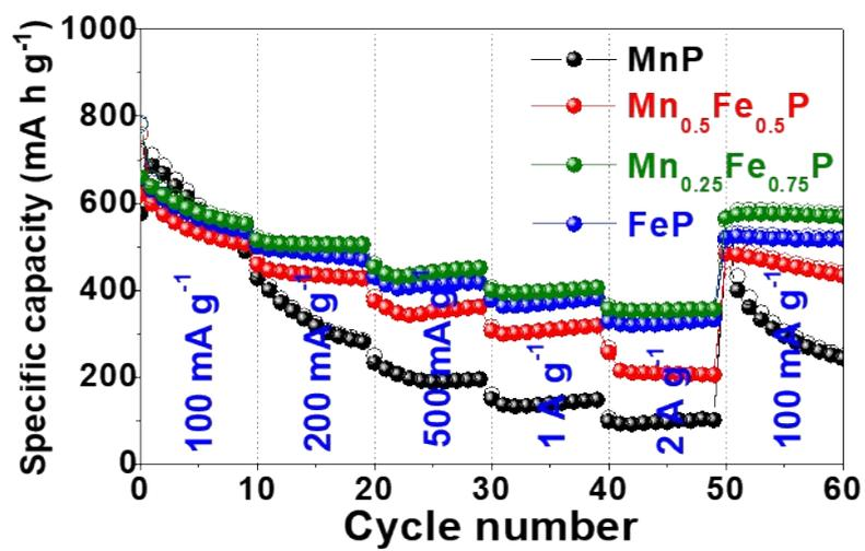
**Fig. S9** (a) Rate capabilities of the  $\text{Mn}_{1-x}\text{Fe}_x\text{P}$  ( $x = 0, 0.5, 0.75, \text{ and } 1$ ) electrodes.
