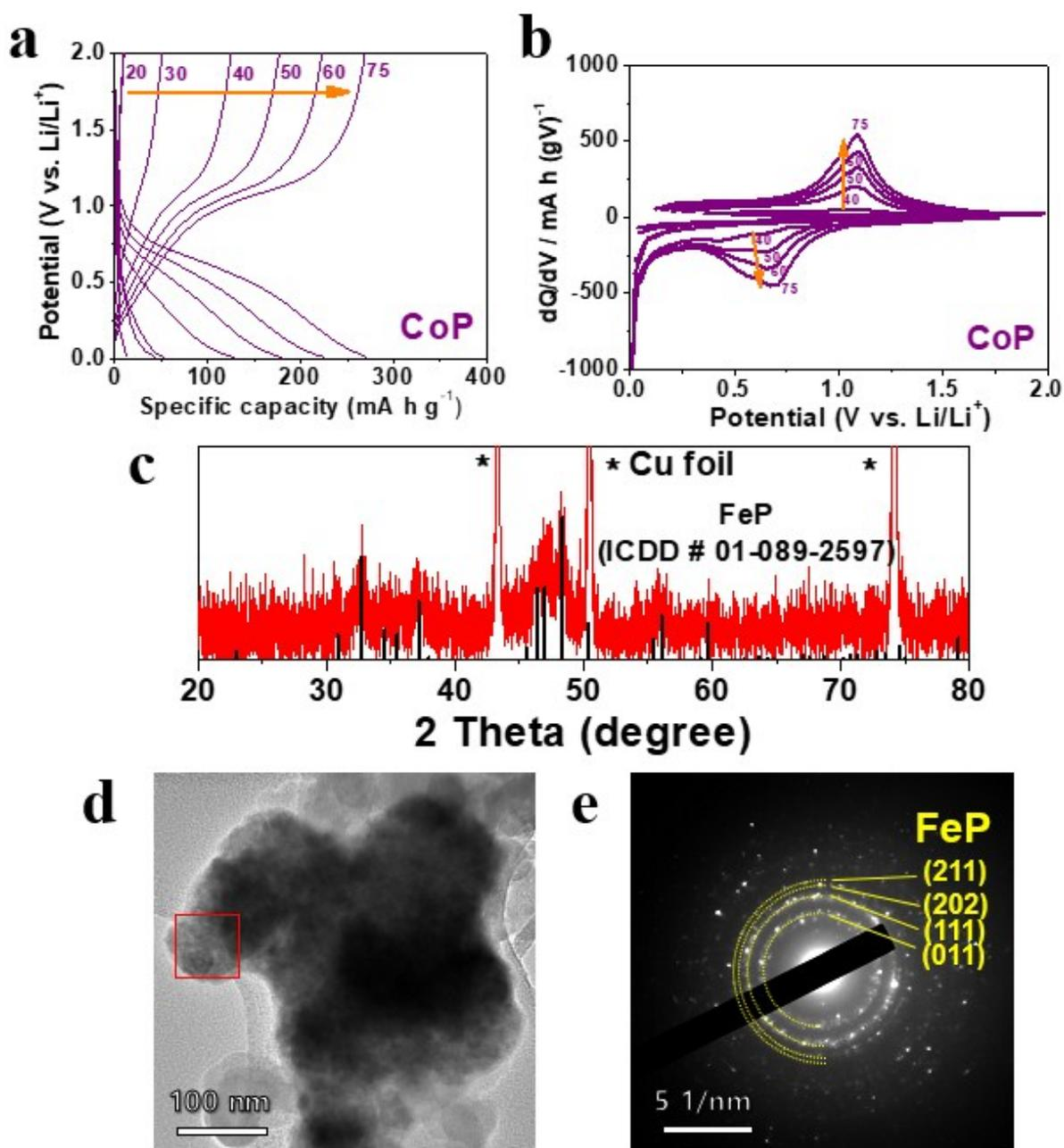
**Fig. S12** (a) Galvanostatic voltage profiles and (b) corresponding differential capacity plots (DCPs) of CoP electrode at 2 A g<sup>-1</sup> and (c) XRD pattern, (d) TEM image, and (e) SAED pattern of FeP electrode for 1<sup>st</sup> fully discharged state at 2 A g<sup>-1</sup>.
