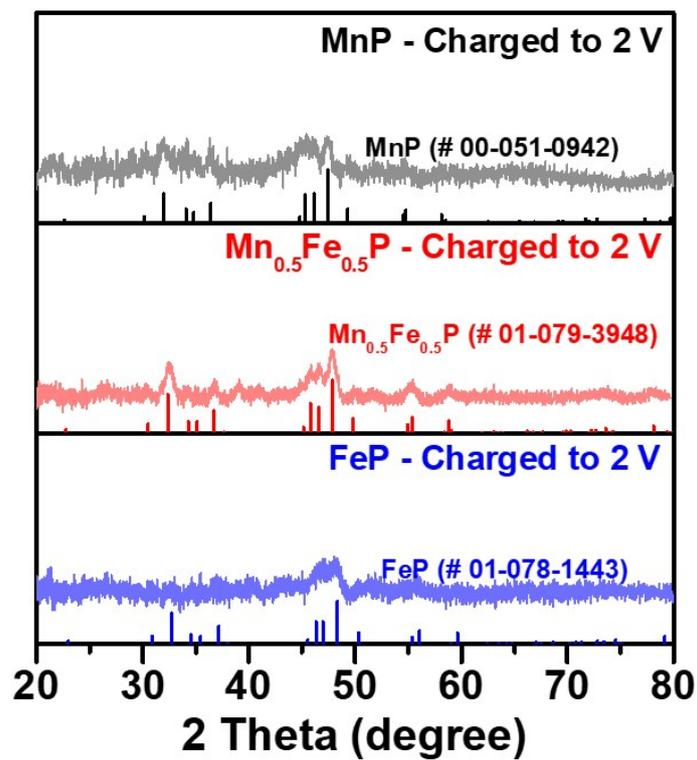
**Fig. S6** *Ex-situ* XRD patterns of 1<sup>st</sup> fully charged states for Mn<sub>1-x</sub>Fe<sub>x</sub>P (x = 0, 0.5, and 1.0) electrodes. The reference peaks for MnP (ICDD # 00-051-0942, black color), Mn<sub>0.5</sub>Fe<sub>0.5</sub>P (ICDD # 01-079-3948, red color), and FeP (ICDD # 01-078-1443, blue color) are included.
