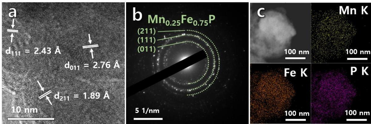
**Fig. S3** (a) HRTEM image, (b) SAED pattern, and (c) STEM and EDS element mapping images (Mn K, Fe K, and P K) of as-prepared  $\text{Mn}_{1-x}\text{Fe}_x\text{P}$  ( $x = 0.75$ ) NPs.
