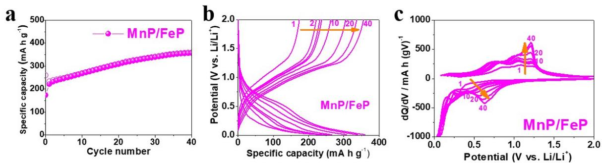
**Fig. S13** (a) Cycling performance of MnP/FeP electrode at 2 A g<sup>-1</sup> and corresponding (b) galvanostatic voltage profiles and (c) differential capacity plots (DCP).
