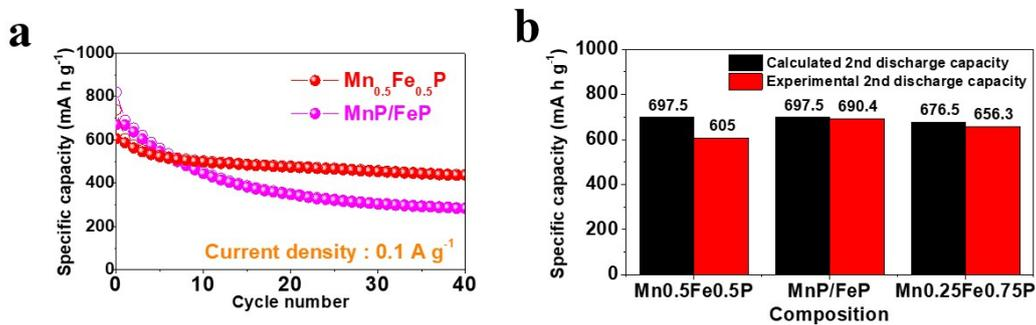
**Fig. S7** (a) Cycle performance of Mn<sub>0.5</sub>Fe<sub>0.5</sub>P solid solution and MnP/FeP mixture electrodes at the current density of 100 mA g<sup>-1</sup> and (b) comparison of experimentally determined and expected 2<sup>nd</sup> discharge capacity in Mn<sub>0.5</sub>Fe<sub>0.5</sub>P and Mn<sub>0.25</sub>Fe<sub>0.75</sub>P solid solution and MnP/FeP mixture electrodes. The expected values were estimated from the reversible capacities of both MnP and FeP electrodes.
