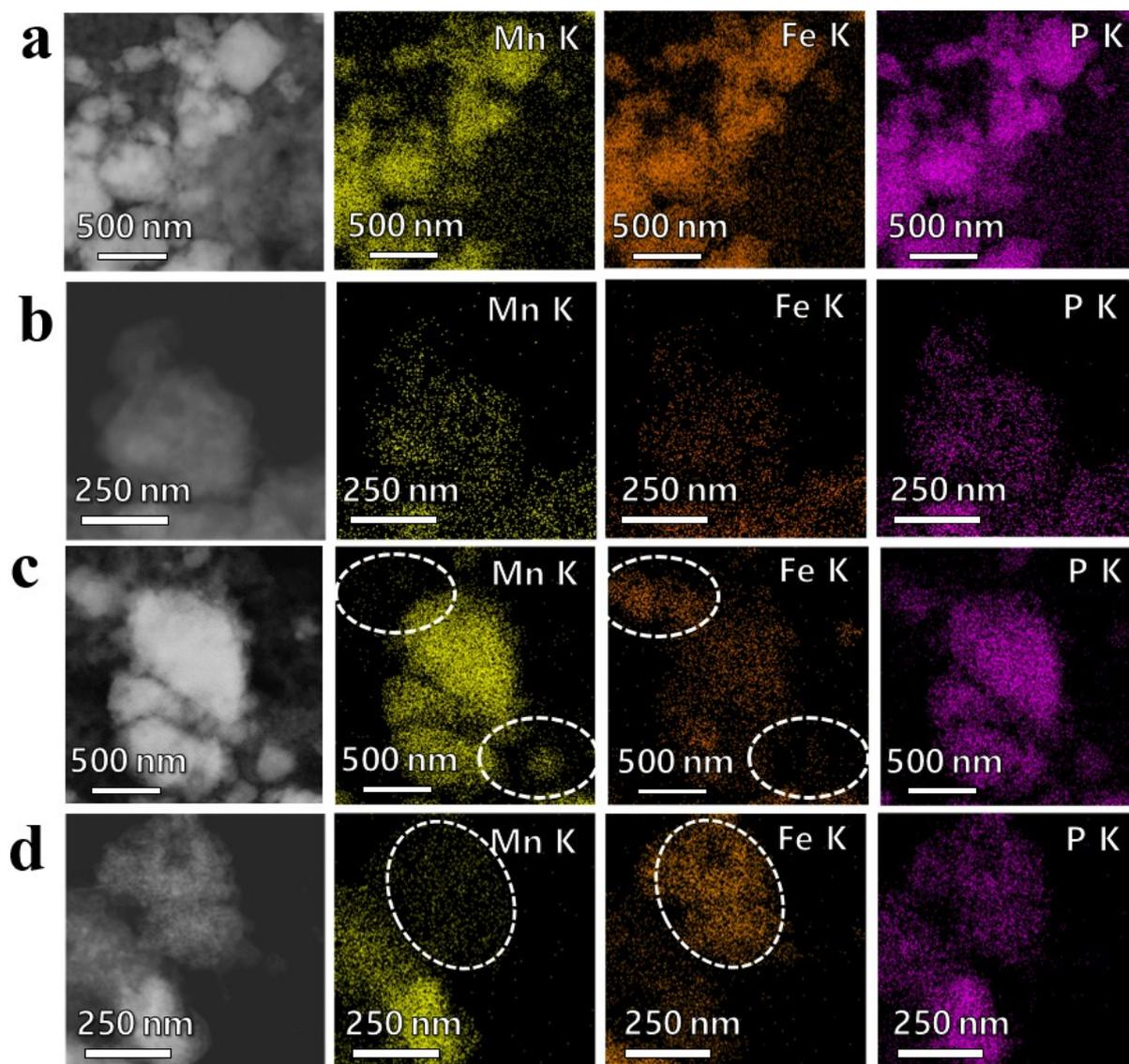
**Fig. S14** STEM images and EDS mapping images (Mn K, Fe K, and P K) of after 1<sup>st</sup> and 100<sup>th</sup> cycled electrodes tested at 2 A g<sup>-1</sup> for (a,b)  $\text{Mn}_{0.5}\text{Fe}_{0.5}\text{P}$  and (c,d) MnP/FeP electrodes.
