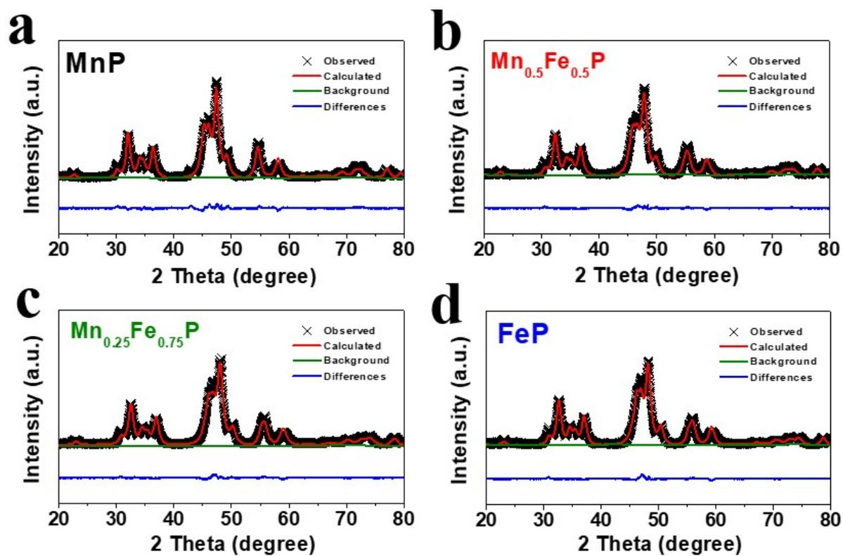
**Fig. S1** XRD Rietveld refinement results for as-synthesized  $\text{Mn}_{1-x}\text{Fe}_x\text{P}$  (x = 0, 0.5, 0.75, and 1.0) NPs.
