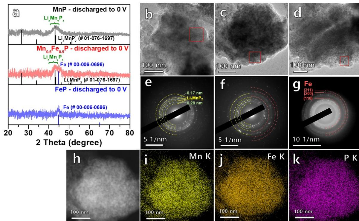
**Fig. S5** (a) *Ex-situ* XRD patterns, TEM images, and SAED patterns of fully discharged states of (b,e) MnP, (c,f) Mn<sub>0.5</sub>Fe<sub>0.5</sub>P, and (d,g) FeP electrodes, and (h) STEM image and (i-k) EDS mapping (Mn K, Fe K, and P K) of (c) Mn<sub>0.5</sub>Fe<sub>0.5</sub>P electrode.
