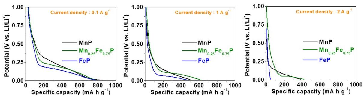
**Fig. S11** Galvanostatic discharge voltage profiles of Mn<sub>1-x</sub>Fe<sub>x</sub>P (x = 0, 0.75, and 1) electrodes for 1<sup>st</sup> cycle at 0.1, 1.0, and 2.0 A g<sup>-1</sup>, respectively.
