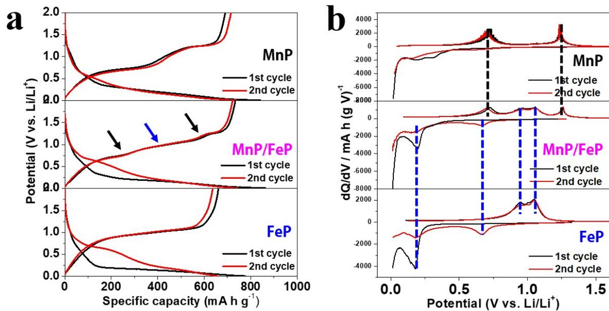
**Fig. S4** (a) Galvanostatic discharge/charge profiles and (b) corresponding differential capacity plots (DCPs) of MnP, MnP/FeP mixture, and FeP electrodes.
