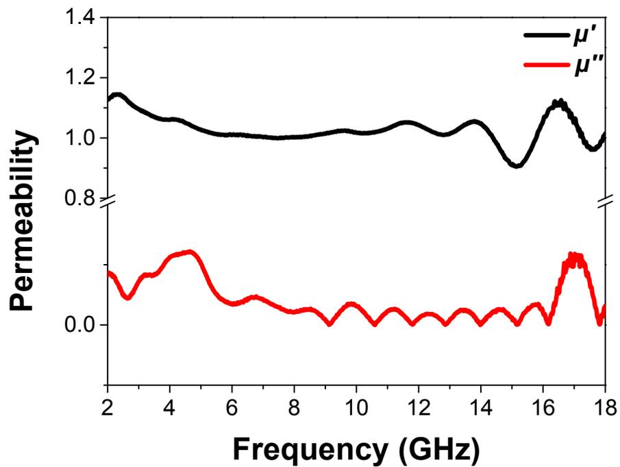
Fig S4. Permeability of TSPG film in the frequency range of 2-18 GHz.
