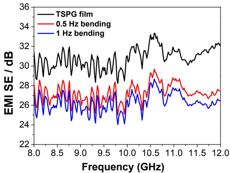
**Fig S2.** EMI shielding effectiveness of a TSPG film before and after repeatedly bending to a radius of 2.5 mm 500 cycles.
