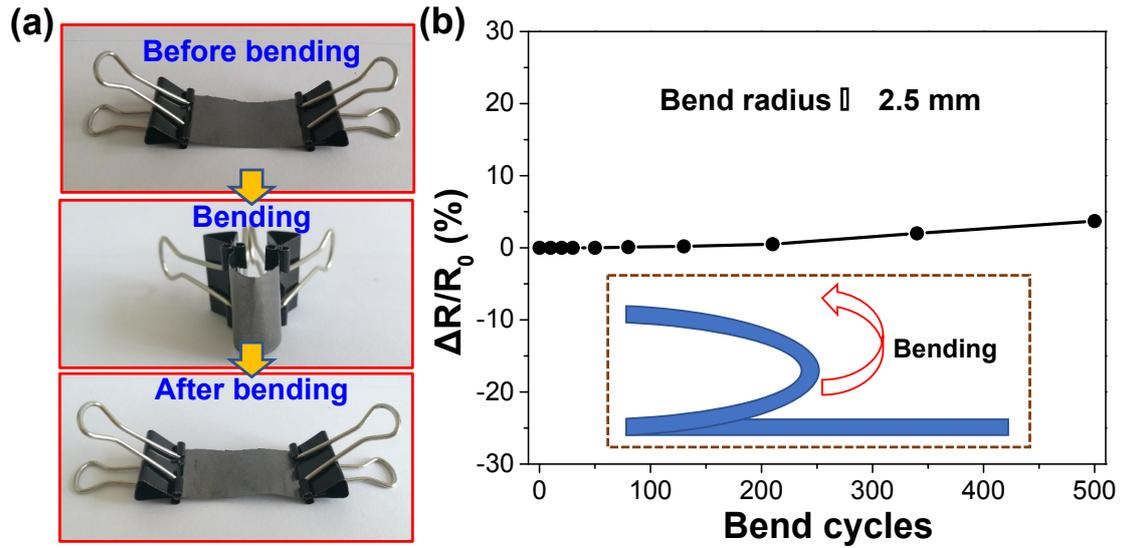
**Fig S1.** (a) A schematic for the bending process of the film (bend radius  $<$  2.5 mm, 500 times). (b) Resistance change of the TSPG film under a repeatedly bending process.
