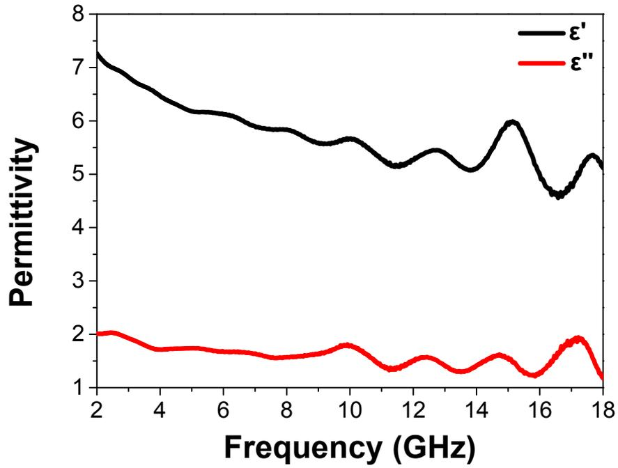
Fig S3. Permittivity of TSPG film in the frequency range of 2-18 GHz.
