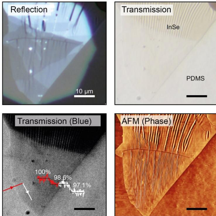
**Figure S5.** Optical pictures of a wrinkled InSe flake deposited onto PDMS in reflection illumination mode (top left) and transmission (top right). Bottom left: intensity of the blue channel of the transmission image. The line with arrows indicate the position of the shown line profiles. Bottom right: AFM phase topology. Notice that the wrinkles (with wavelength  $< 800$  nm) in the thinnest regions, which are visible in the AFM image, could not be observed optically.
