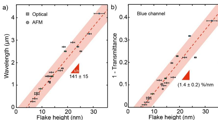
Figure S4. a-b) Wavelength of the wrinkles (a) and optical absorption in the blue channel (b) as a function of the flake height obtained by AFM. The dashed red line is a linear fit to the data and the shaded region represents the 95% confidence bands.
