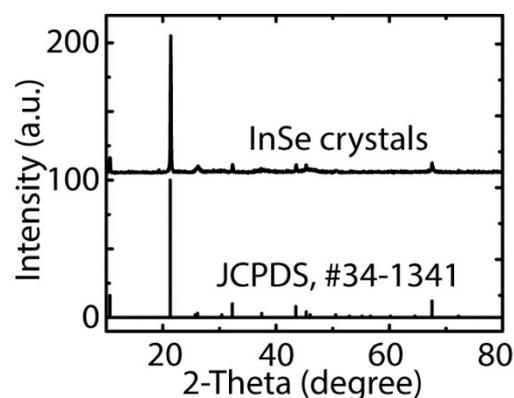
Figure S2: The X-ray diffraction (XRD) characterization of InSe crystals. The comparison between XRD spectrum of InSe crystals indicates a high agreement with the hexagonal InSe phase (JCPDS, card no. 34-1341).
