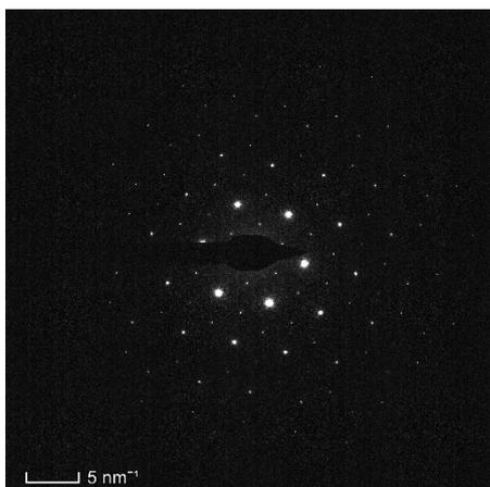
Figure S3: The electron diffraction pattern of InSe crystals by transmission electron microscopy (TEM).
