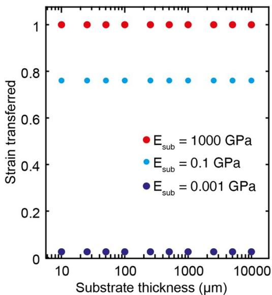
**Figure S8.** Finite element analysis simulation of the strain transferred to a 10 nm thick InSe flake as a function of the thickness of the substrate for different values of the substrate Young's modulus.
