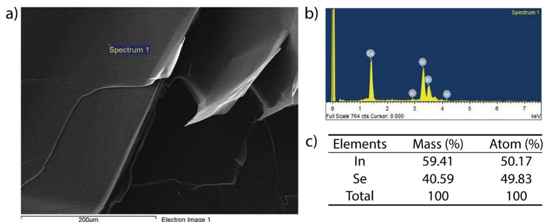
Figure S1: The scanning electron microscopy (SEM) characterization of InSe bulks. a) The surface morphology of mechanical cleavage plane of InSe. b) The energy dispersive spectrum (EDS) of the position marked with Spectrum 1 in panel a. c) The composition of InSe bulks gotten from EDS result. The atomic ratio In:Se  $\approx$  1:1.
