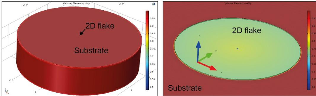
**Figure S7.** Pictures of the final 3D geometry used in COMSOL to simulate the strain transfer from a substrate to a flake deposited on top taken at two different magnifications.
