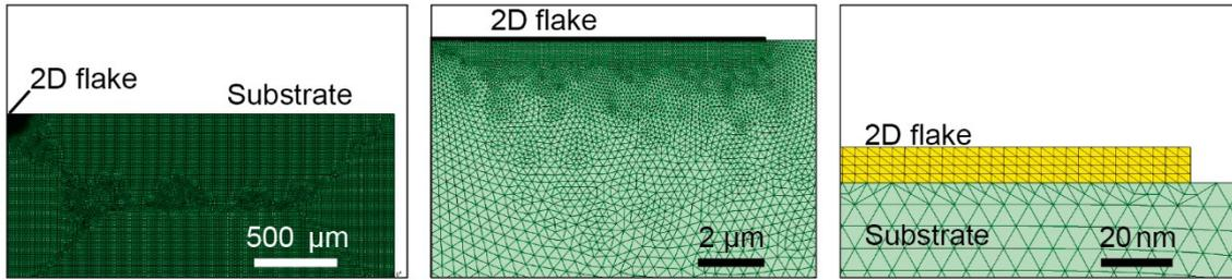
**Figure S6.** Pictures of the axisymmetric geometry used in COMSOL to simulate the strain transfer from a substrate (green) to a flake deposited on top (yellow) taken at different magnifications.
