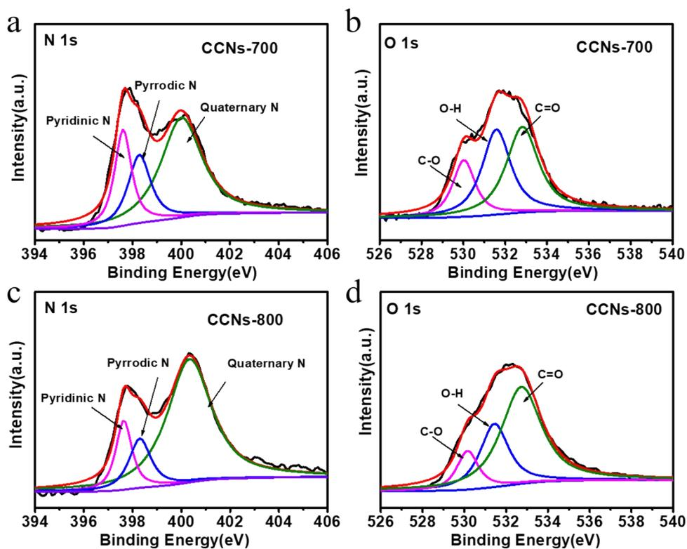
Fig. S10. High resolution of (a, c) N 1s and (b, d) O 1s for CCNs samples.
