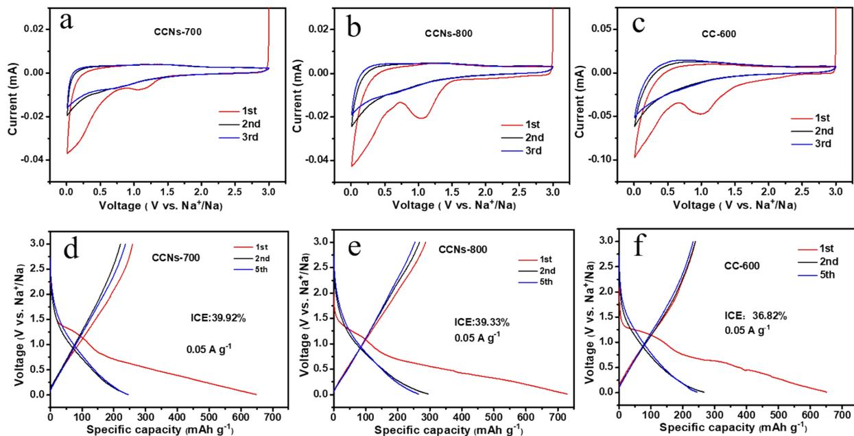
**Fig. S11.** (a, b, c) Typical CV curves at a scan rate of 0.2 mV/s and (d, e, f) galvanostatic charge–discharge curves of CCNs-700, CCNs-800, and CC-600, respectively.
