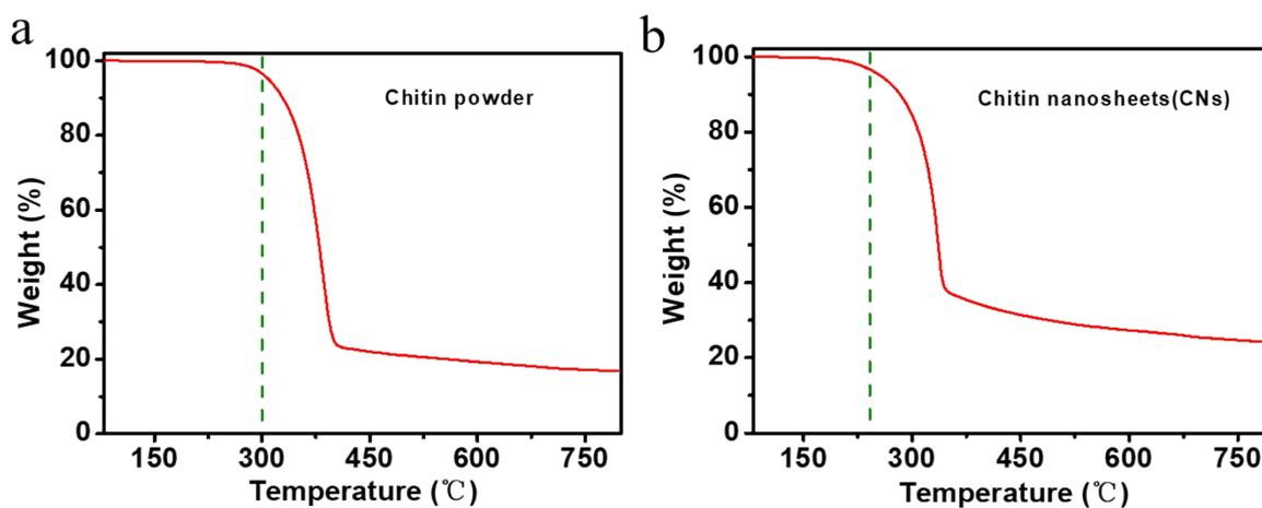
**Fig. S4.** Thermogravimetric analysis (TGA) of (a) chitin powder and (b) chitin nanosheets (CNs) under argon atmosphere.
