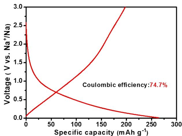
**Fig. S12.** Initial charge and discharge curves of CCNs-600 at current density of 50 mA g<sup>-1</sup> after Pretreatment.
