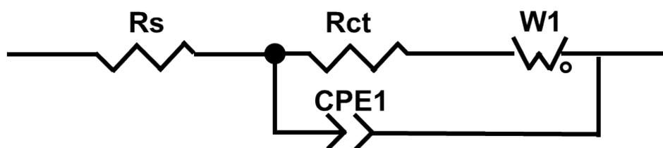
**Schematic S1.** The schematic of Impedance fitting circuit
