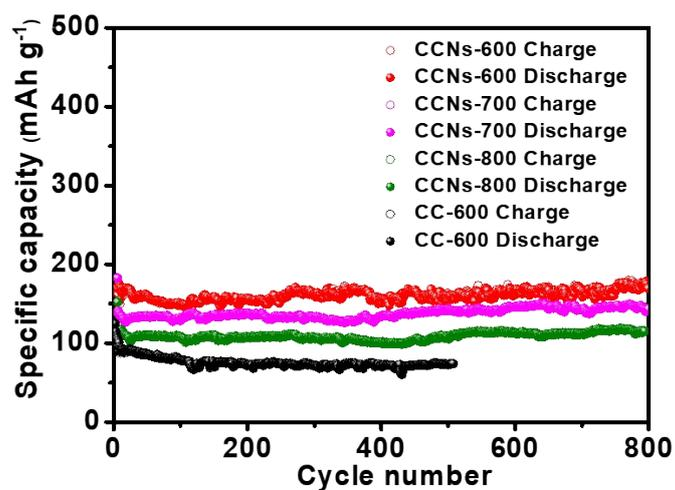
**Fig. S17.** Cycling performance of different CCNs samples at a current density of  $2 \text{ A g}^{-1}$
