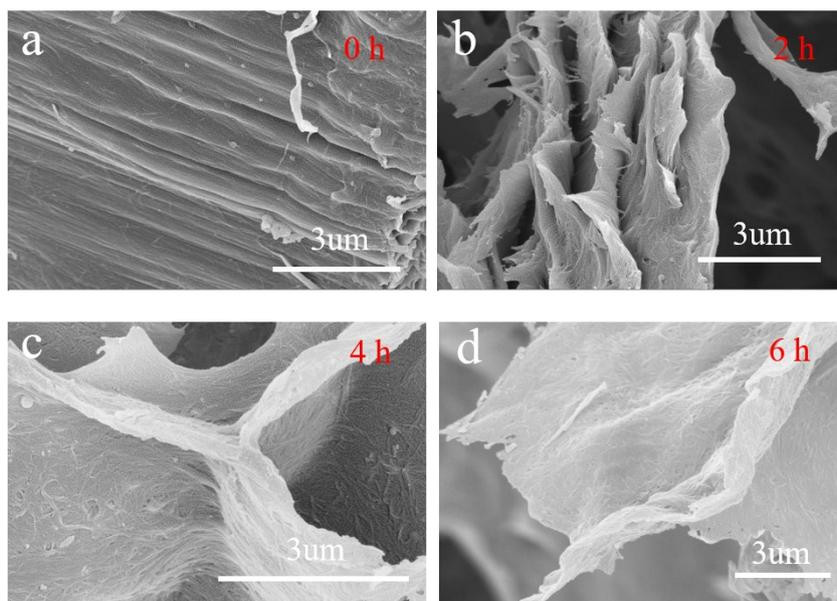
**Fig. S1.** (a-d) Exfoliation process of chitin nanosheets under hydrothermal treatment at different reaction time.
