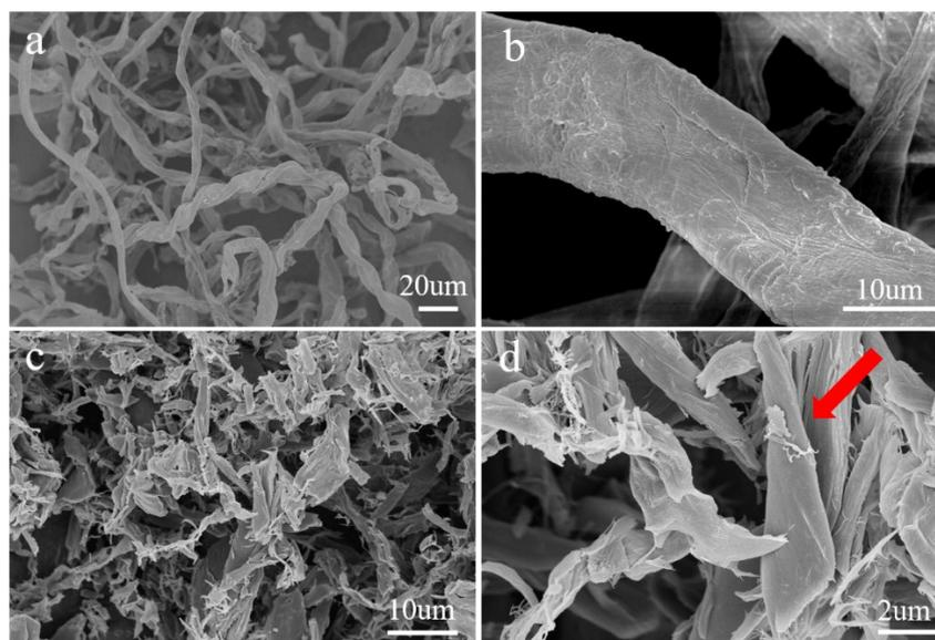
**Fig. S2.** SEM images of cotton linter before (a, b) and after (c, d) hydrothermal treatment.
