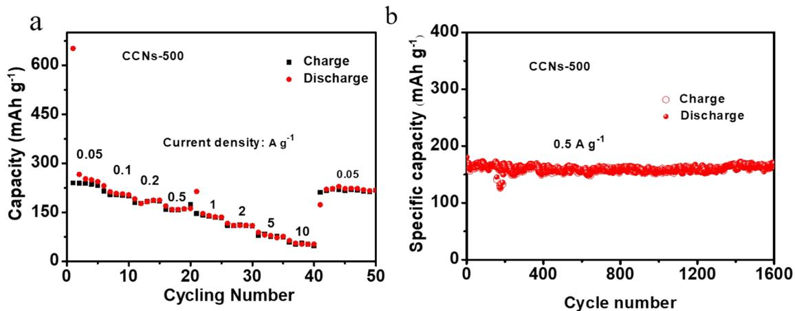
Fig. S14. (a) Rate property and (b) cycling performance of CCNs-500 under 0.5 A g<sup>-1</sup>.
