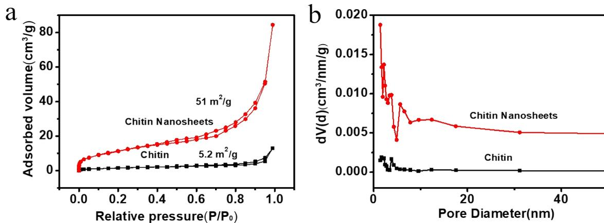
**Fig. S3.** (a) Nitrogen adsorption and desorption isotherms and (b) pore size distributions of chitin and chitin nanosheets.
