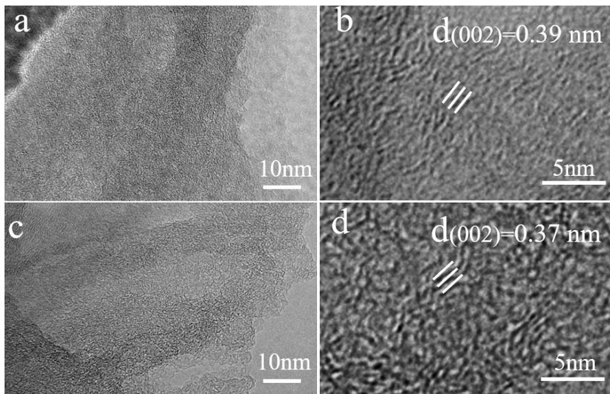
**Fig. S8.** TEM and HRTEM images of (a, b) CCNs-700 and (c, d) CCNs-800.
