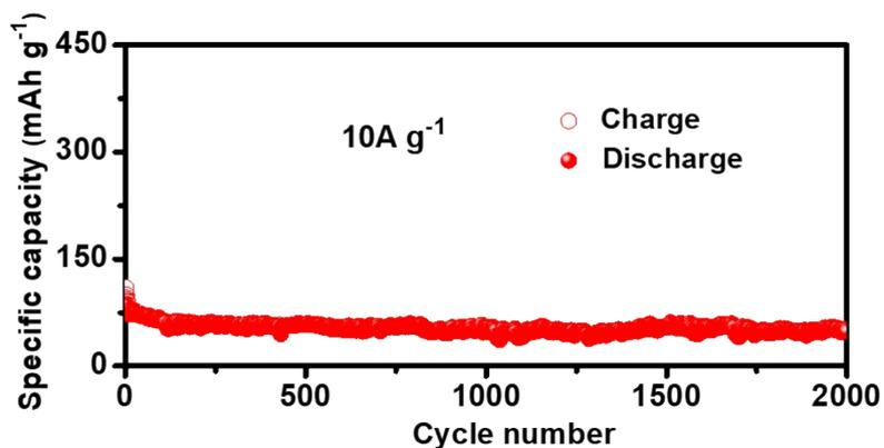
Fig. S16. Cycling performance of different CCNs-600 at a current density of 10 A g<sup>-1</sup>
