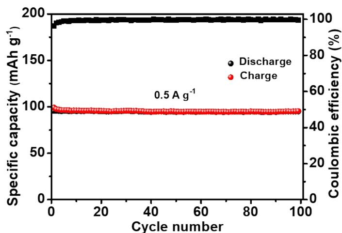
**Fig. S19.** The cycling performance of  $\text{Na}_3\text{V}_2(\text{PO}_4)_3$  cathode at  $0.5 \text{ A g}^{-1}$  with a voltage platform of  $3.4 \text{ V}$ .
