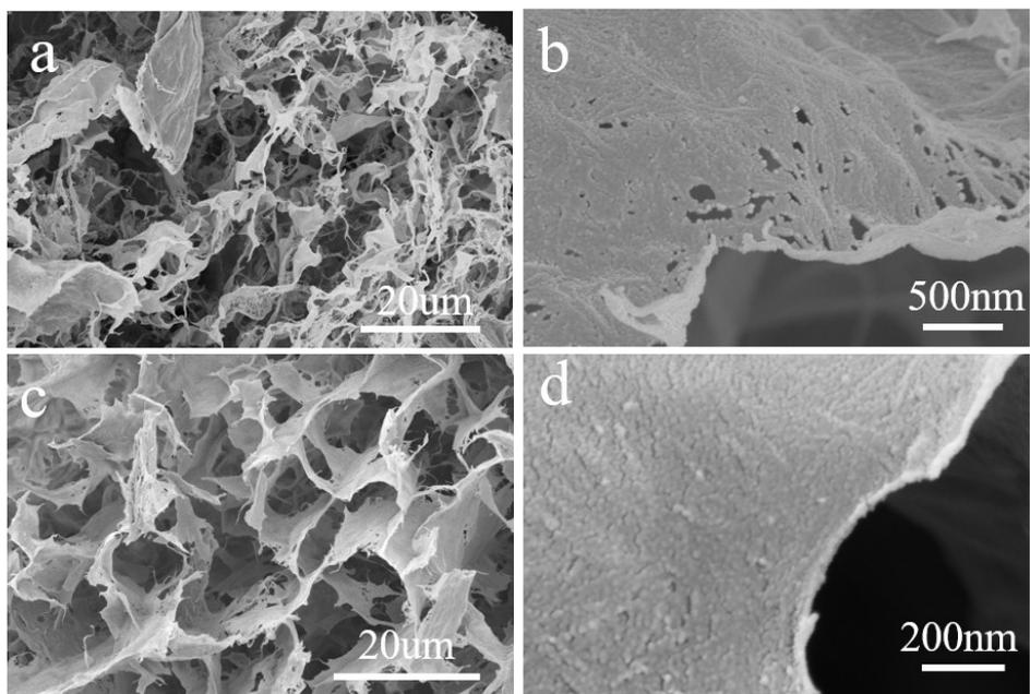
**Fig. S5.** SEM images of (a, b) CCNs-700 and (c, d) CCNs-800.
