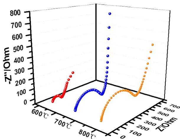
**Fig. S13.** Electrochemical impedance spectra of different CCNs samples with the frequency ranging from 100 KHz to 0.1 Hz.
