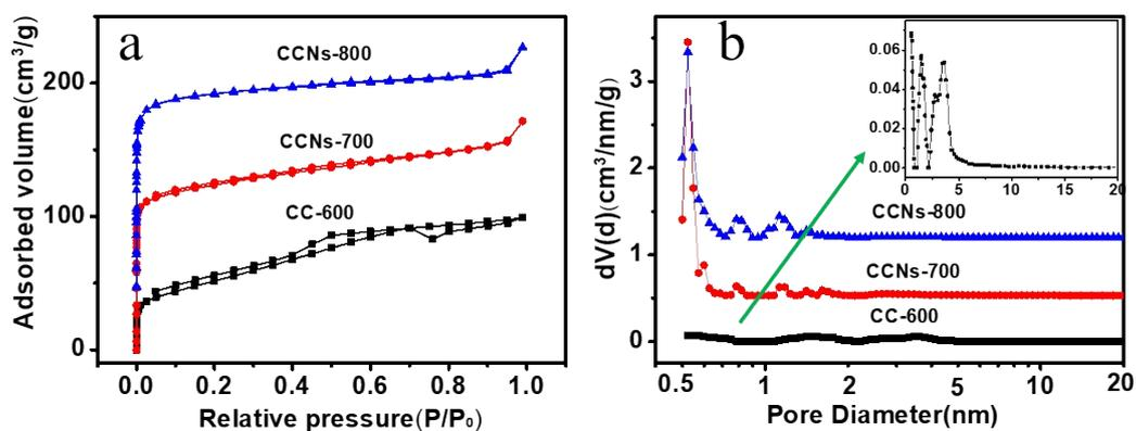
**Fig. S9.** (a) Nitrogen adsorption and desorption isotherms and (b) pore size distributions of CCNs and CC-600 samples.
