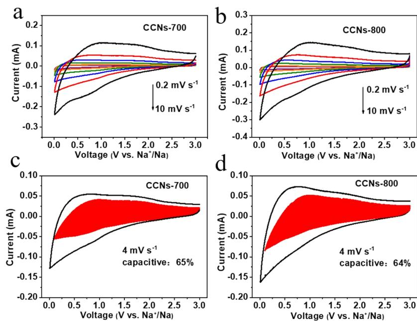
**Fig. S18.** (a, b) CV curves of the different CCNs electrode at various scan rates, (c, d) CV curve of the different electrode at  $4 \text{ mV s}^{-1}$  with the shadowed area representing the surface capacitive contribution.
