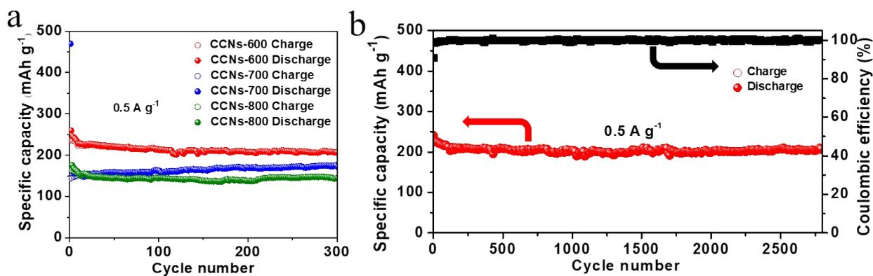
Fig. S15. (a) Cycling performance of different CCNs samples at a current density of 0.5 A g<sup>-1</sup>, (b) cycling performance of CCNs-600 for over 2500 cycles.
