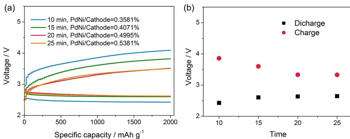
**Figure S4. The influence of PdNi amount of PdNi/NiNF on the battery performance. (a)** The first charge-discharge curves and (b) the corresponding overpotential of Li-O<sub>2</sub> cells with different PdNi/NiNF cathodes.
