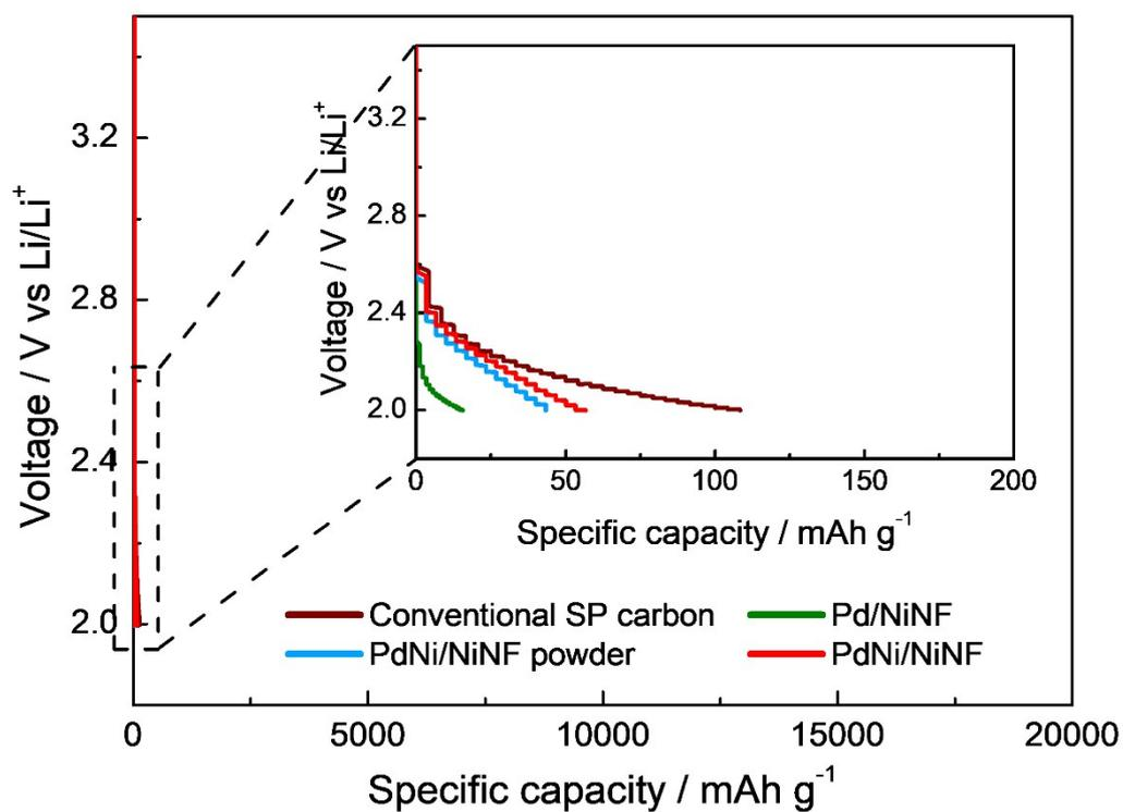
**Figure S9.** The discharge curves of the Ar-filled cells based on the conventional SP carbon, Pd/NiNF, PdNi/NiNF powder and PdNi/NiNF alone electrodes at a current density of 0.10 mA cm<sup>-2</sup>.
