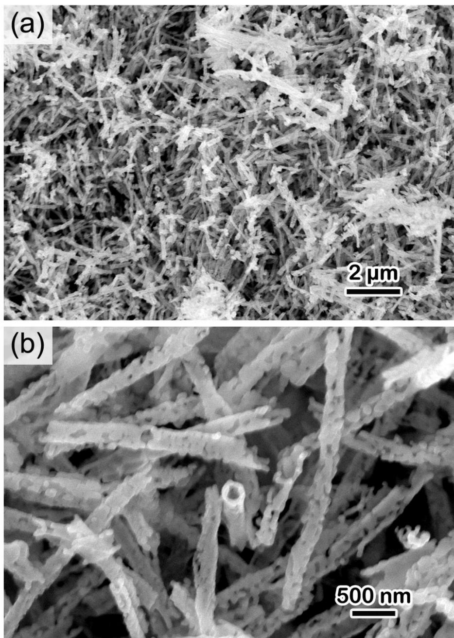
**Figure S7.** (a) Low and (b) high magnification SEM images of the PdNi/NiNF powder cathode.
