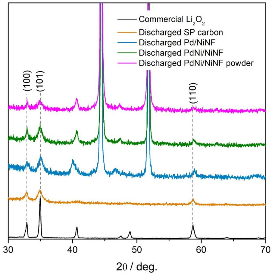
**Figure S8.** PXRD patterns of the discharged cathodes with the conventional SP carbon, Pd/NiNF, PdNi/NiNF, PdNi/NiNF powder after the first discharge.
