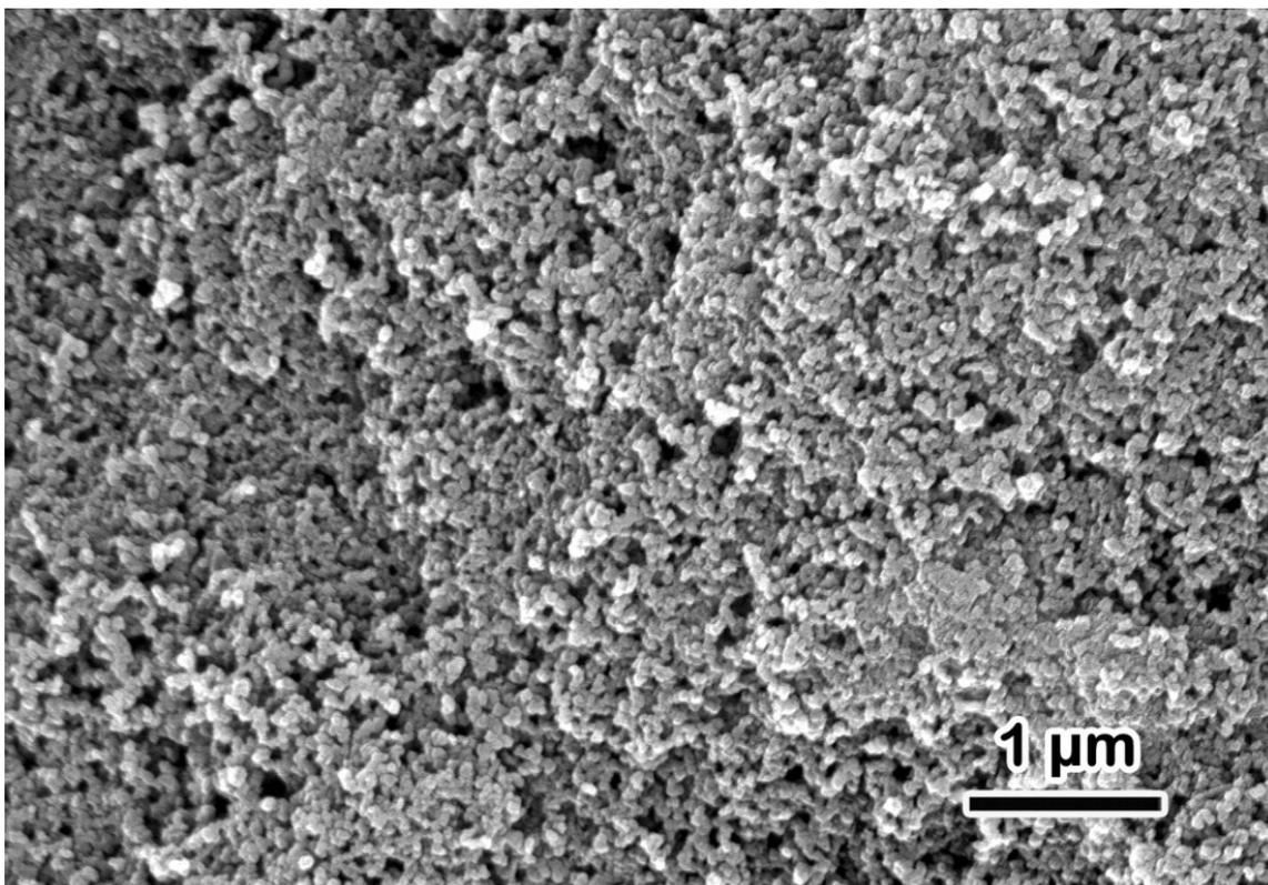
**Figure S6.** FESEM image of the conventional SP carbon cathode.
