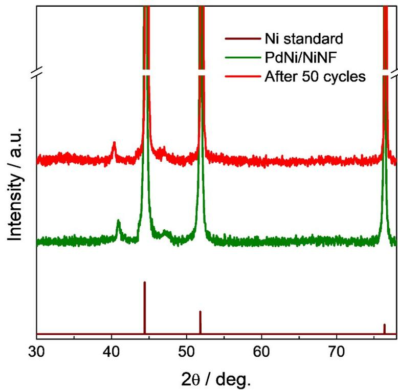
**Figure S11.** PXRD patterns of the discharged PdNi/NiNF cathode before and after 50 cycles.
