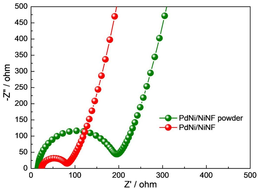
**Figure S5.** Electrochemical impedance spectra (EIS) of PdNi/NiNF and PdNi/NiNF powder cathodes.
