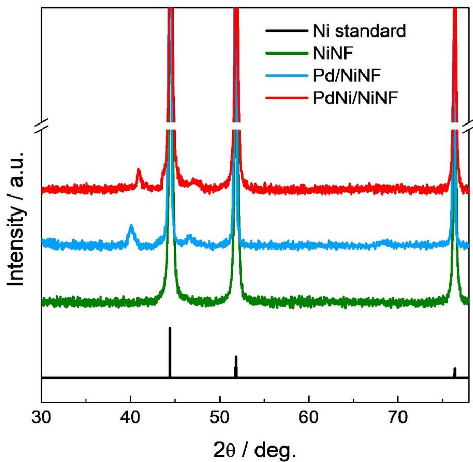
**Figure S2.** Powder X-ray diffraction patterns of Ni NF, Pd/NiNF and PdNi/NiNF cathodes.
