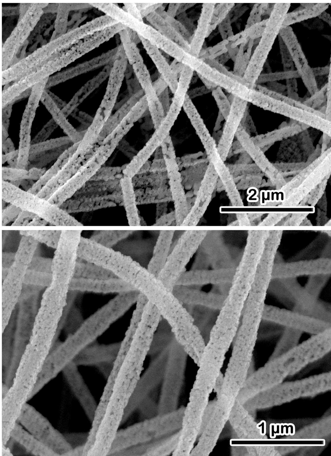
**Figure S1.** The field emission scanning electron microscopic (FESEM) image of Pd/NiNF.
