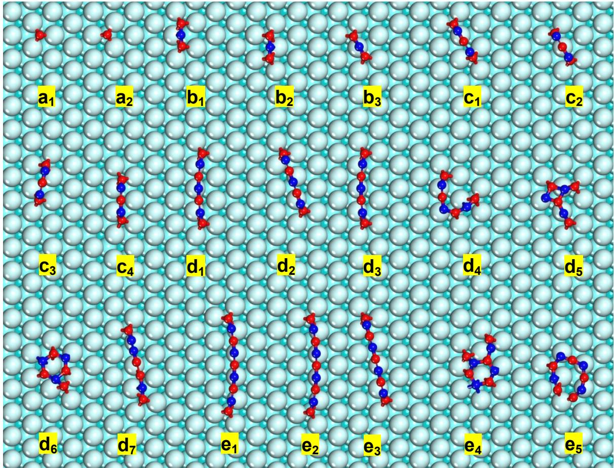
**Fig. S7** Structures and formation energies of small  $B_nN_{n-1}$  ( $1 \leq n \leq 5$ ) clusters on a Cu (111) surface.
