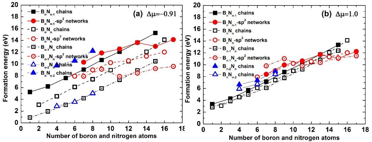
**Fig. S13** Formation energies of chains and most-stable sp<sup>2</sup> networks of  $B_{n-1}N_n$ ,  $B_nN_n$ ,  $B_nN_{n-1}$ ,  $B_{n-2}N_n$  and  $B_nN_{n-2}$  on a Cu(111) surface versus the number of atoms in h-BN clusters with chemical potential differences  $\Delta\mu$ = (a) -0.91, and (b) 1.0. Blue triangles present that considering  $B_n N_m$  chains with more N-N or B-B bonds is not helpful to understand growth of h-BN clusters on a Cu(111) surface.
