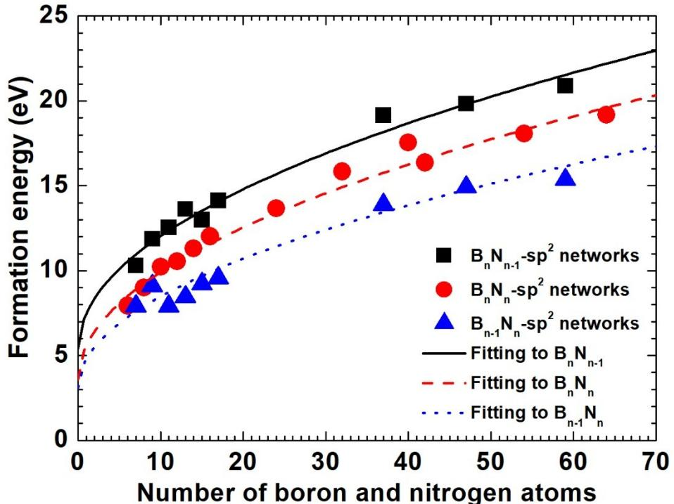
**Fig. S14** Formation energies of lowest-energy sp<sup>2</sup> networks of  $B_n N_m$  ( $m=n-1$ ,  $n$ ,  $n+1$ ) on a Cu (111) surface versus the number of atoms in h-BN clusters. Fitting curves are obtained by Eq. (5). The values of fitting parameters are presented in Table 1. The fitting curves for sp<sup>2</sup>-networks clusters in Fig. 3, 6 and 9 are the same as the corresponding one in this figure, respectively.
