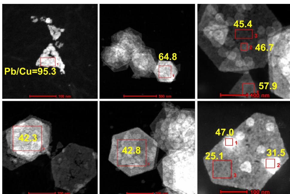
**Figure S17.** Results of EDX characterization of individual NPLs as well as NPL ensembles revealing a random distribution of residual copper atoms all over the NPLs (the Pb:Cu ratio is shown in each image with a corresponding area on which the analysis was performed).
