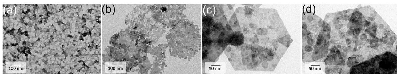
**Figure S13.** TEM images of PbS NPLs and nanosheets after ligand exchange with NH<sub>4</sub>I in MFA (a) and in DMF (b), with PbI<sub>2</sub> in DMF (c), and with LiI in DMF (d).
