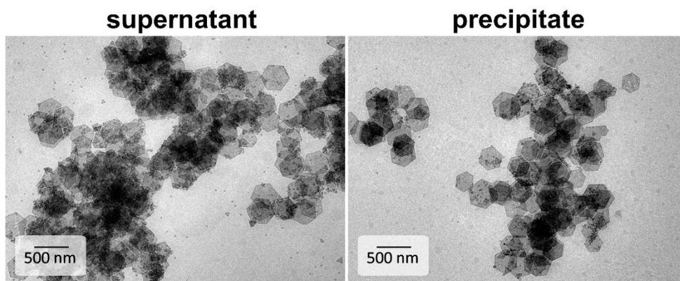
**Figure S16.** TEM images of A) precipitate and B) supernatant of LiI-capped PbS NCs after centrifugation.
