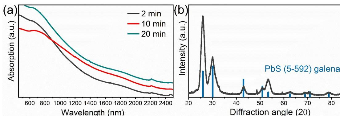
**Figure S12.** Absorption spectra of the products of Cu<sup>+</sup>-to-Pb<sup>2+</sup> CE reaction sampled after 2, 10 and 20 minutes (a) along with XRD pattern of the 2 min sample (b).
