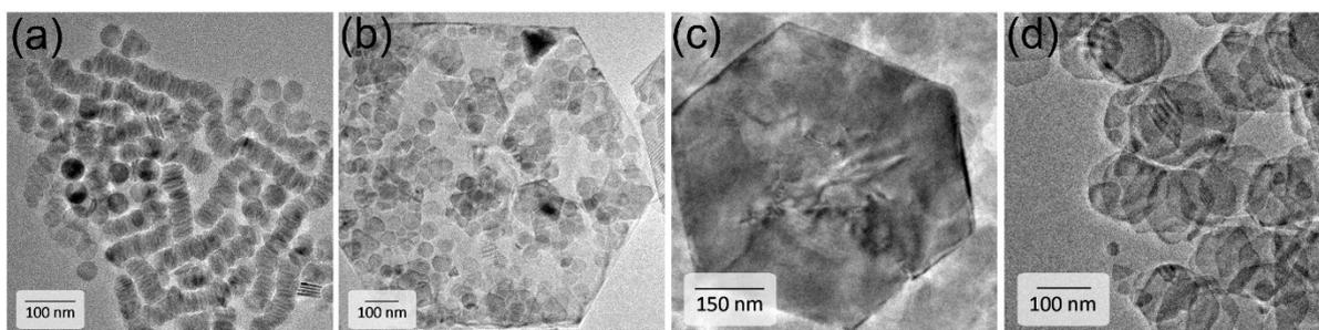
**Figure S11.** TEM images of CuS NPLs and larger nanosheets obtained with a Cu:S mol. ratio of 1:8 (a, b) and 1:16 (c, d).
