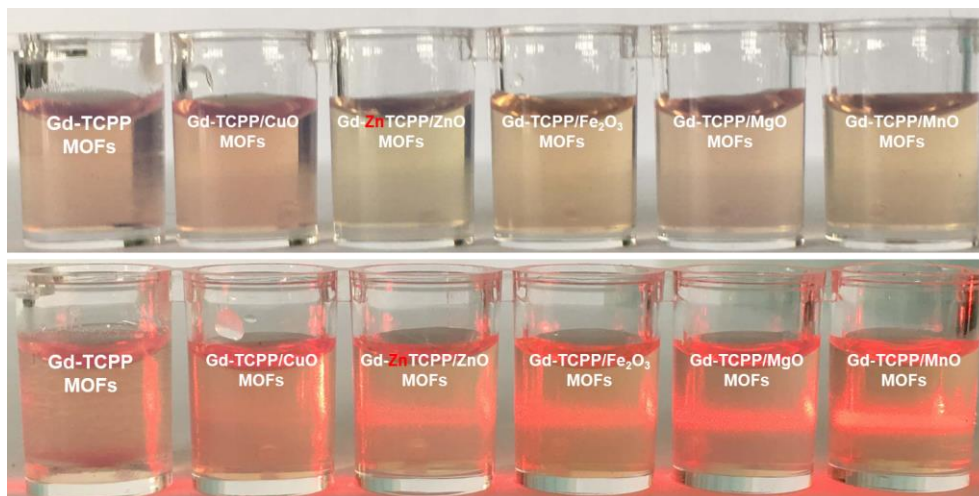
Figure S10. Tyndall effect has been observed for the Gd-TCPP, Gd-TCPP/CuO, Gd-ZnTCPP/ZnO, Gd-TCPP/Fe 2 O 3 , Gd-TCPP/MgO, and Gd-TCPP/MnO nanohybrids.
