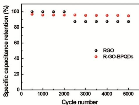
Fig. S5 Specific capacitance retention of supercapacitors based on RGO and R-GO-BPQDs after 5000 cycles (current density: 0.1 mA/ cm<sup>2</sup>).
