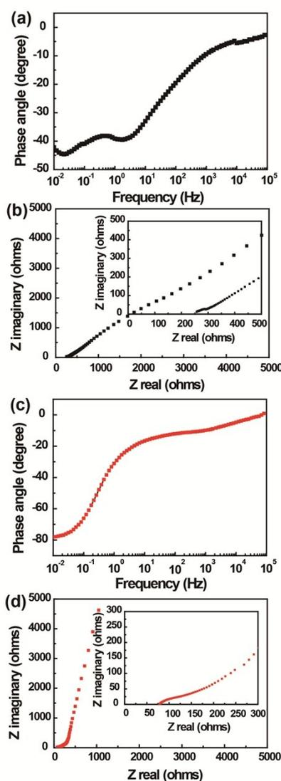
Fig. S4 Bode plots and Nyquist impedance plots of RGO (a, b) and R-GO-BPQDs (c, d) at frequency from 0.01 to 5000 Hz. The corresponding  $R_s$  values are 258 and 78  $\Omega$ , respectively.
