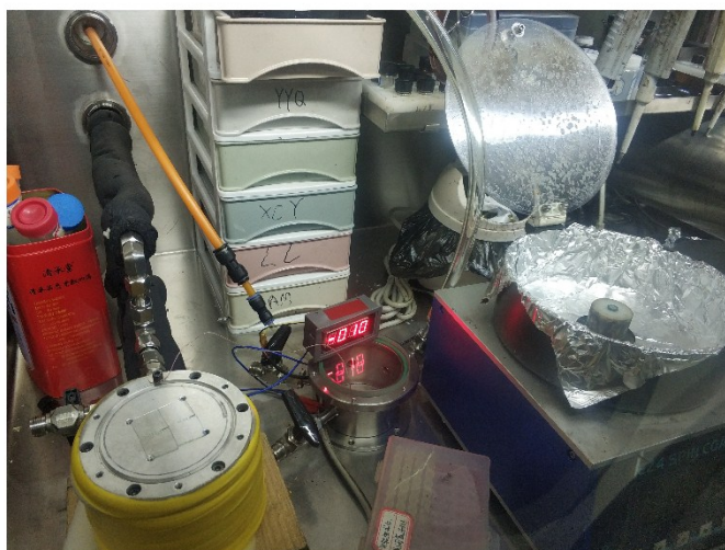
Figure S1. The design and the photo of the home-made cooling system for NPCG method. The cooling plate is placed near the spin coater in the same glove box.
