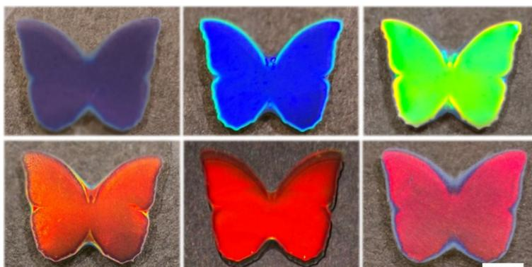
**Figure S3.** Optical images of the rGO hybrid non-close-packed CCAs films with different structural color. Scale bar was 1 cm.
