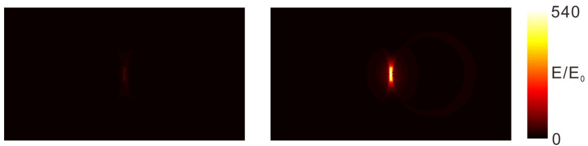
Figure S3. Comparison of the electric-field enhancement distributions of dimer (38/26/1) at the (left) dipolar (532 nm) and (right) coupling (637 nm) modes.
