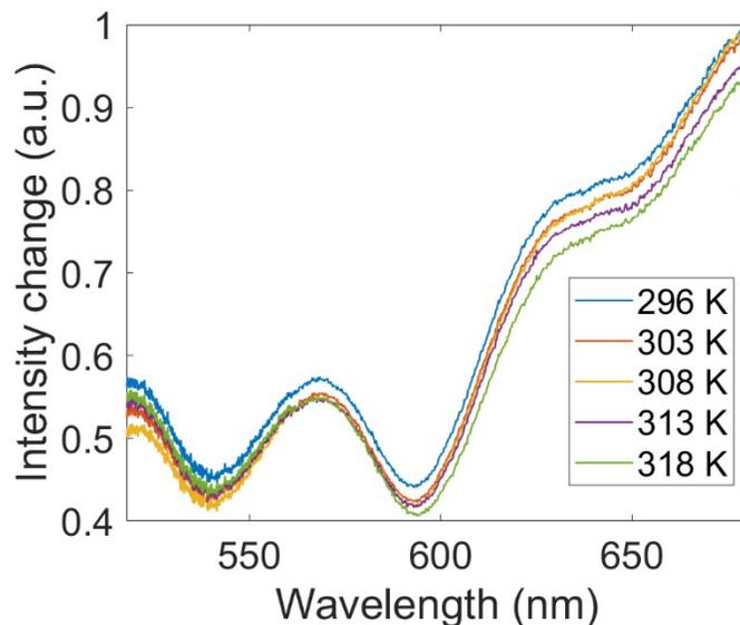
**Figure S5:** The spectrum of the MOF-coated sensor at different temperatures are measured. The spectra red shift as the temperature increases because the refractive index of the material (mainly from Au and Si) increases as temperature increases from 296 K to 318 K. The information is used to calibrate the baseline of the sensor during the measurement.
