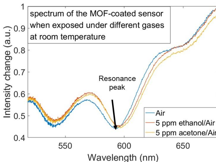
**Figure S2:** Measured spectrum of the MOF-coated sensor when exposed under dry air, 5  $\mu\text{mol/mol}$  (ppm) acetone and 5  $\mu\text{mol/mol}$  (ppm) ethanol. The intensity changes at the resonance peak are measured during the gas sensing process. Note: The spectrum is measured in a reflection-based configuration and therefore the resonance peak is inverted (occurs as a valley).
