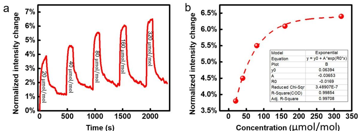
**Figure S6:** Results from a single set experiment to establish the dynamic range of the device for acetone monitoring. (a) Sensor response to acetone vapor with concentration from 20  $\mu\text{mol/mol}$  (ppm) to 320  $\mu\text{mol/mol}$ . This experiment was run to determine the upper limit of the NHA sensor. As from the exponential curve fitting of the sensor
