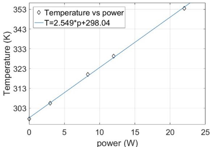
**Figure S4:** Temperature vs power consumption for the system. The system has a high-power consumption of  $2.549 \text{ W/K}$  because the whole gas cell is heated up by the cartridge heater. The power consumption can be decreased by using an integrated micro-heater. In this case, only the sensing platform ( $300 \mu\text{m} \times 300 \mu\text{m}$ ) instead of the whole gas cell would be heated.
