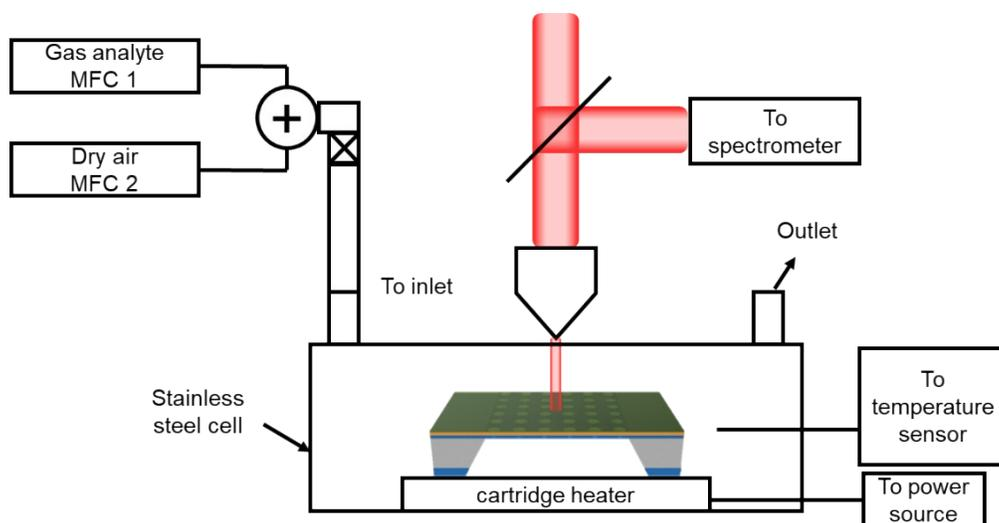
**Figure S1:** Schematic view of the system setup. A broadband visible light source (400 nm - 700 nm) is focused on the sensor by a microscope and the reflected signal is captured by a spectrometer. A cartridge heater is inserted in the gas cell to vary the operating temperature. Target gases (e.g. acetone and ethanol) from cylinders are mixed with dry air to generate different concentrations. The flow rate is controlled at 2 slm as set on mass-flow controllers.
