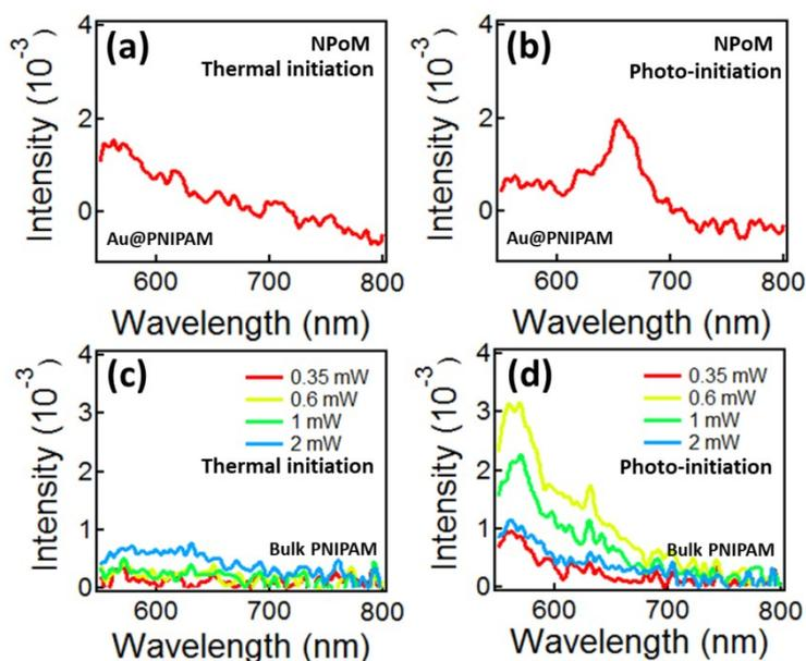
Fig. S5 PL spectra of (a, b) Au@PNIPAM NPoMs and (c, d) PNIPAM beads with (a, c) thermally initialized PNIPAM coatings ( $K_2S_4O_8$  as the initiator) and (b, d) photo-initialized PNIPAM coatings (2-hydroxy-2-methylpropio-phenone as the photo-initiator). Clearly, the PL signals mainly come from the incorporated segment of photo-initiators but neither from the PNIPAM chains, nor from the plasmon gap emission.
