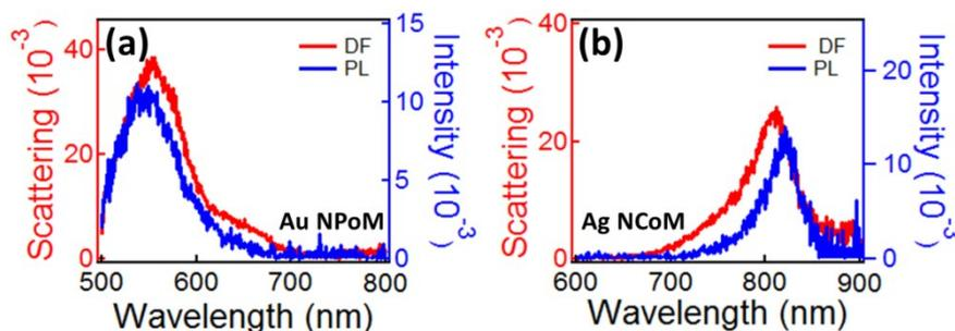
Fig. S3. DF and PL spectra of (a) 100 nm Au NPoM and (b) 100 nm Ag nanocube on mirror (NCoM).
