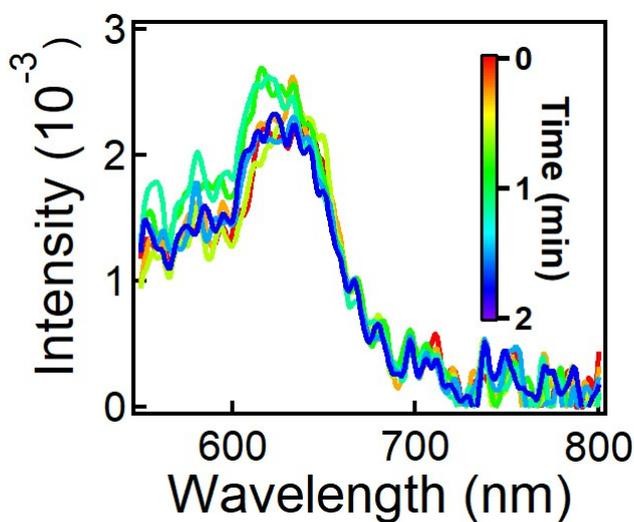
Fig. S6 Time-dependent PL spectra of Au@PNIPAM NPoM system under the irradiation of 532 nm laser (0.35 mW).
