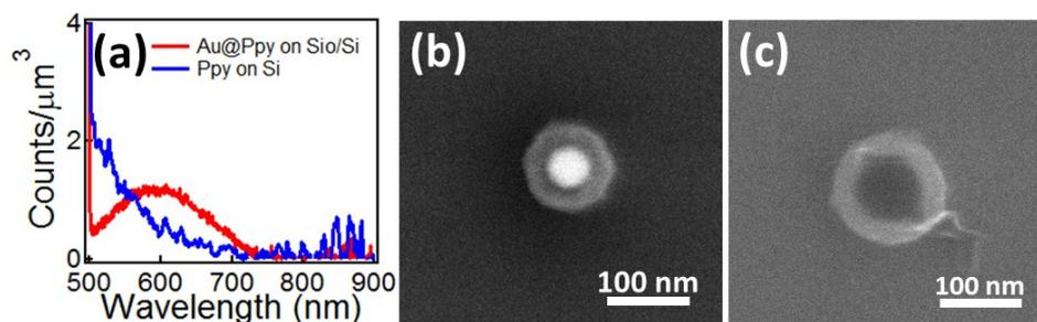
Fig. S4. (a) PL spectra of Au@Ppy NP and Ppy bead on Si substrate and (b, c) their corresponding SEM images. (b) Au@Ppy NP, (c) Ppy bead.
