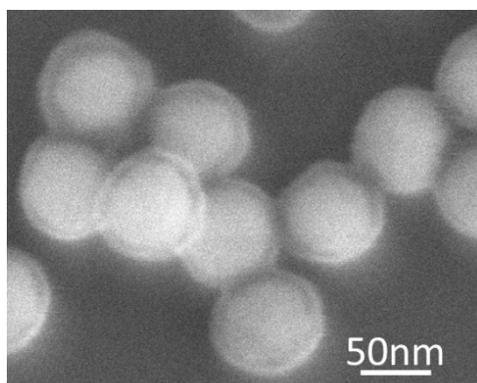
Fig. S2. SEM image of the Au@Ppy NPs (shell thickness: ~7 nm).
