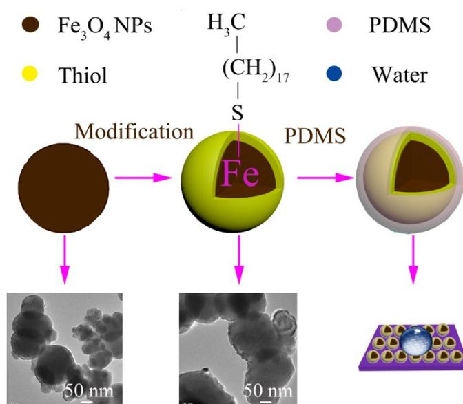
**Figure S1.** Surface modification of Fe<sub>3</sub>O<sub>4</sub> NPs.
