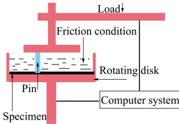
**Figure S7.** The schematic diagram of the friction testing device.
