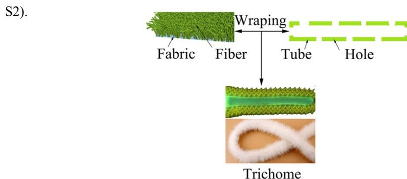
**Figure S2.** Fabrication process of the bioinspired fiber trichome.
