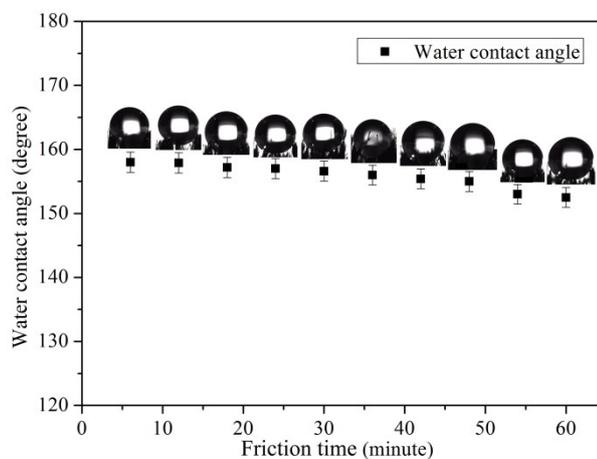
**Figure S10.** The value of water contact angle of the fabric worn surface as a function of friction time.
