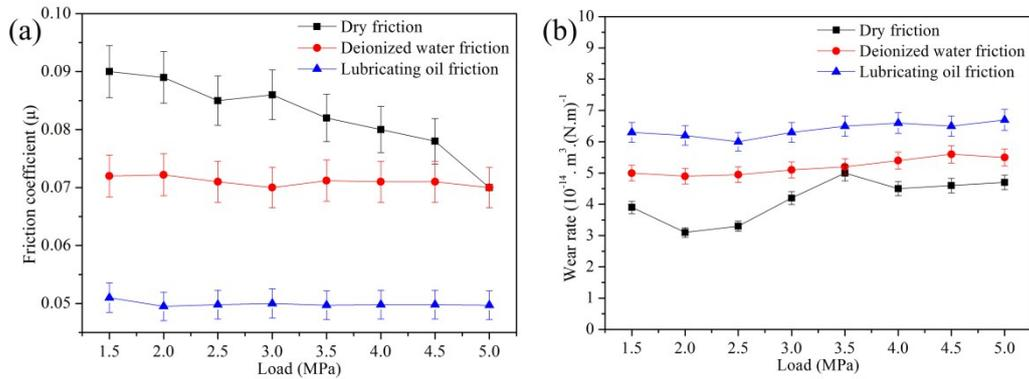
**Figure S8.** The value of friction coefficient (a) and wear rate (b) of the fabric sample at the different applied load.
