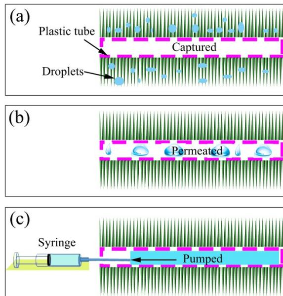
**Figure S5.** The schematic diagram of the continuous water transport of the caterpillar-inspired
