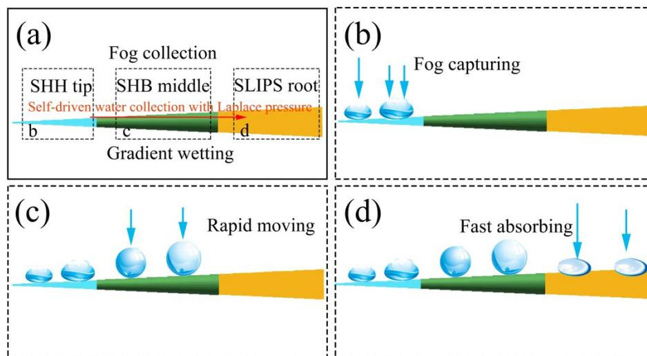
**Figure S6.** The structure of the caterpillar-inspired fiber trichome with gradient wetting.
