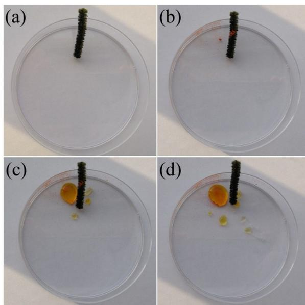
**Figure S11.** The self-cleaning characteristics of the earthworm-inspired fiber trichome.
