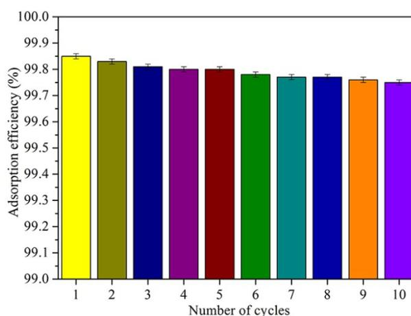
**Figure S3.** Oil adsorption performance of the caterpillar-inspired fiber trichome as a function of cycles by using n-hexane/water mixture.
