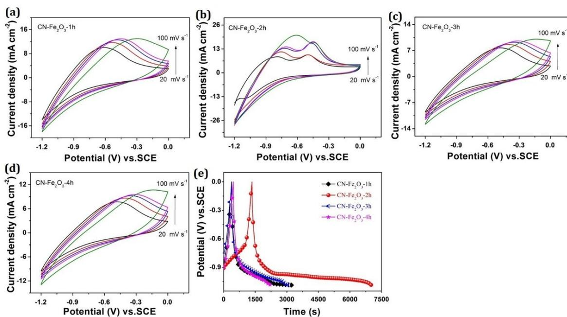
**Fig. S4.** a-d) CV curves of CN-Fe<sub>2</sub>O<sub>3</sub>-xh. e) GCD curves of CN-Fe<sub>2</sub>O<sub>3</sub>-xh at the current density of 0.5 mA cm<sup>-2</sup>.
