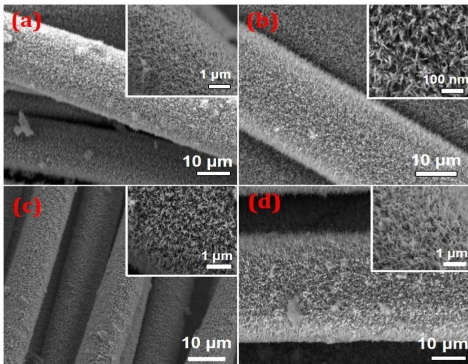
**Fig. S3.** SEM images for CN-Fe<sub>2</sub>O<sub>3</sub> at different reduction time. a) 1 h, b) 2 h, c) 3 h and d) 4 h.
