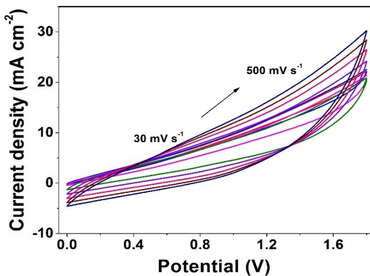
Fig. S10. CV curves of CN-Fe<sub>2</sub>O<sub>3</sub>-2h//MnO<sub>2</sub> ASC device.
