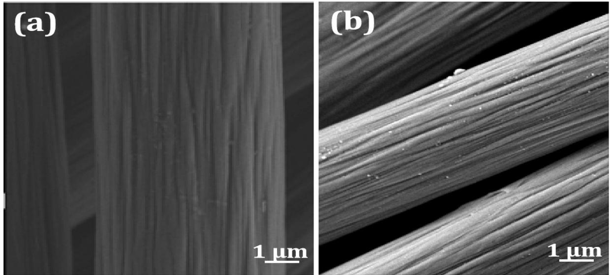
Fig. S1. SEM patterns of (a) pristine CC and PDA coated CC.
