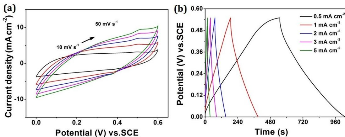
Fig. S9. a) CV curves of MnO<sub>2</sub>. b) GCD curves of MnO<sub>2</sub> at different current density from 0.5 mA cm<sup>-2</sup> to 5 mA cm<sup>-2</sup>.
