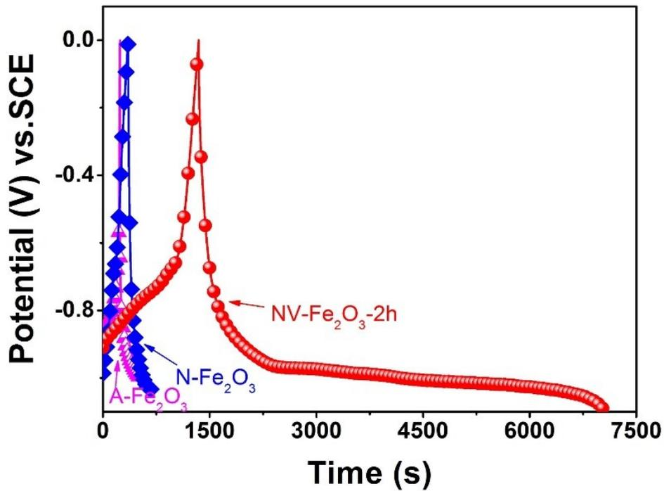
Fig. S6. GCD curves of A-Fe<sub>2</sub>O<sub>3</sub>, N-Fe<sub>2</sub>O<sub>3</sub> and CN-Fe<sub>2</sub>O<sub>3</sub>-2h at a current density of 0.5 mA cm<sup>-2</sup>.
