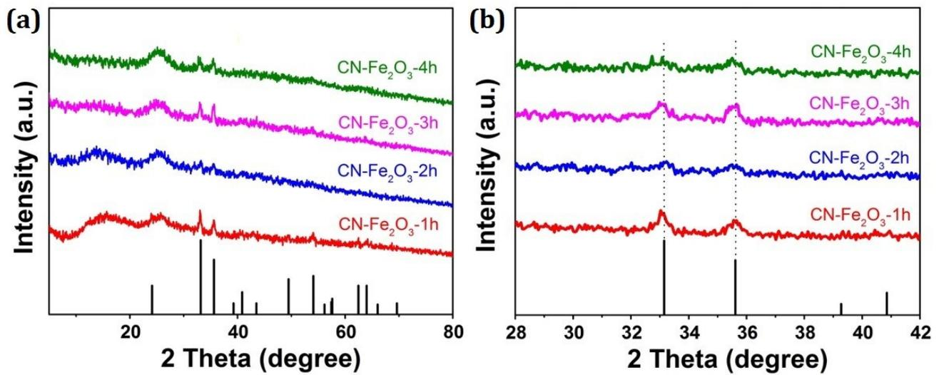
Fig. S2. XRD patterns for CN-Fe<sub>2</sub>O<sub>3</sub>-1h, CN-Fe<sub>2</sub>O<sub>3</sub>-2h, CN-Fe<sub>2</sub>O<sub>3</sub>-3h and CN-Fe<sub>2</sub>O<sub>3</sub>-4h.
