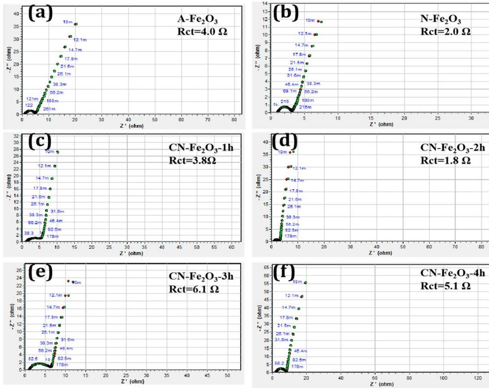
Fig. S5. The fitted Nyquist plots of a) A-Fe<sub>2</sub>O<sub>3</sub>; b) N-Fe<sub>2</sub>O<sub>3</sub>; c-d) CN-Fe<sub>2</sub>O<sub>3</sub>-xh
