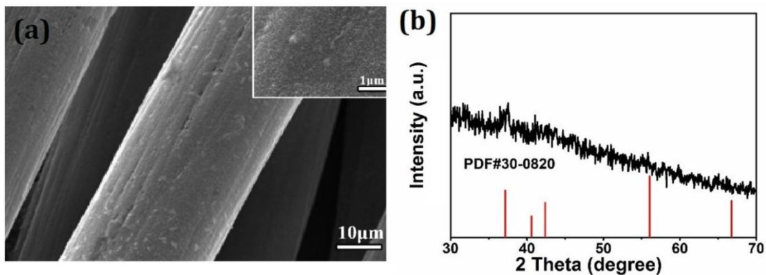
Fig. S8. a) SEM images of MnO<sub>2</sub> on CC fibers. b) XRD patterns of pristine MnO<sub>2</sub>.
