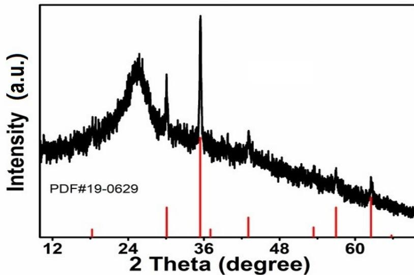
**Fig. S7.** XRD patterns of CN-Fe<sub>2</sub>O<sub>3</sub>-2h after long-term cycles.
