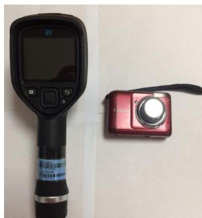
Fig. S23 Picture of the thermal imaging (left) and modified digital (right) cameras.
