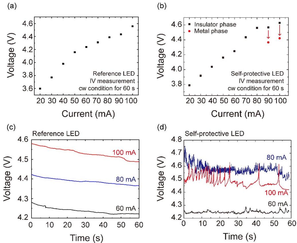
**Fig. S3** Voltage-current plots in *cw* current condition for (a) reference LED and (b) self-protective LED and voltage-time measurement for *cw* current conditions of 60, 80, and 100 mA for (c) reference LED and (d) self-protective LED.
