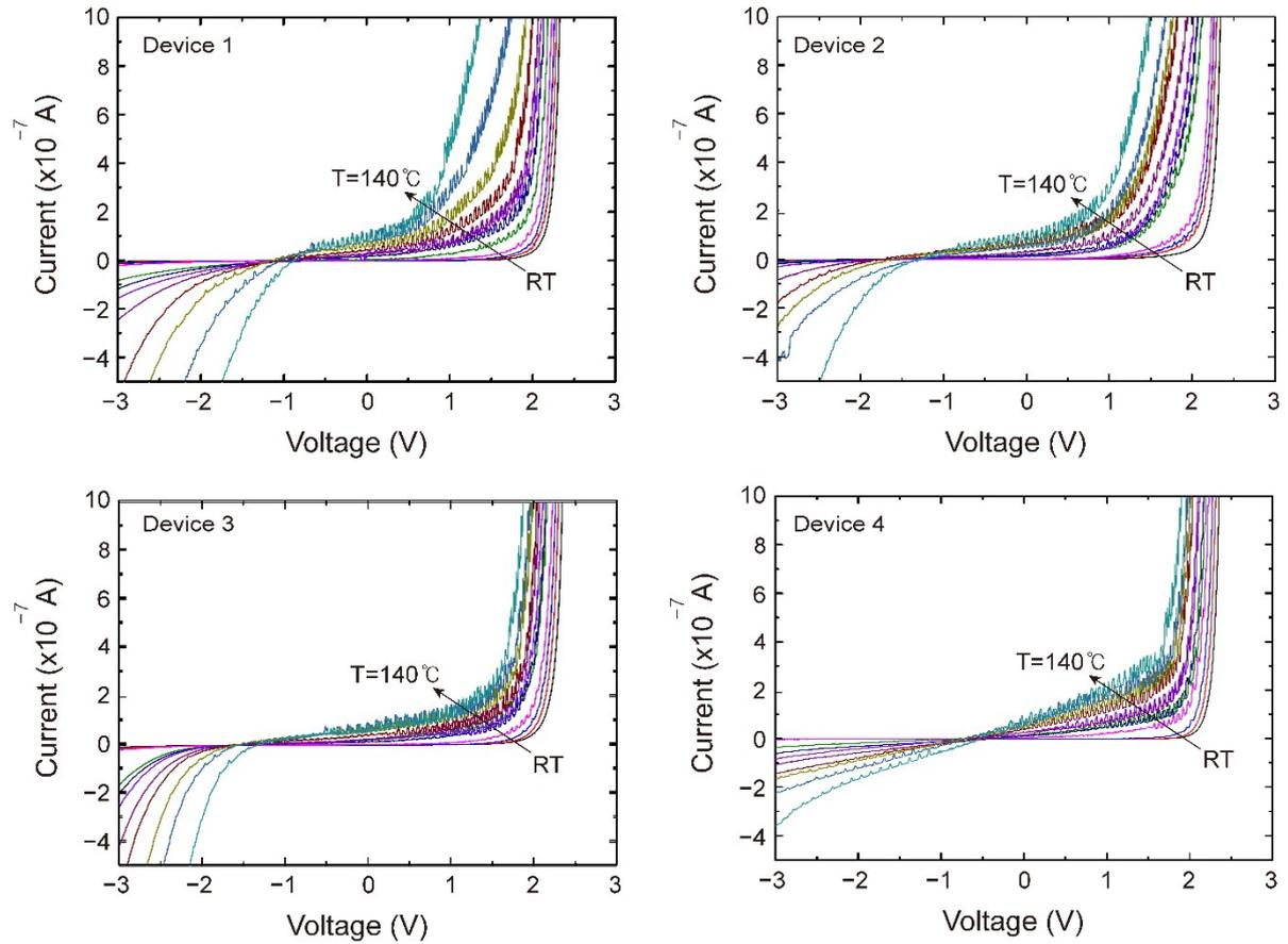
**Fig. S2** Temperature-dependent I-V measurement results for various self-protective LED samples.
