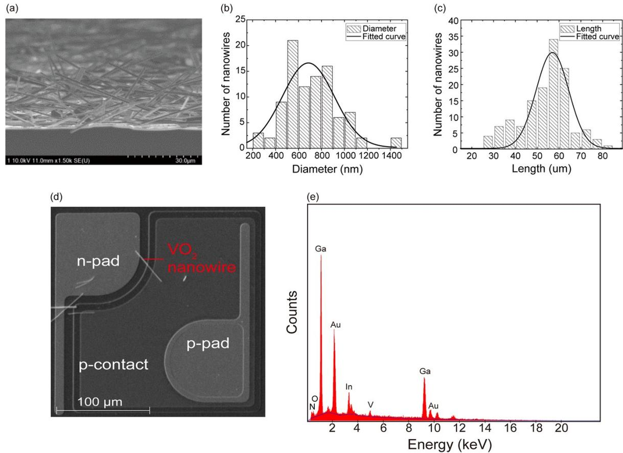
**Fig. S1** (a) SEM image for VO<sub>2</sub> nanowires after vapor transport growth. Histograms and corresponding Gaussian fits showing the distribution in (b) the diameter and (c) the length of VO<sub>2</sub> nanowires. (d) top-view SEM image and (e) EDX data for self-protective LED.
